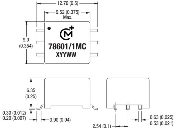
Unless otherwise stated all dimensions in mm (inches) ±0.25 (0.01). All pins on a 2.54 (0.1) pitch and within ±0.25 (0.01) of true position. Package Weight: 1.1g Typ.
