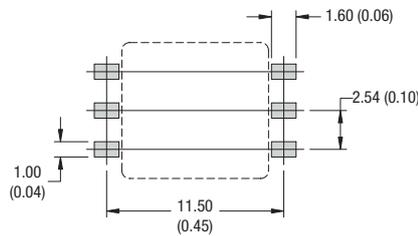
Unless otherwise stated all dimensions in mm (inches) ±0.25 (0.01). All pins on a 2.54 (0.1) pitch and within ±0.25 (0.01) of true position.
