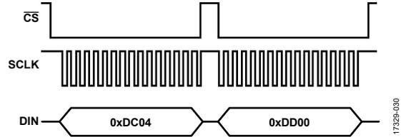
Figure 47. SPI Sequence for Writing 0x0004 to FILT\_CTRL
