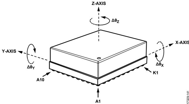
Figure 53. Delta Angle Axis and Polarity Assignments
