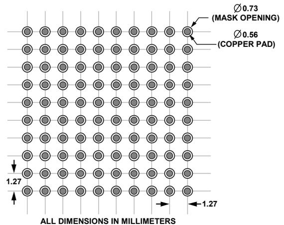
Figure 63. Recommend PCB Pattern, Solder Mask Defined Pads
