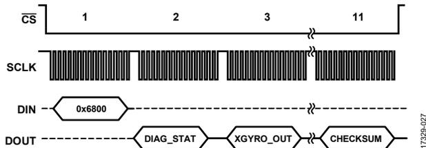
Figure 43. Burst Read Sequence with BURST\_SEL = 0
