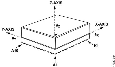
Figure 51. Accelerometer Axis and Polarity Assignments
