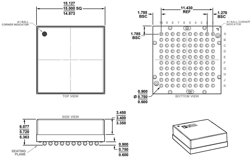
Figure 67. 100-Ball Ball Grid Array Module [BGA]
