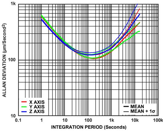
Figure 23. Accelerometer Allan Deviation,  $T_c = 25^\circ\text{C}$
