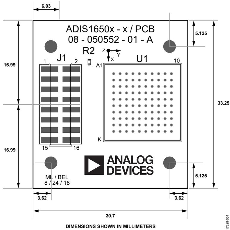
Figure 65. Top View of the ADIS16507 Breakout Board
