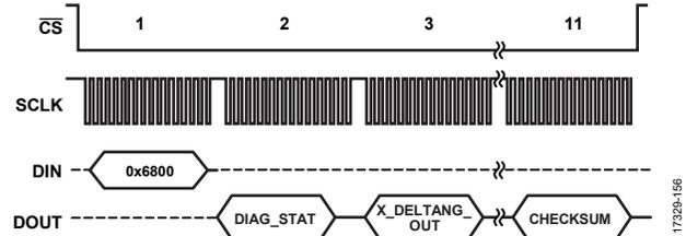
Figure 44. Burst Read Sequence with BURST\_SEL = 1
