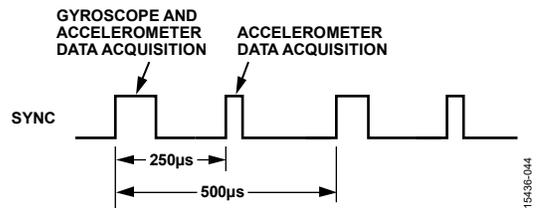
Figure 30. Sync Output Signal, Register MSC\_CTRL, Bits[3:2] = 11
