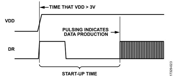
Figure 37. Data Ready Response During Startup
