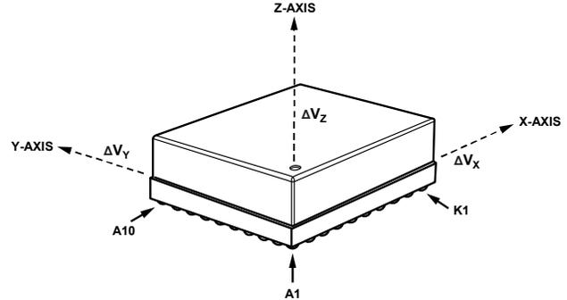
Figure 55. Delta Velocity Axis and Polarity Assignments
