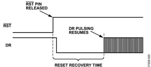
Figure 39. Data Ready Response During Reset ( $\overline{RST} = 0$ ) Recovery
