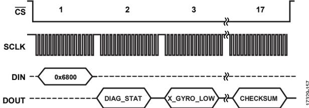
Figure 45. Burst Read Sequence with BURST\_SEL = 0
