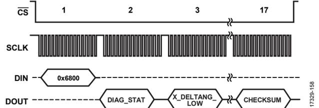
Figure 46. Burst Read Sequence with BURST\_SEL = 1
