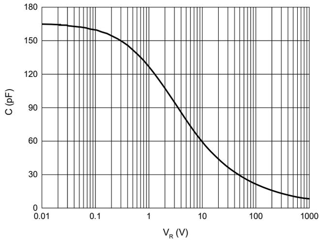
Fig. 4 - Capacitive Charge vs Reverse Voltage
