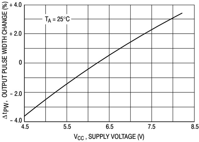
Figure 5.  $f_{out}$ , Pulse Width Change versus Supply Voltage
