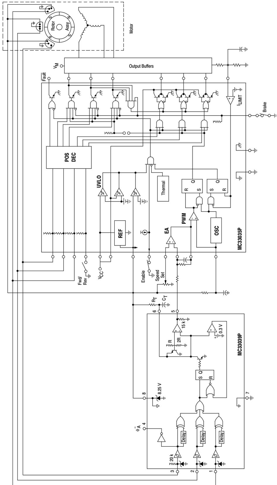
Figure 2. Typical Closed Loop Speed Control Application
