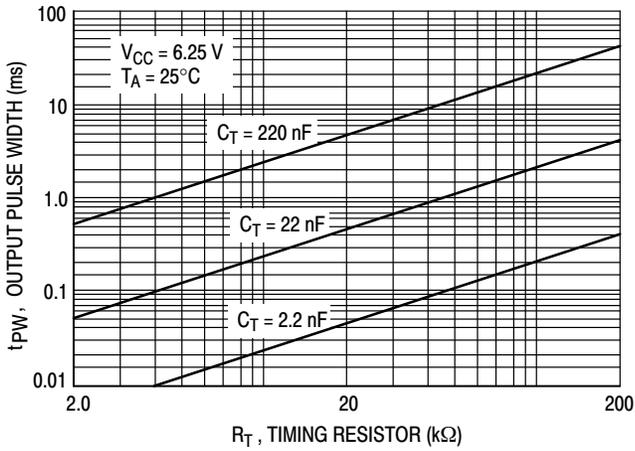
Figure 3.  $f_{out}$ , Pulse Width versus Timing Resistor
