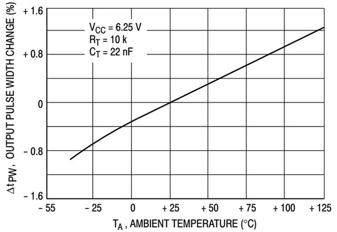
Figure 4.  $f_{out}$ , Pulse Width Change versus Temperature
