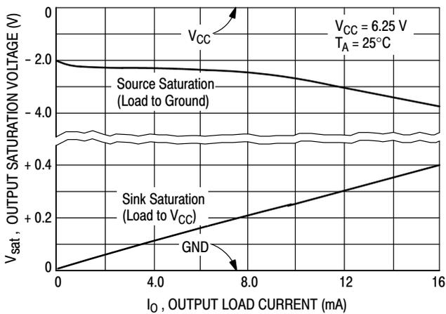
Figure 7.  $f_{out}$ , Saturation versus Load Current
