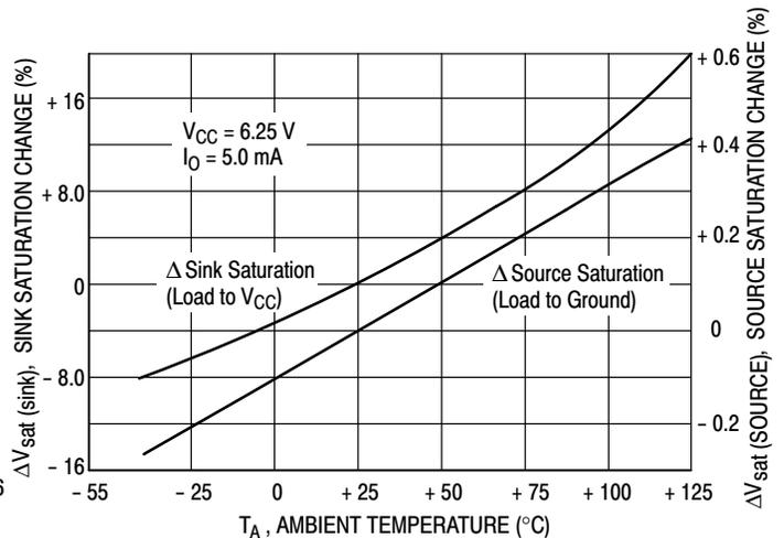
Figure 8.  $f_{out}$ , Saturation Change versus Temperature
