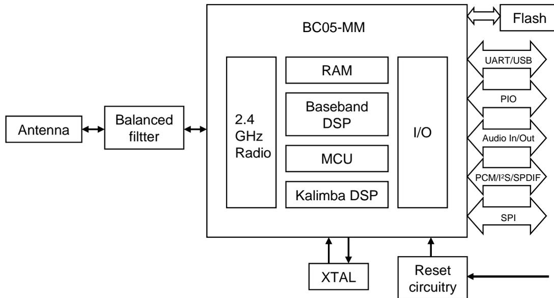
**Figure 1:** Block diagram of WT32
