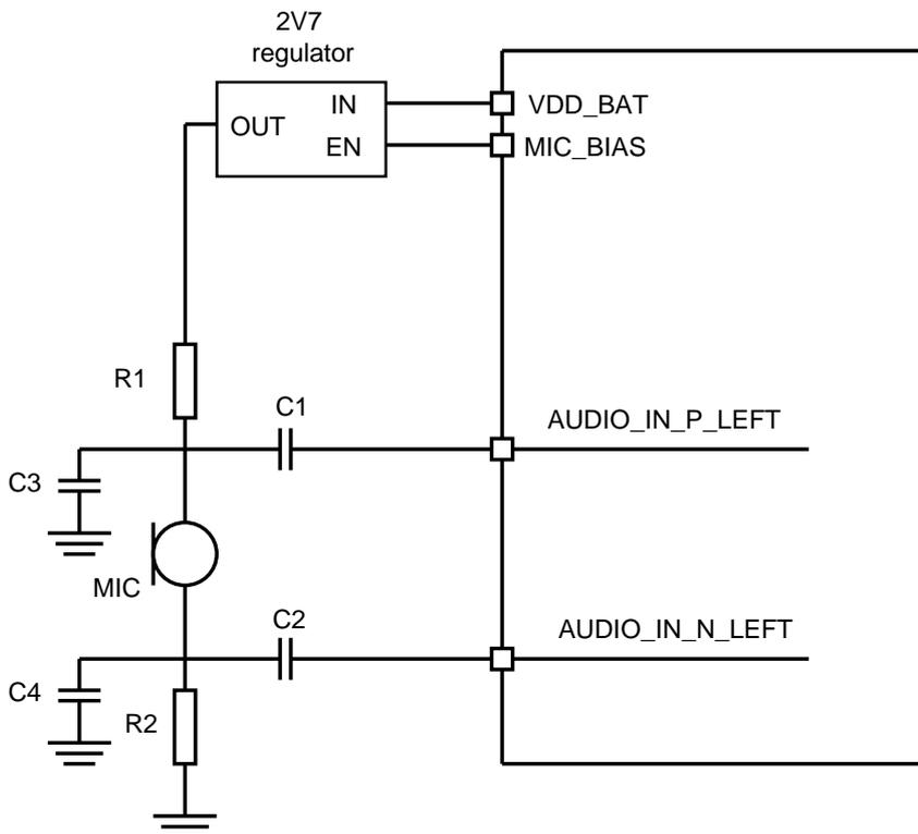
**Figure 17:** Recommended microphone biasing (left channel shown)
