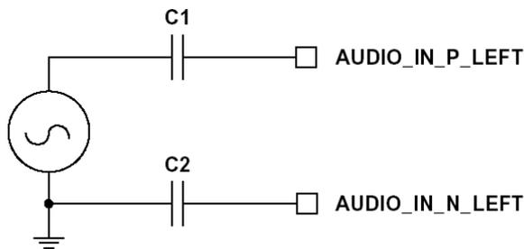
**Figure 19:** Single ended input (left channel shown)
