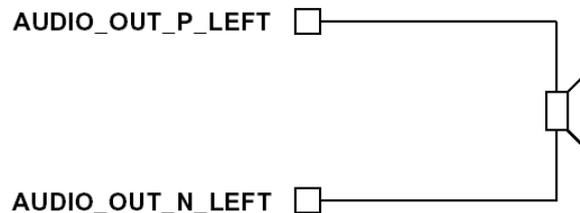
**Figure 20:** Speaker output (left channel shown)
