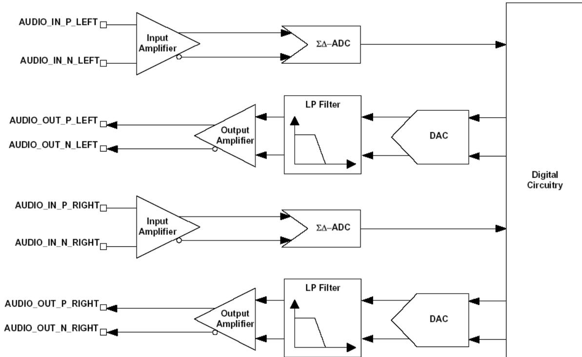
**Figure 13:** Stereo CODEC audio input and output stages
