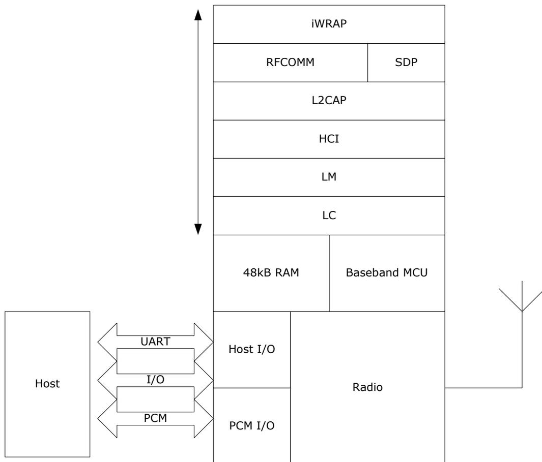
**Figure 34: iWRAP Stack**
