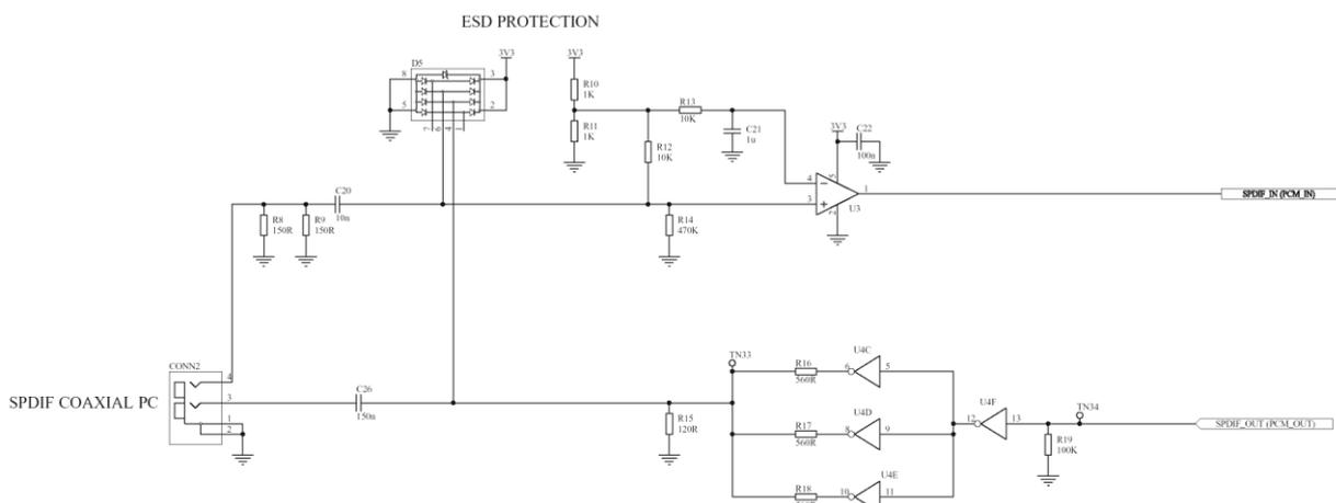
**Figure 15:** Example circuit for SPDIF interface (Co-Axial)
