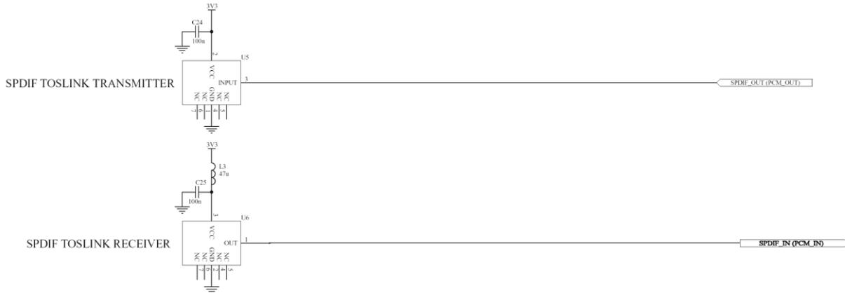
**Figure 16:** Example circuit for SPDIF interface (Optical)
