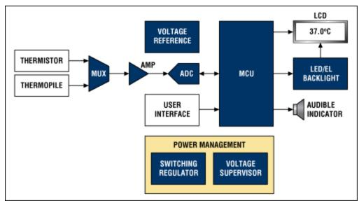
Functional block diagram of a digital thermometer. For a list of Maxim's recommended solutions for digital thermometer designs, please go to: www.maximintegrated.com/thermometer.
