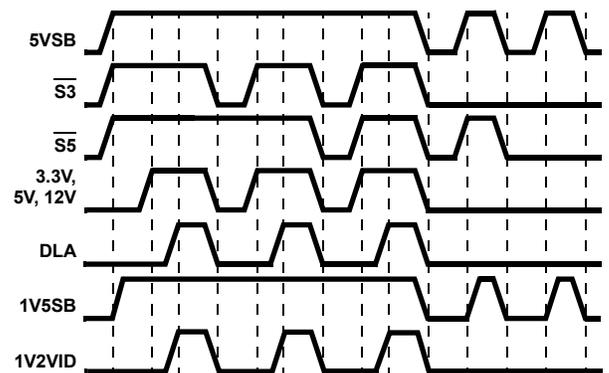
FIGURE 6. 1.5V<sub>SB</sub> AND 1.2V<sub>VID</sub> TIMING DIAGRAM
