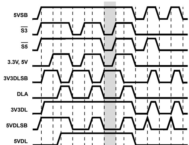
FIGURE 5. 5V<sub>DUAL</sub> AND 3.3V<sub>DUAL</sub>/3.3V<sub>SB</sub> TIMING DIAGRAM; ISL6504A
