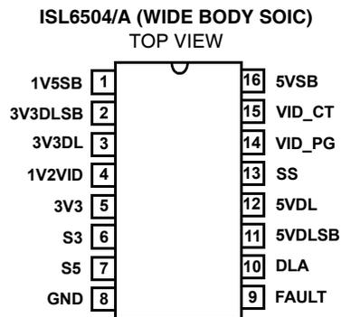
NOTE: SOIC layout should accommodate both wide and narrow footprints.
