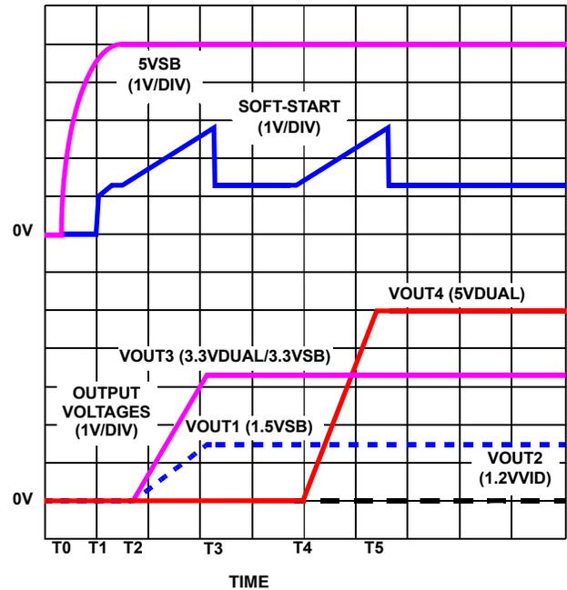
FIGURE 8. SOFT-START INTERVAL IN A SLEEP STATE; ISL6504A
