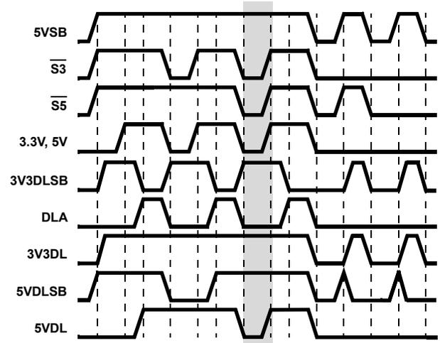
FIGURE 4. 5V<sub>DUAL</sub> AND 3.3V<sub>DUAL</sub>/3.3V<sub>SB</sub> TIMING DIAGRAM; ISL6504
