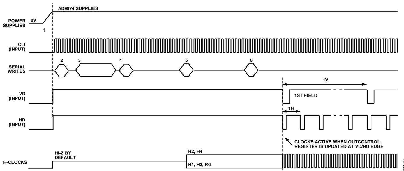
Figure 48. Recommended Power-Up Sequence
