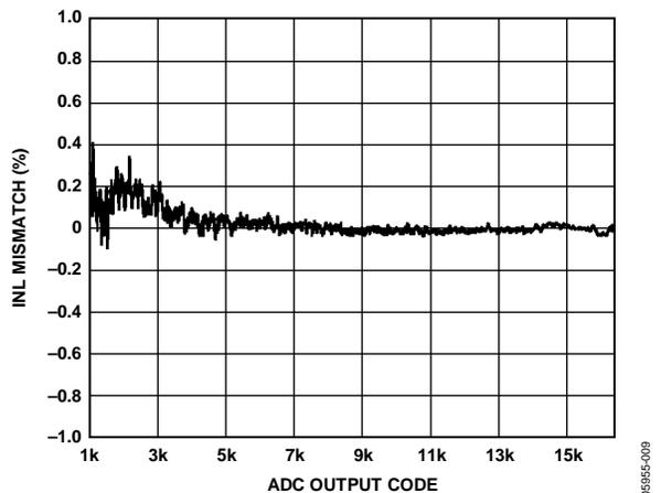
Figure 8. Linearity Mismatch vs. ADC Output Code
