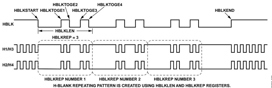
Figure 28. HBLK Repeating Pattern Using HBLKMODE = 1
