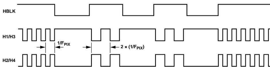
H-CLOCK FREQUENCY CAN BE REDUCED DURING HBLK BY 1/2 (AS SHOWN), 1/4, 1/6, 1/8, 1/10, 1/12, AND SO ON, UP TO 1/30 USING HCLKWIDTH REGISTER.
