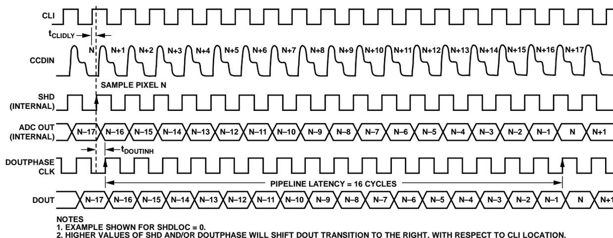
Figure 22. Pipeline Delay of AFE Data Outputs
