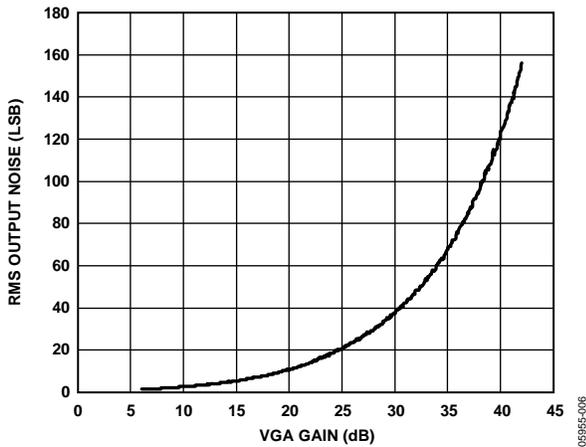
Figure 5. RMS Output Noise vs. VGA Gain
