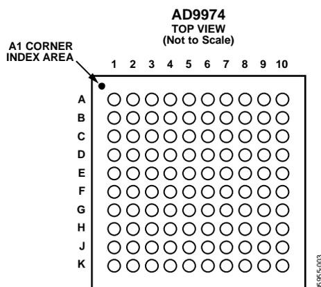
Figure 3. Pin Configuration
