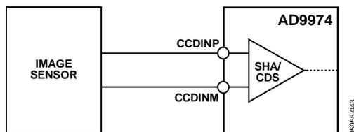
Figure 43. SHA Mode—Differential Input Configuration
