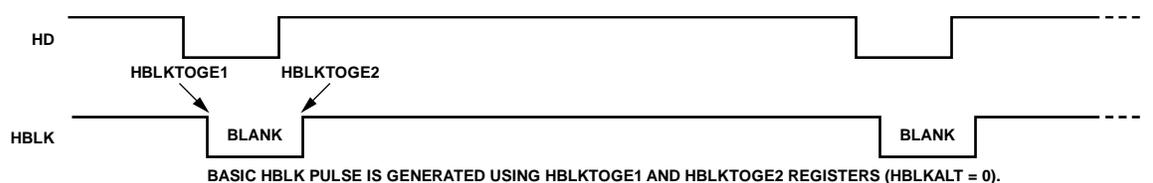
Figure 25. Typical Horizontal Blanking Pulse Placement (HBLKMODE = 0)
