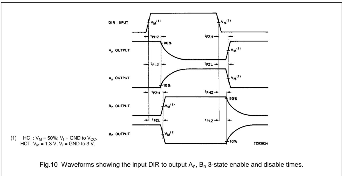
Fig.10 Waveforms showing the input DIR to output  $A_n, B_n$  3-state enable and disable times.
