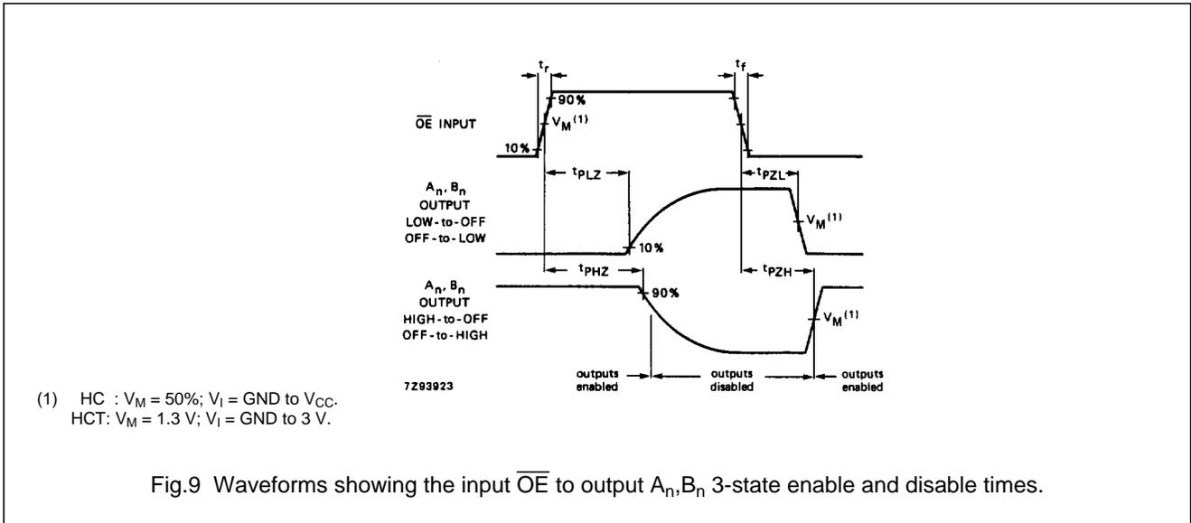
Fig.9 Waveforms showing the input  $\overline{\text{OE}}$  to output  $A_n, B_n$  3-state enable and disable times.
