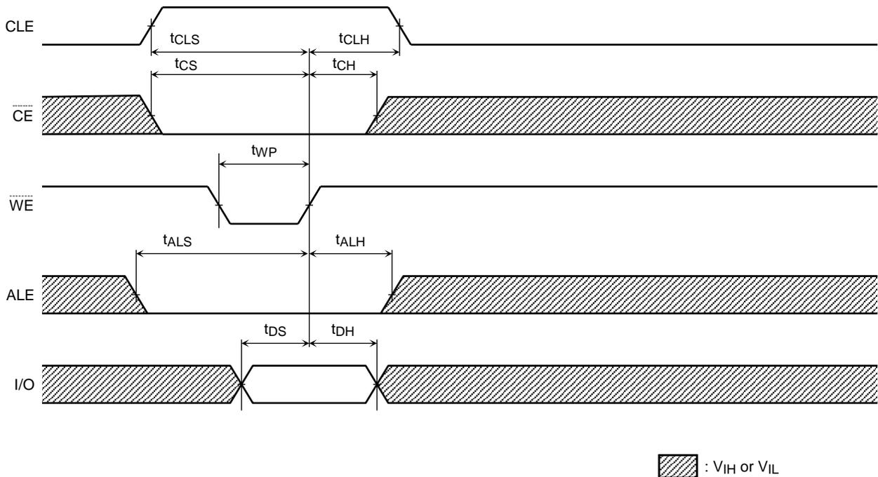
Address Input Cycle Timing Diagram
