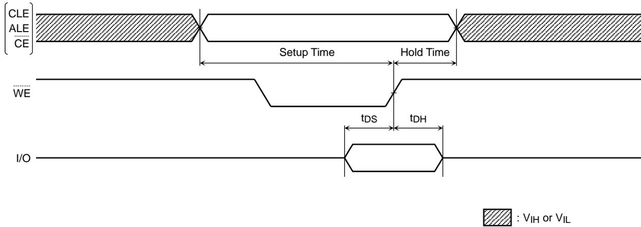
Command Input Cycle Timing Diagram
