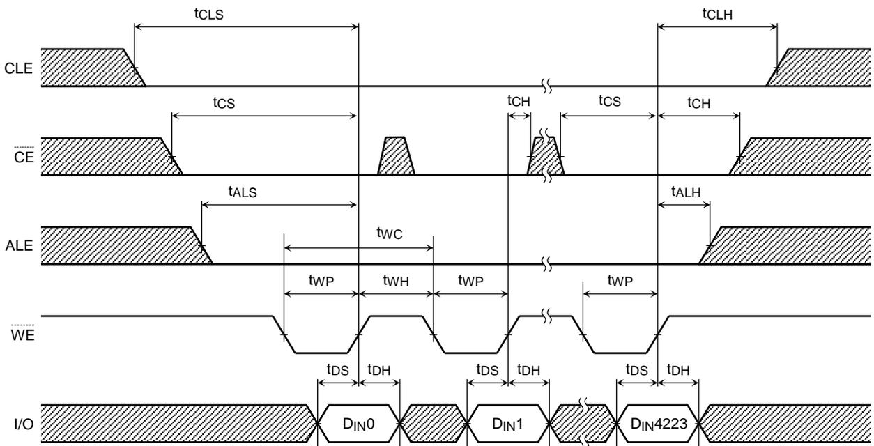
Serial Read Cycle Timing Diagram
