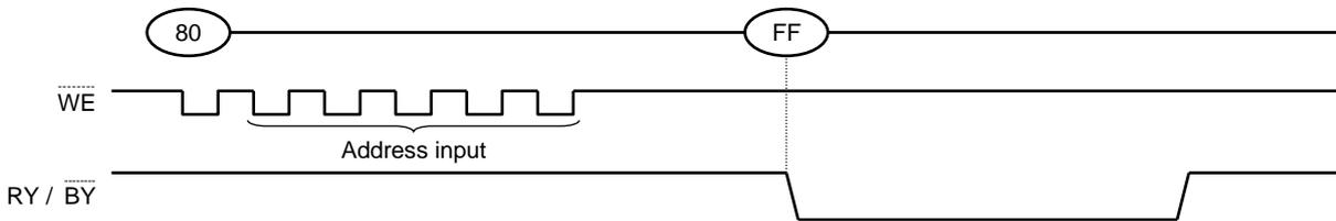
If a command other than “85h”, “10h”, “11h” or “FFh” is input, the Program operation is not performed and the device operation is set to the mode that the input command specifies.
