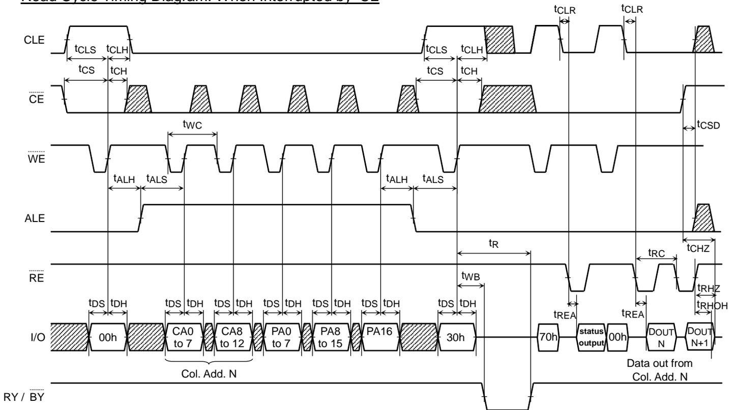
Column Address Change in Read Cycle Timing Diagram (1/2)
