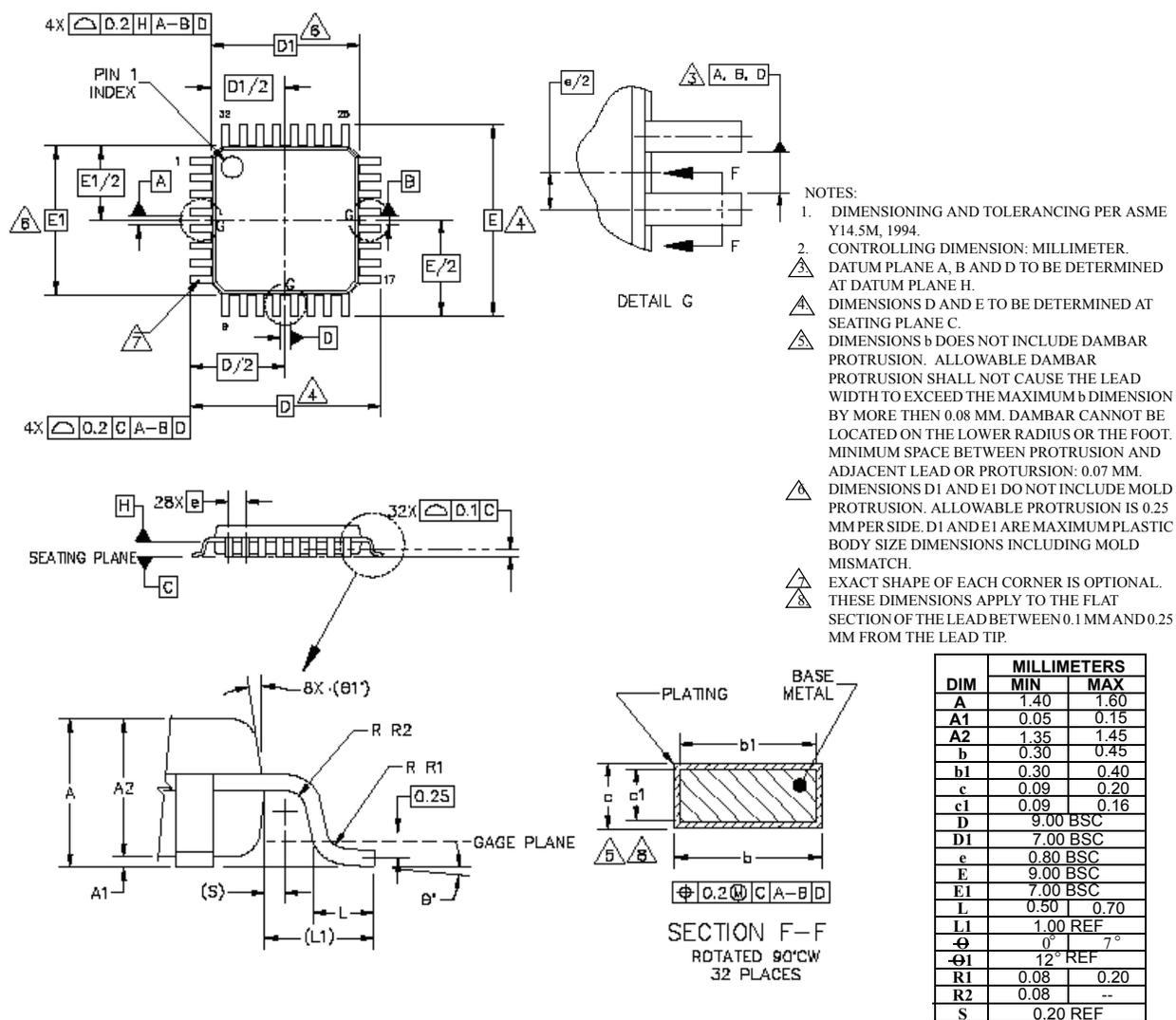
Figure 4-2 32-pin LQFP Mechanical Information (Case 873A)
