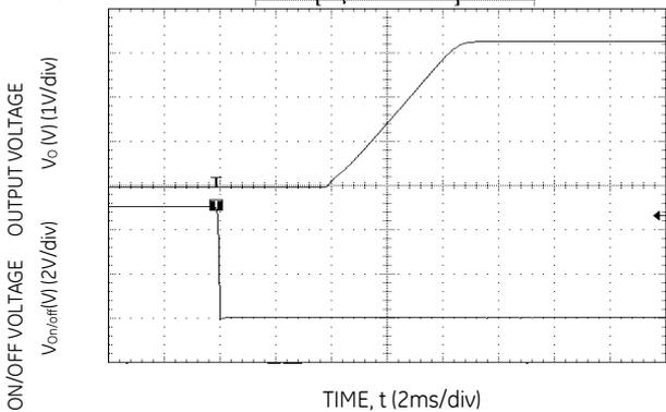
**Figure 14. Typical Start-Up Using Remote On/Off ( $V_{in} = 5.0Vdc$ ,  $V_o = 3.3Vdc$ ,  $I_o = 3A$ ).**
