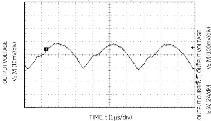
**Figure 8. Typical Output Ripple and Noise**
