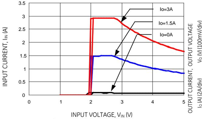
**Figure 7. Input voltage vs. Input Current**
