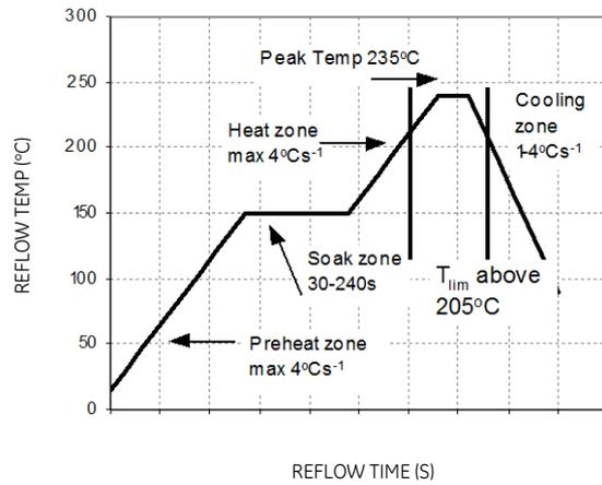
Figure 37. Reflow Profile for Tin/Lead (Sn/Pb) process.
