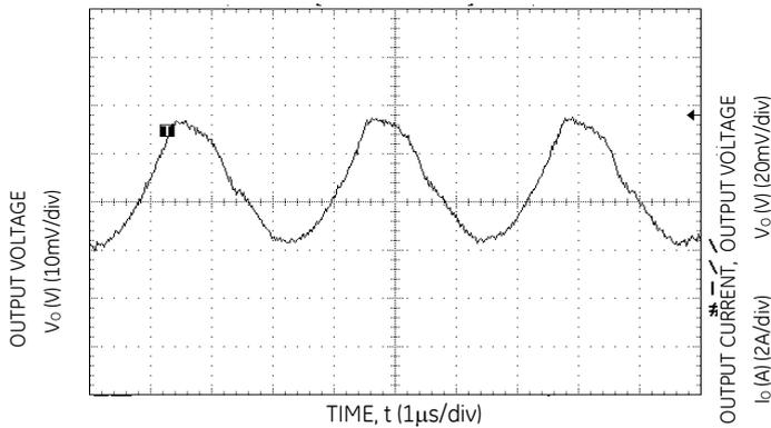
**Figure 9. Typical Output Ripple and Noise**
