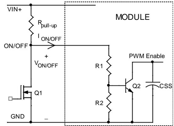
Figure 31. Circuit configuration for using negative logic On/Off.
