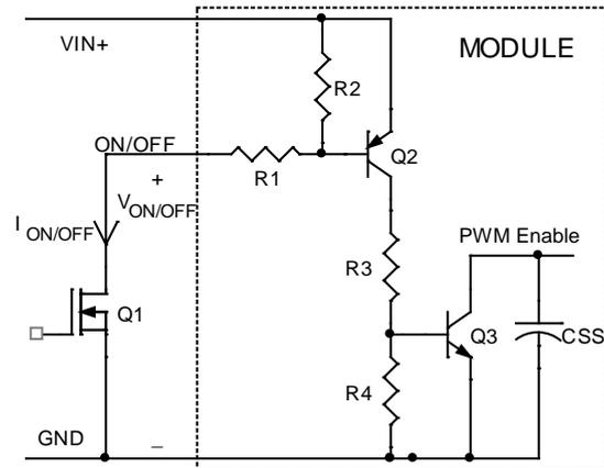
Figure 30. Circuit configuration for using positive logic On/Off.
