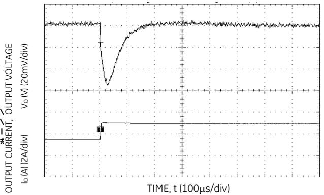
**Figure 12. Transient Response to Dynamic Load Change**
