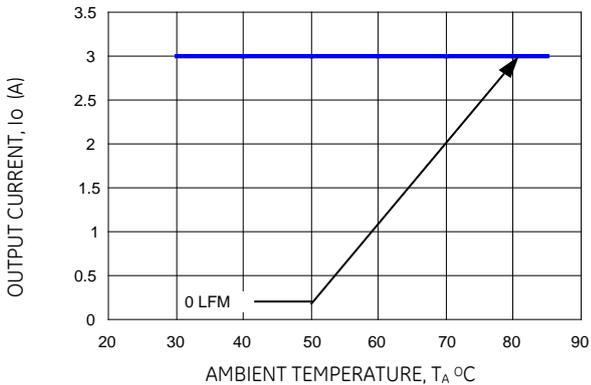
Figure 21. Derating Output Current versus Local Ambient Temperature and Airflow (VIN = 5.0Vdc, Vo=0.75 Vdc).
