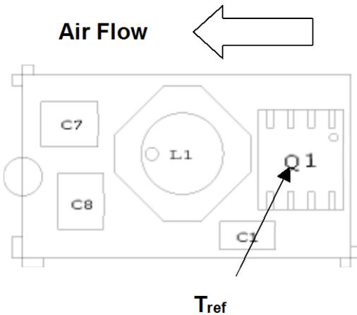
Figure 34. T<sub>ref</sub> Temperature measurement location.
