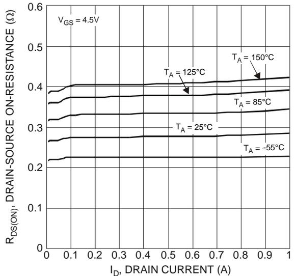
Figure 4 Typical On-Resistance vs. Drain Current and Temperature
