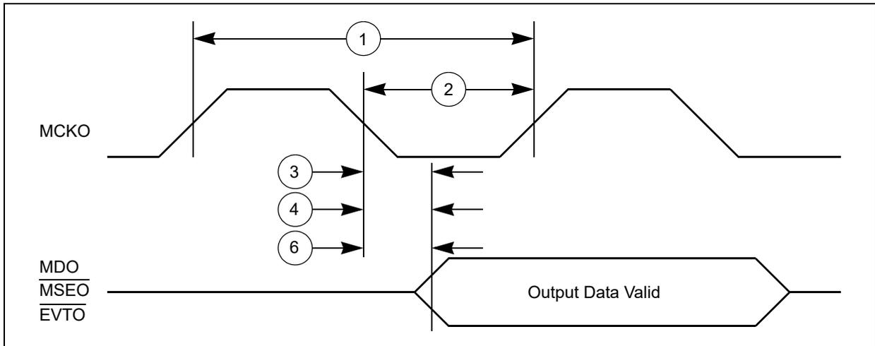
Figure 23. Nexus event trigger and test clock timings
