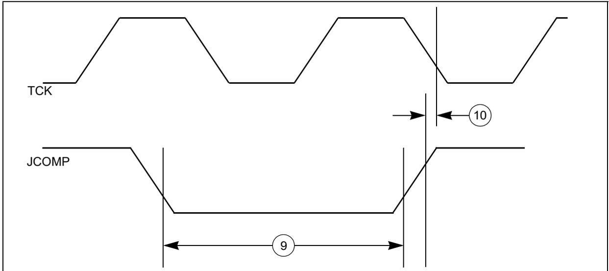
Figure 21. JTAG boundary scan timing
