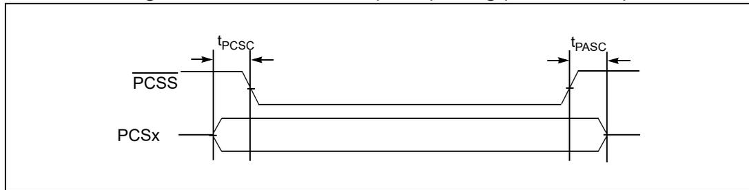
4.17.2.1.2 DSPI CMOS master mode — modified timing
