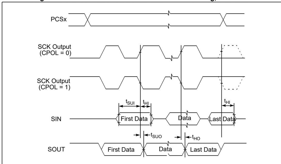
Figure 32. DSPI PCS strobe ( $\overline{\text{PCSS}}$ ) timing (master mode)
