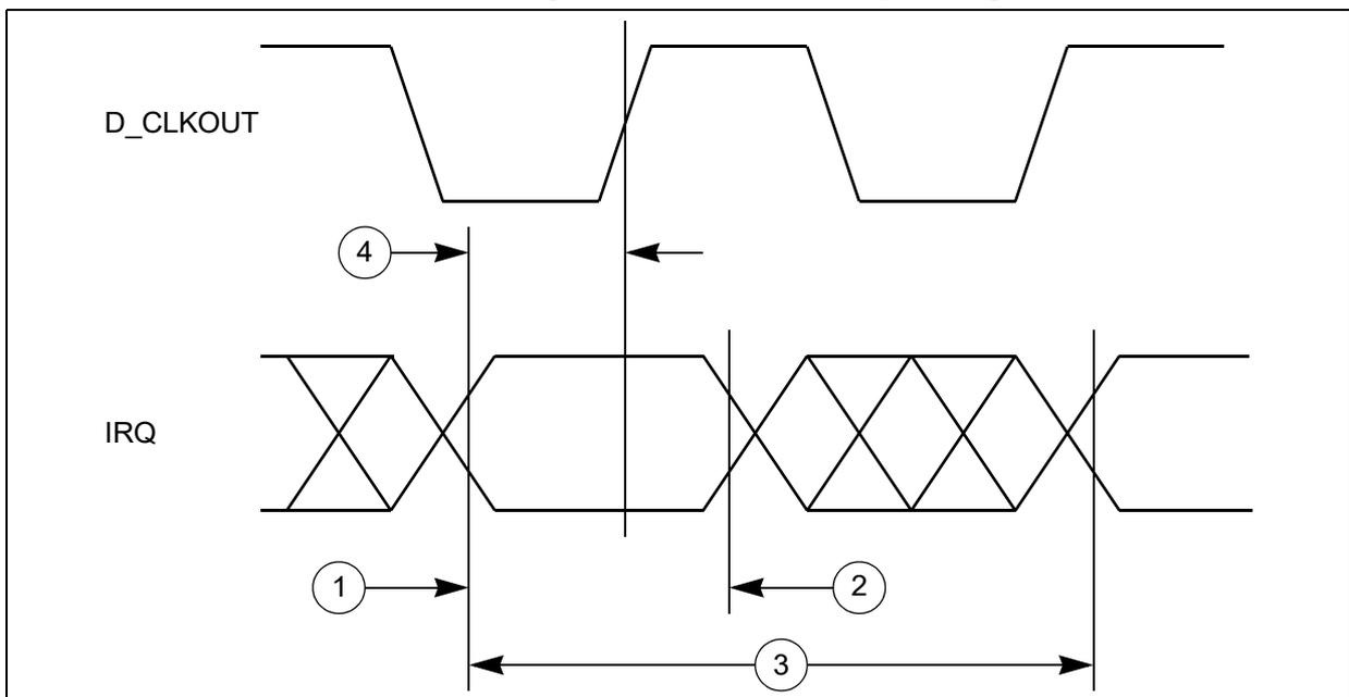
**4.17.2 DSPI timing with CMOS pads**
