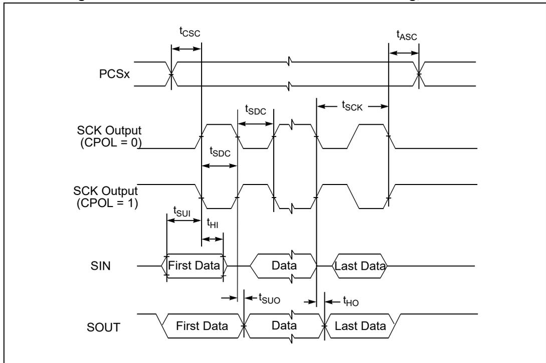
**Figure 31. DSPI CMOS master mode — modified timing, CPHA = 1**
