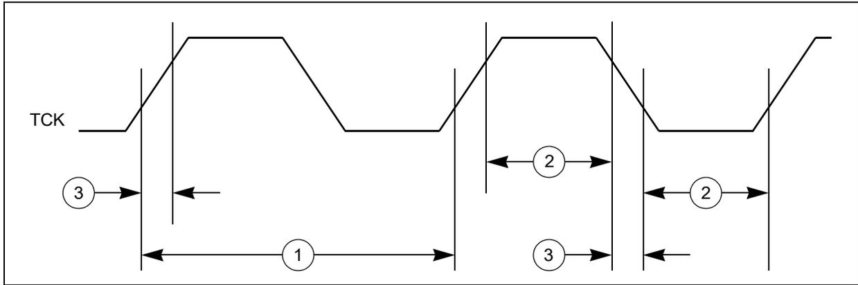
Figure 19. JTAG test access port timing
