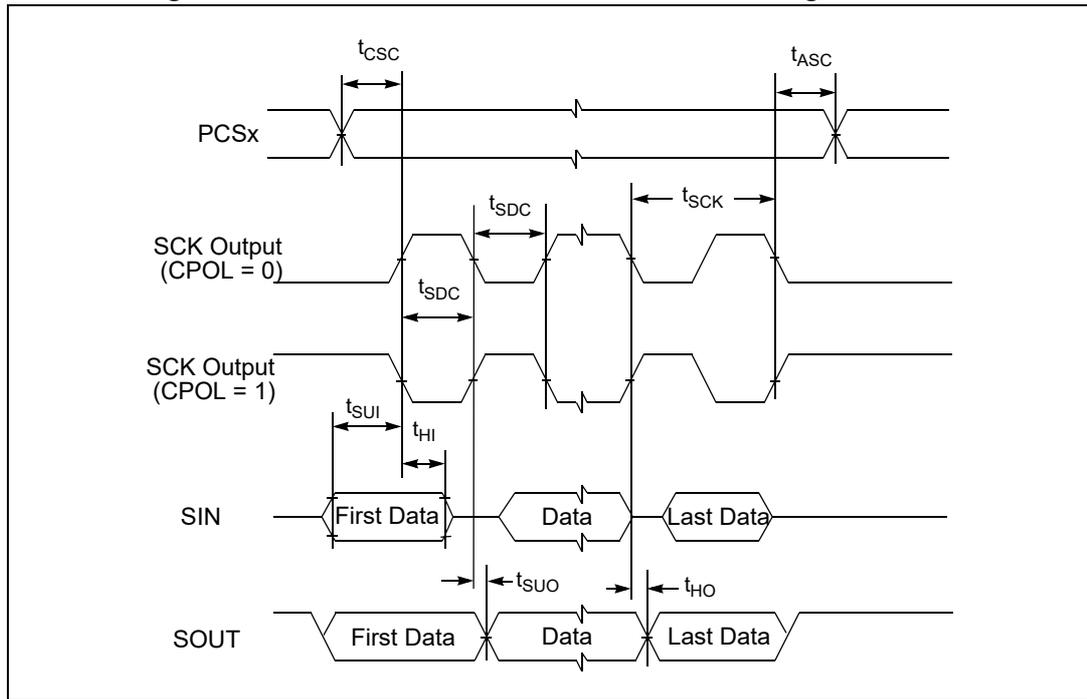
Figure 28. DSPI CMOS master mode — classic timing, CPHA = 1
