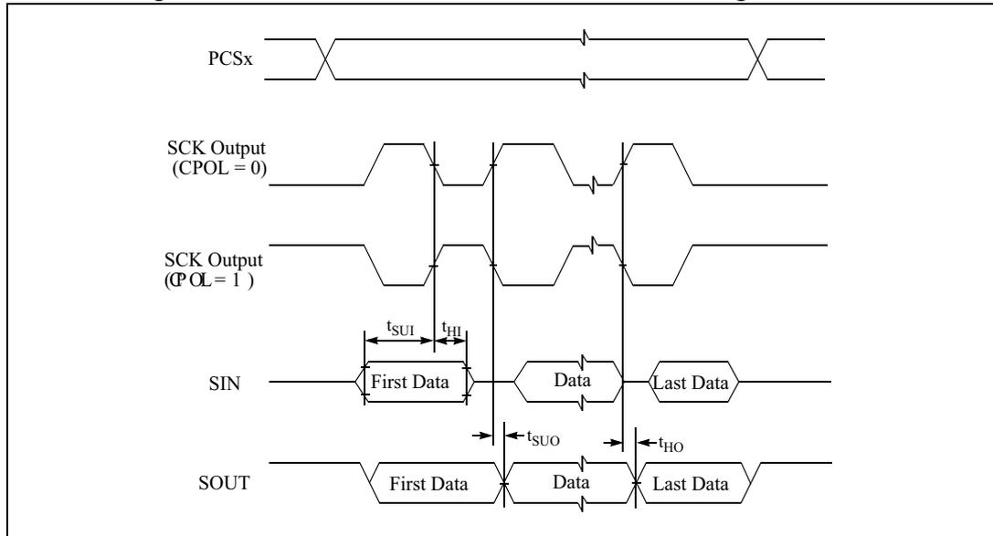
Figure 29. DSPI PCS strobe (PCSS) timing (master mode)
