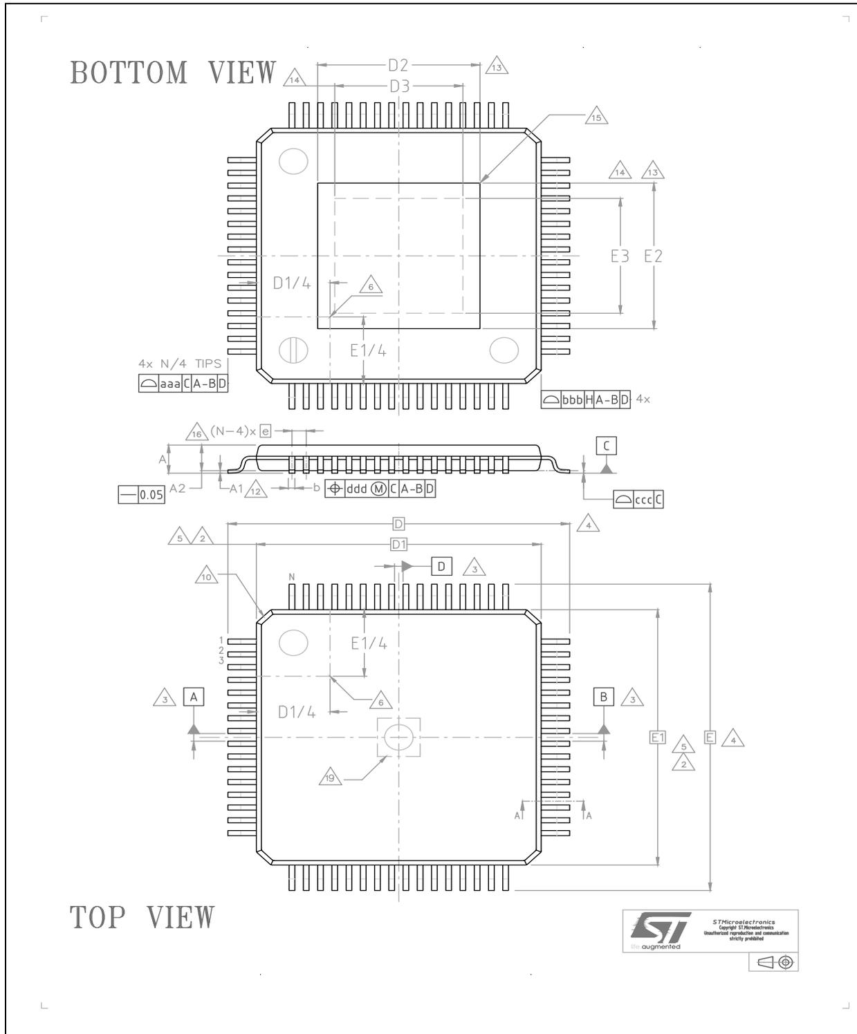
Figure 44. eTQFP64 section A-A
