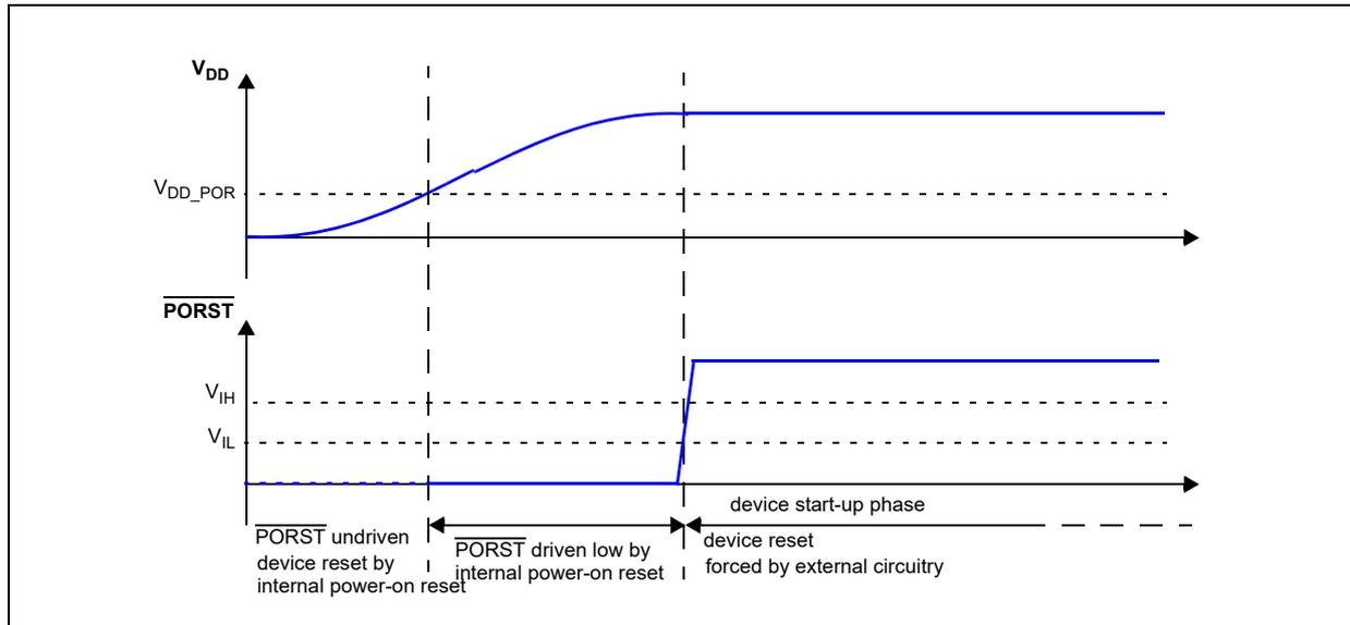
Figure 6 describes device behavior depending on supply signal on PORST:
