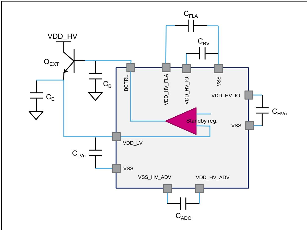
Figure 16. Standby regulator with internal ballast mode
