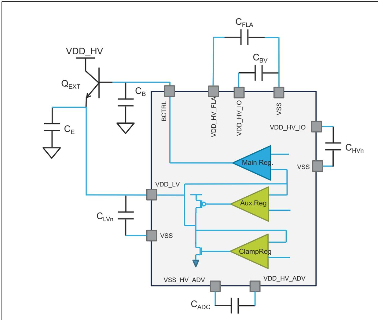
Figure 15. Standby regulator with external ballast mode
