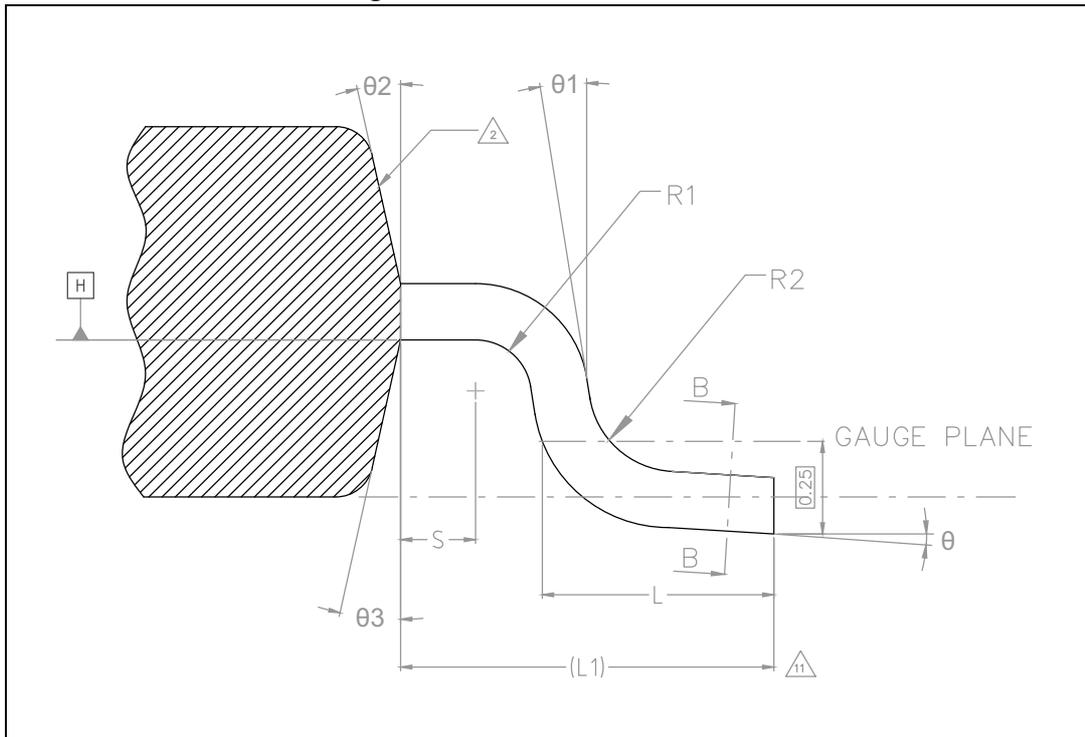
Figure 45. eTQFP64 section B-B
