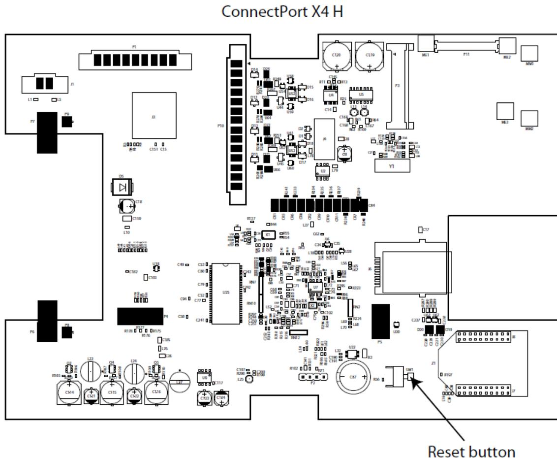
3. Hold the **Reset** button down gently with a non-conductive, small diameter tool (such as wood or plastic) with a blunt end (NOT SHARP or the button could be damaged). Power on the device while holding the Reset button down. On some models, after a few seconds you may see the Status LED blink a 1-1-1 pattern once.
