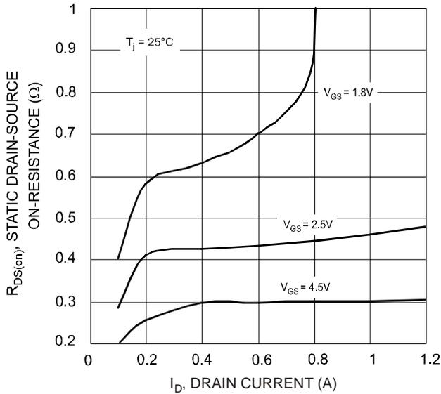
Fig. 7 On-Resistance vs. Drain Current and Gate Voltage
