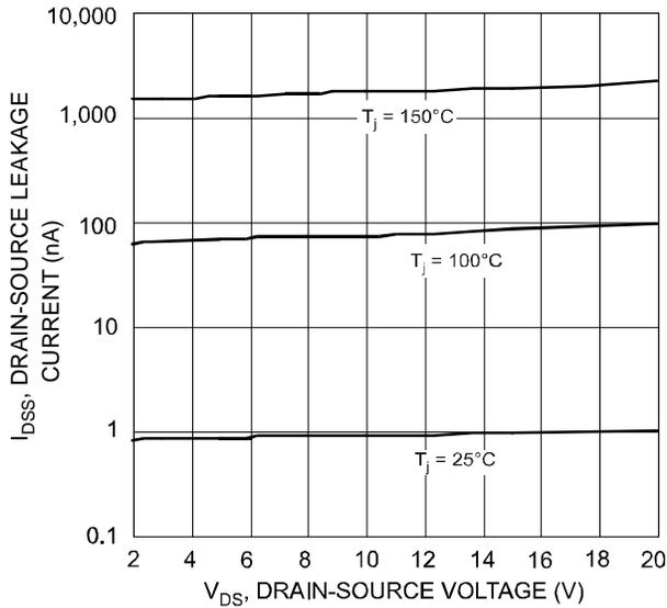
Fig. 9 Drain Source Leakage Current vs. Voltage
