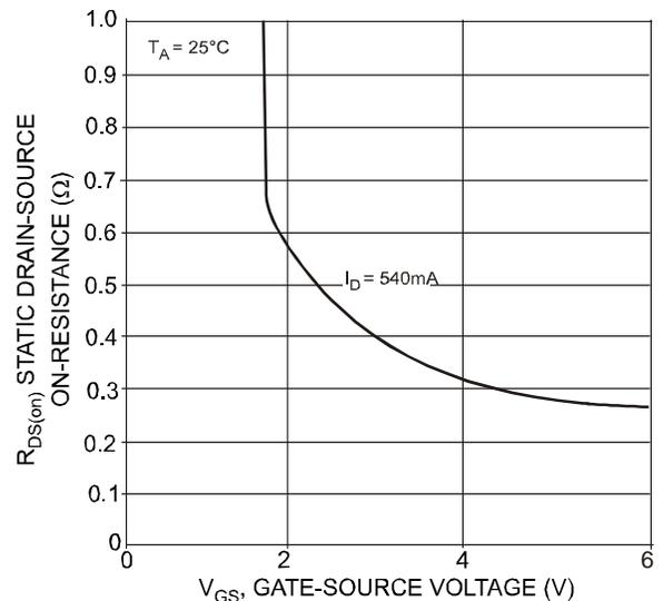
Fig. 6 Static Drain-Source, On-Resistance vs. Gate-Source Voltage
