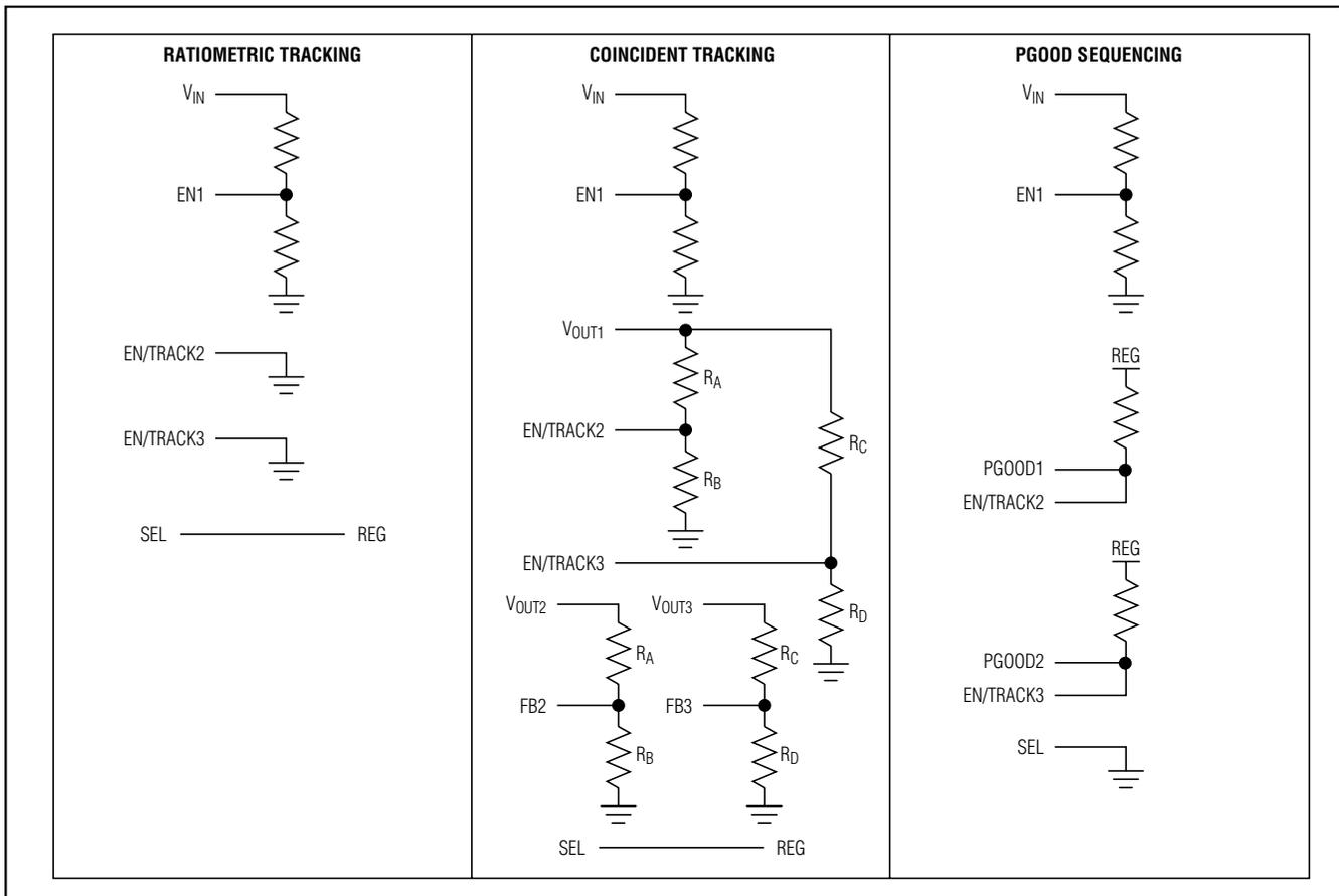
Figure 2. Ratiometric Tracking, Coincident Tracking, PGOOD Sequencing Configurations
