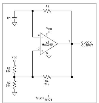
Figure 5. Analog-comparator oscillators produce an arbitrary output frequency of  $f_{OUT} = 1/(R1 \times C1)$ .
