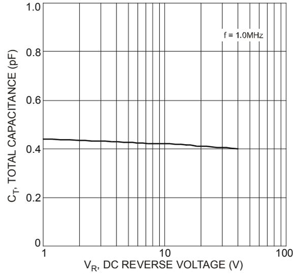
Fig. 4 Total Capacitance vs. Reverse Voltage, Per Element
