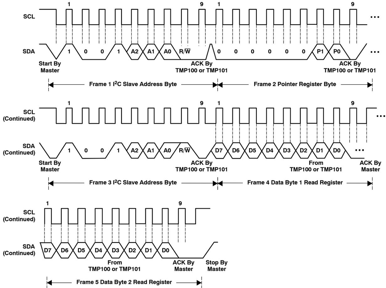
**Figure 6. I<sup>2</sup>C Timing Diagram for Read Word Format**
