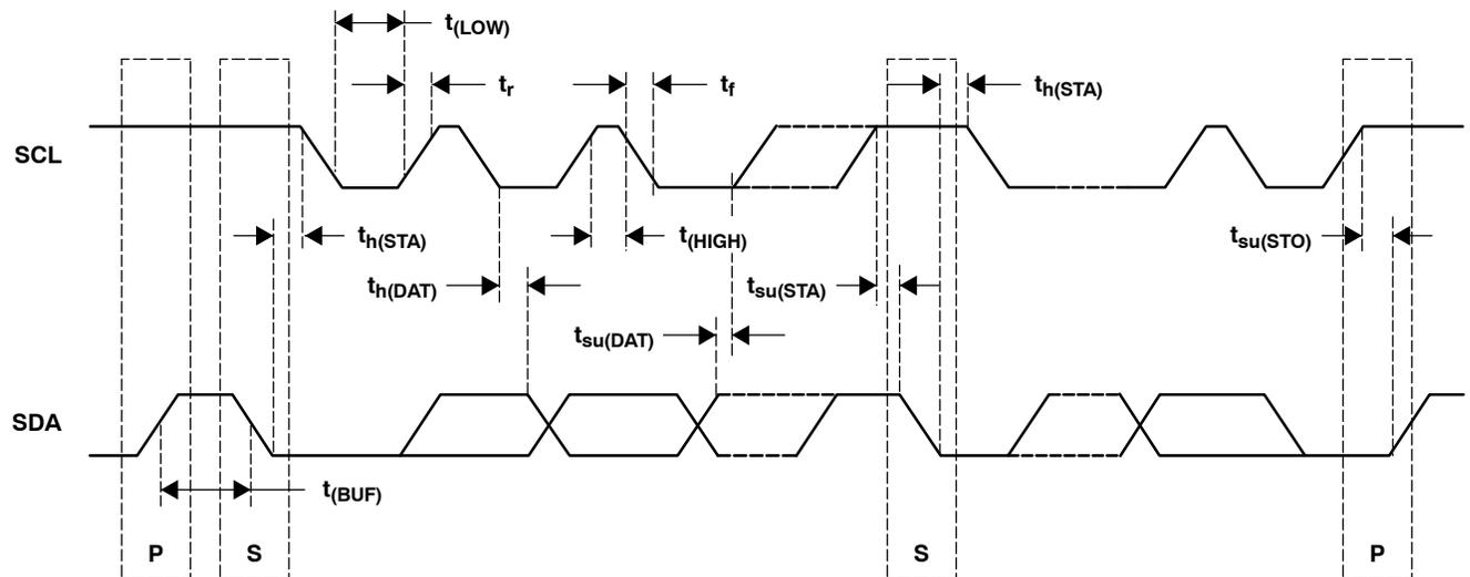
**Figure 4. I<sup>2</sup>C Timing Diagram**
