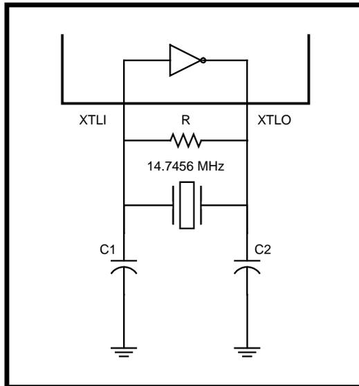
**Figure 5-3 Crystal Oscillator as the Clock Source**
