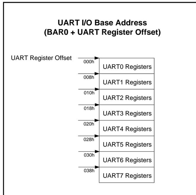
**Figure 7-1 UART Register Block Arrangement in I/O Mode**
