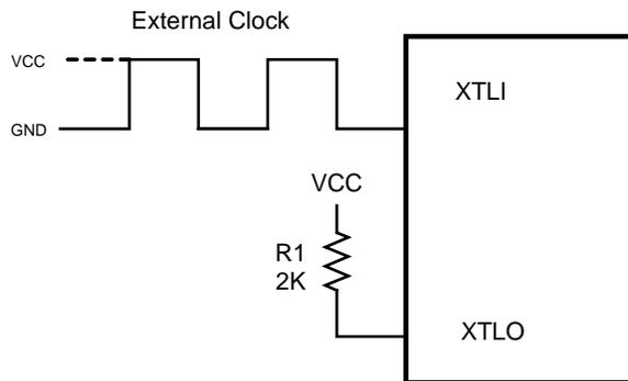
**Figure 5-4 External Clock Source as the Clock Source**
