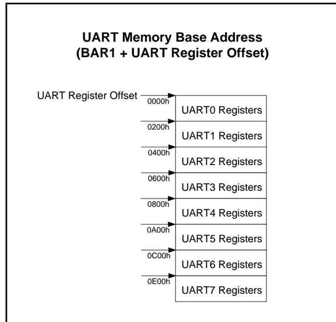
**Figure 7-2 UART Register Block Arrangement in Memory Mode**
