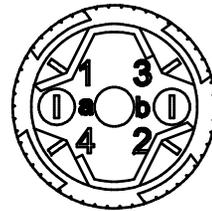
**B** TERMINALS A AND B ARE INCLUDED FOR MECHANICAL SUPPORT ONLY.
