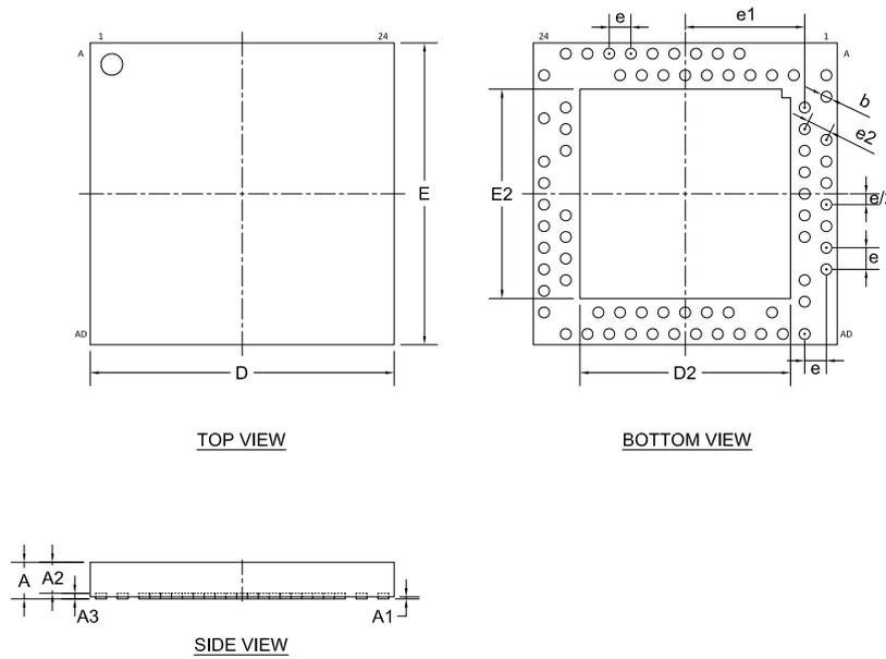
Figure 210: aQFN™ 73 7 x 7 mm package
