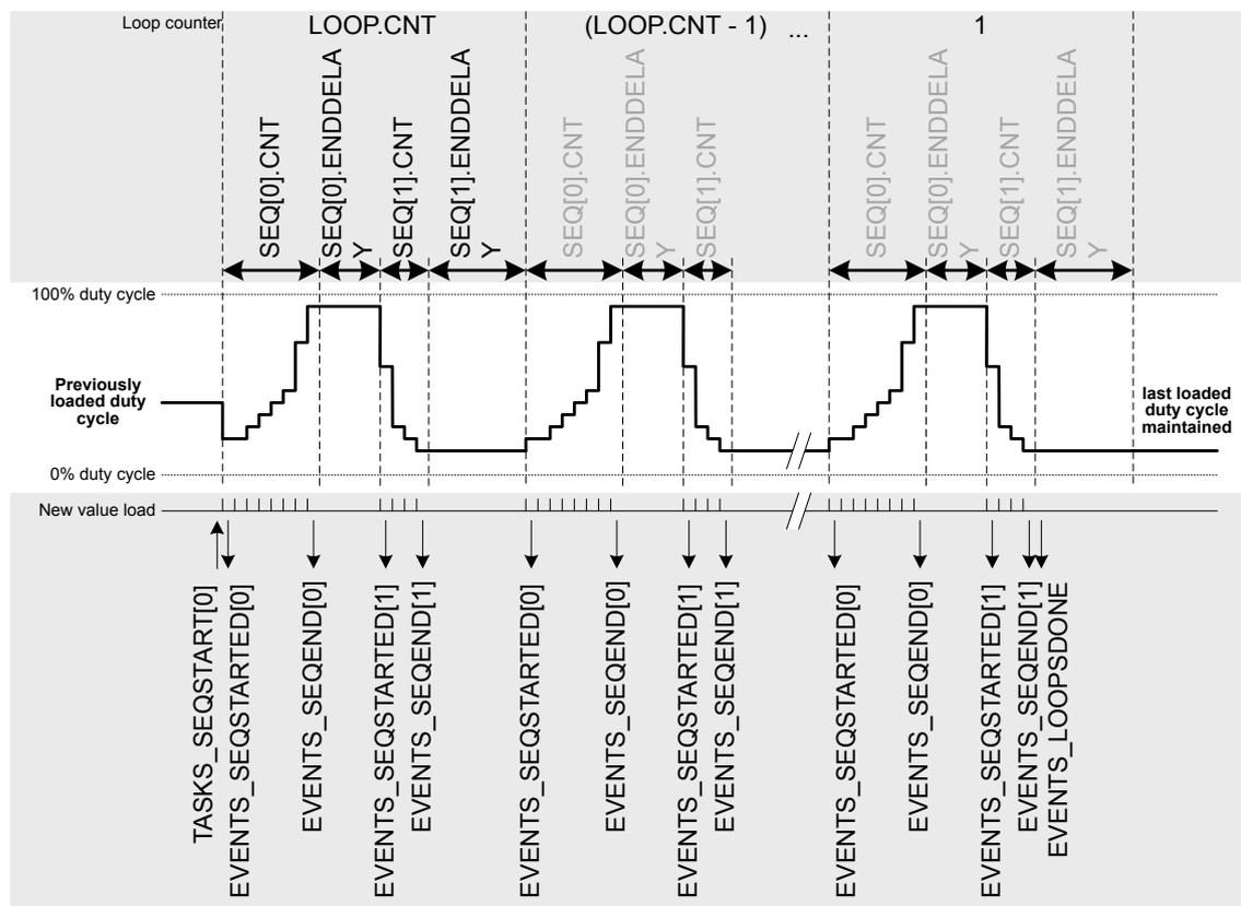
Figure 83: Complex sequence ( $LOOP.CNT > 0$ ) starting with SEQ[0]
