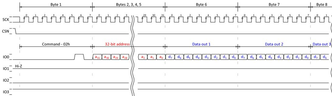
Figure 103: 32-bit PP (page program), SPI MODE = MODE0
