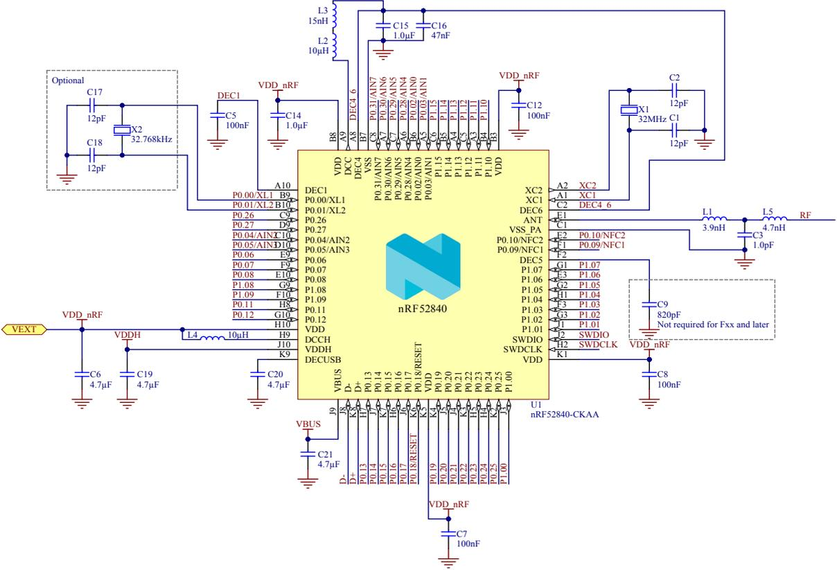
Figure 224: Circuit configuration no. 4 schematic for CKAA WLCSP
