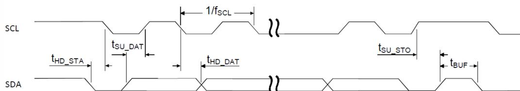
Figure 187: TWIS timing diagram, 1 byte transaction
