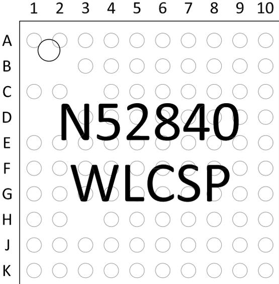
Figure 209: WLCSP ball assignments, top view
