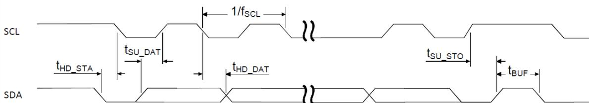
Figure 179: TWIM timing diagram, 1 byte transaction
