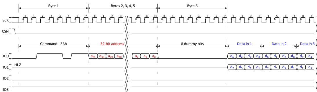
Figure 99: 32-bit READ2O (dual-read output), SPIMODE = MODE0
