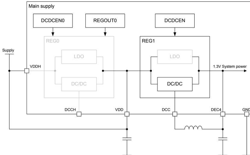
Figure 16: Normal Voltage mode, DC/DC REG1 enabled
