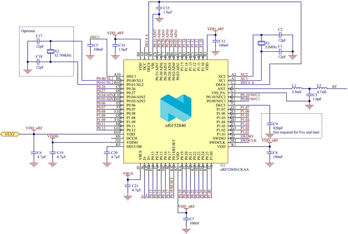
Figure 222: Circuit configuration no. 2 schematic for CKAA WLCSP
