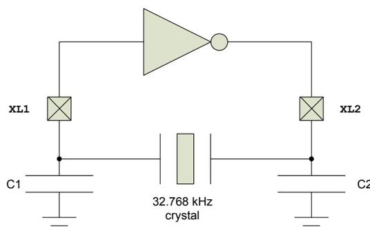
Figure 25: Circuit diagram of the 32.768 kHz crystal oscillator
