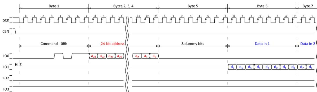
Figure 89: 24-bit FASTREAD, SPI MODE = MODE0
