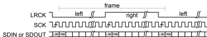
Figure 50:  $I^2S$  format. *CONFIG.SWIDTH* equalling half-frame size.
