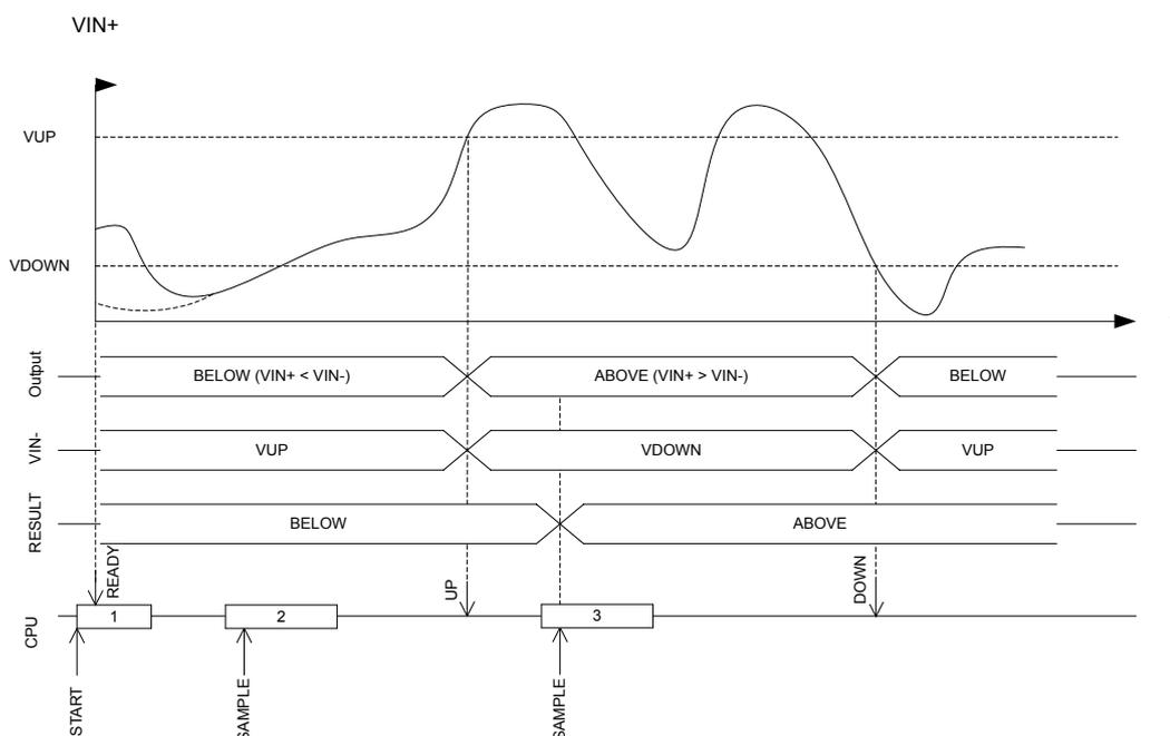
Figure 42: Hysteresis example where  $VIN+$  starts below  $VUP$
