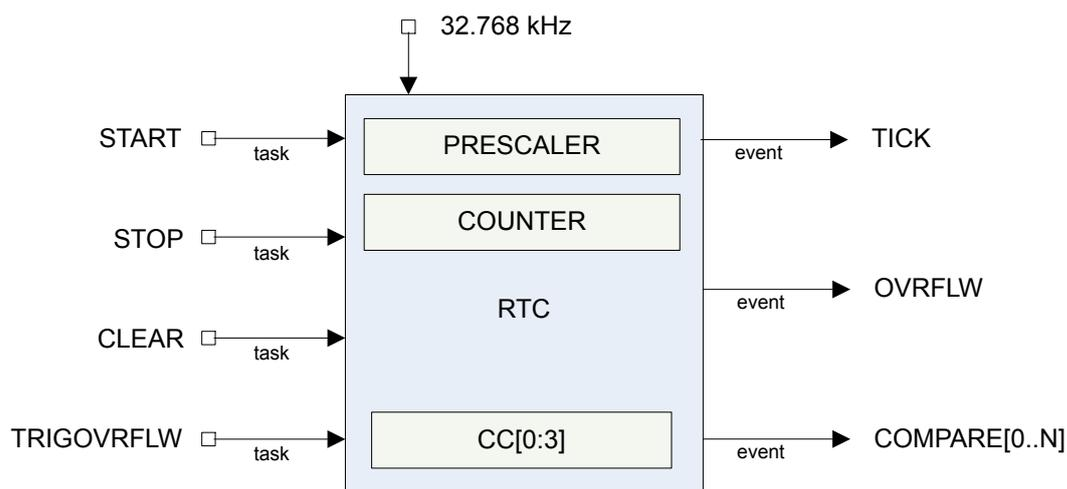
Figure 133: RTC block schematic
