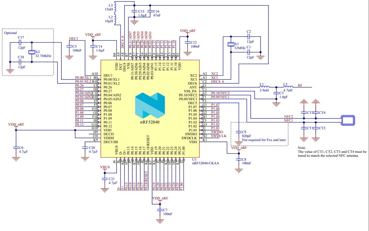
Figure 225: Circuit configuration no. 5 schematic for CKAA WLCSP
