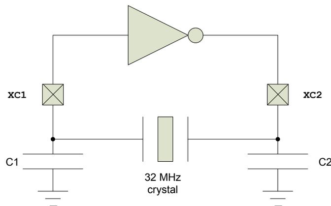
Figure 23: Circuit diagram of the 64 MHz crystal oscillator
