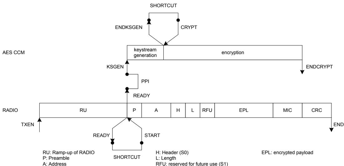
Figure 35: On-the-fly encryption of short packets (MODE.LENGTH = Default) using a PPI connection
