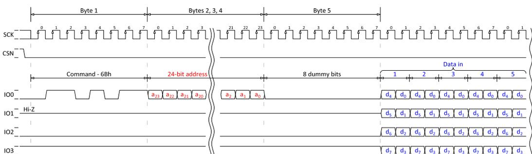
Figure 92: 24-bit READ4O (quad-read output), SPIMODE = MODE0
