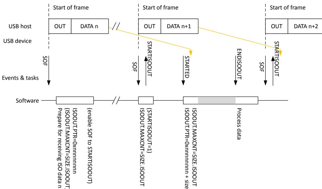
Figure 206: Isochronous OUT transfer
