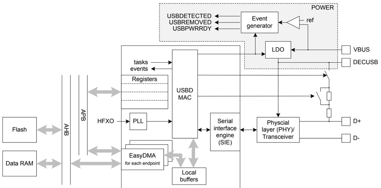
Figure 195: USB device block diagram
