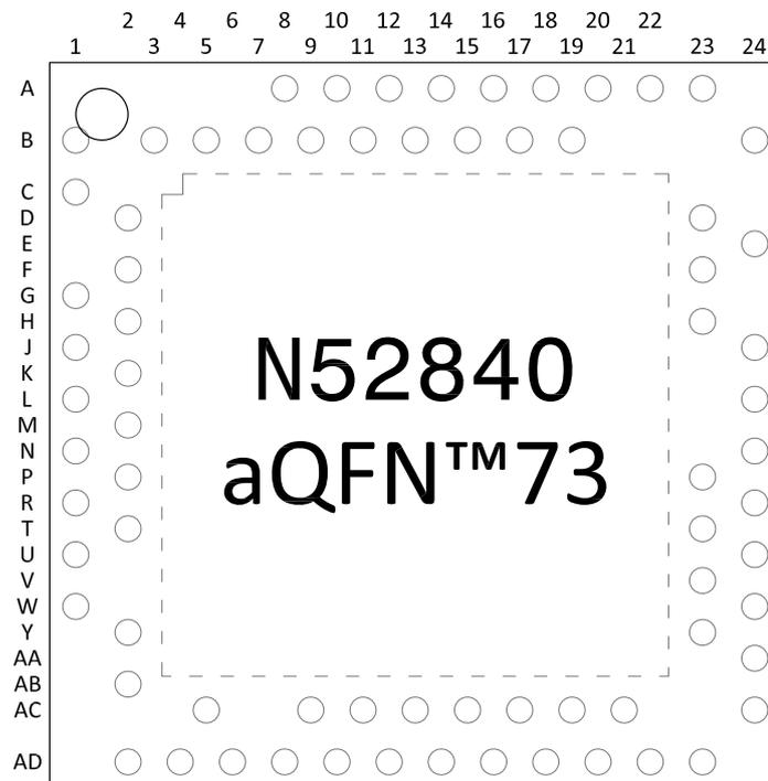
Figure 207: aQFN™73 ball assignments, top view
