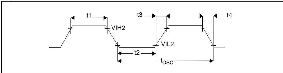
Note: When Direct Drive is selected, an external clock source can be used to drive XTAL1. The maximum frequency of the external clock source depends on the duty cycle: when 64MHz is used, 50% duty cycle shall be granted (low phase = high phase = 7.8ns); when for instance 32MHz is used, a 25% duty cycle can be accepted (minimum phase, high or low gain, equal to 7.8ns).
