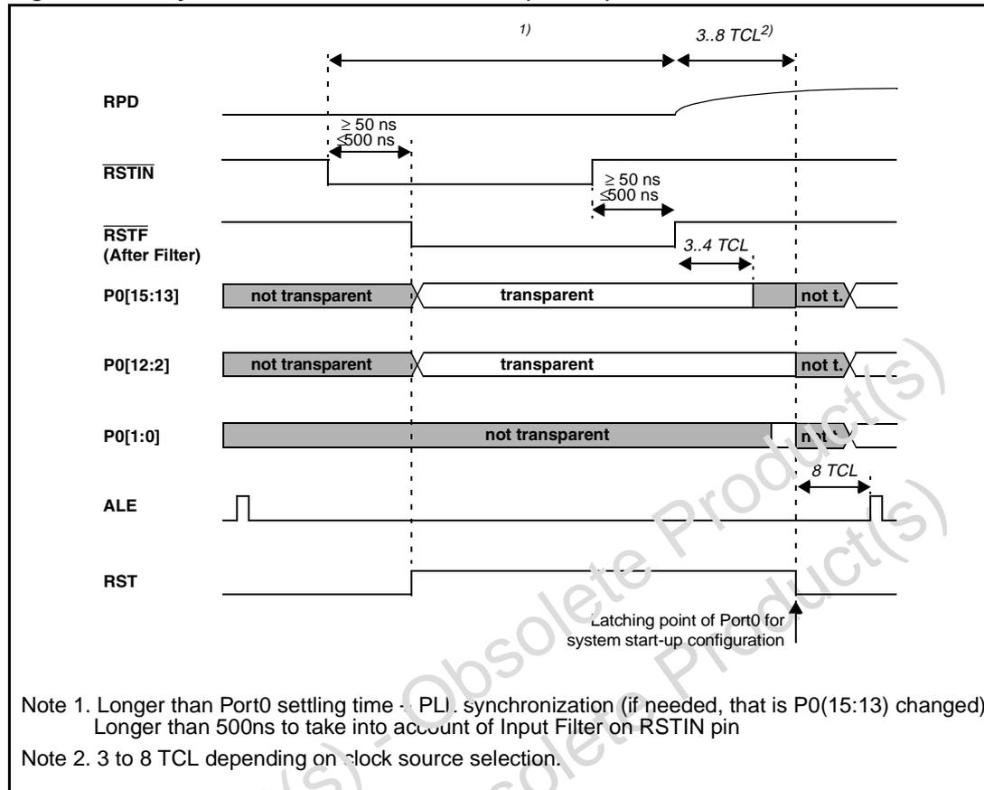
**Exit from asynchronous reset state**
