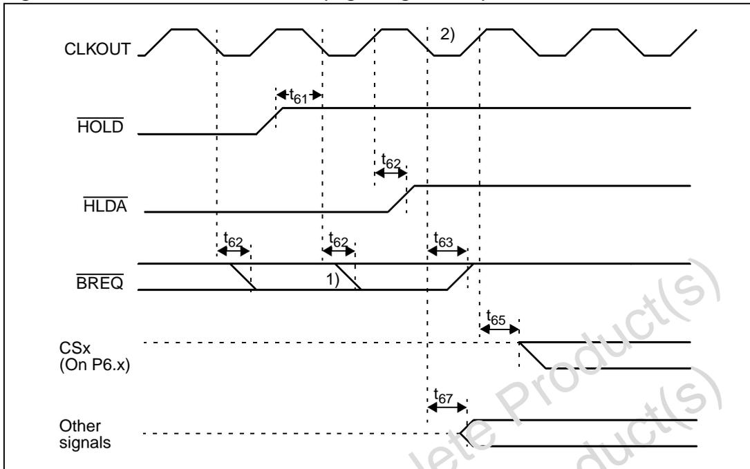
1. This is the last chance for BREQ to trigger the indicated regain-sequence. Even if BREQ is activated earlier, the regain-sequence is initiated by HOLD going high. Please note that HOLD may also be deactivated without the ST10F271 requesting the bus.
