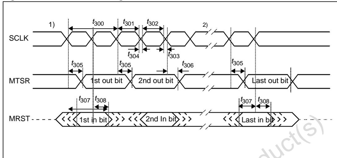
1. The phase and polarity of shift and latch edge of SCLK is programmable. This figure uses the leading clock edge as shift edge (drawn in bold), with latch on trailing edge (SSCPH = 0b, while clock line is low, leading clock edge is low-to-high transition (SSCPO = 0b).
