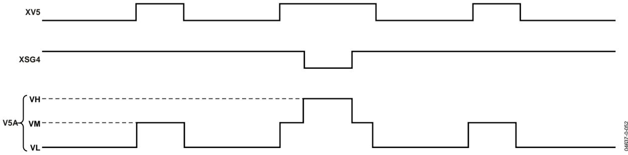
Figure 62. XV5, XSG4, and V5A Output Polarities
