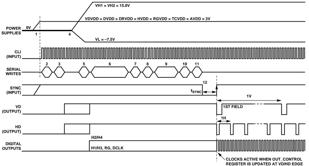
Figure 67. Recommended Power-Up Sequence and Synchronization, Master Mode
