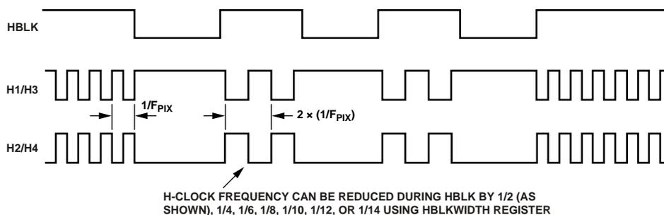
Figure 27. Generating Wide H-Clock Pulses during HBLK Interval
