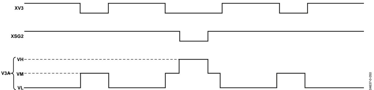
Figure 60. XV3, XSG2, and V3A Output Polarities
