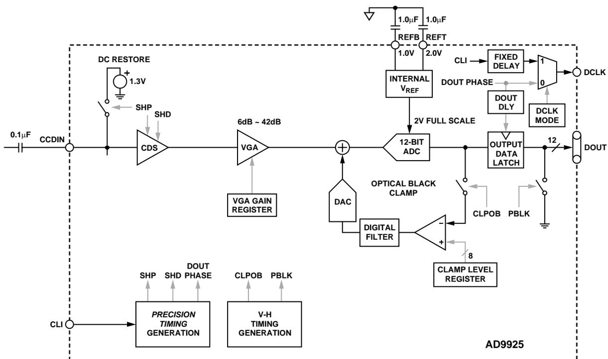
Figure 55. Analog Front End Functional Block Diagram
