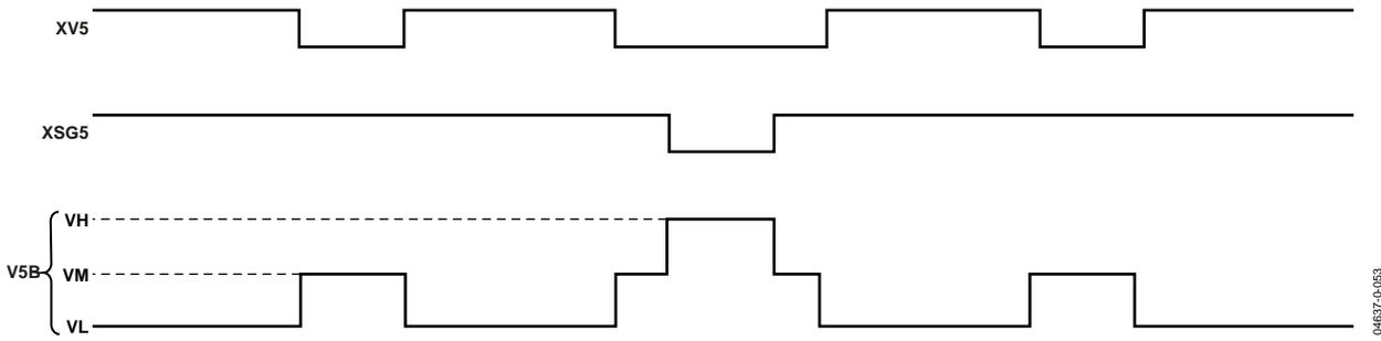
Figure 63. XV5, XSG5, and V5B Output Polarities
