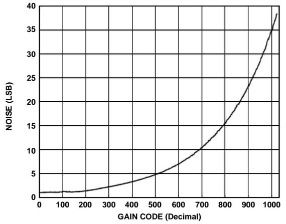
Figure 12. Total Output Noise vs. VGA Gain
