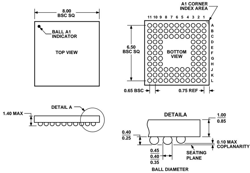
Figure 78. 96-Lead Chip Scale Package Ball Grid Array [CSP\_BGA] (BC-96)
