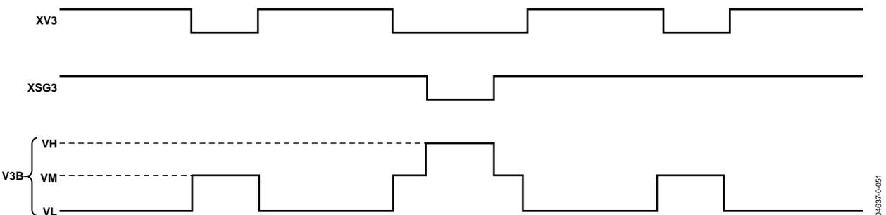
Figure 61. XV3, XSG3, and V3B Output Polarities
