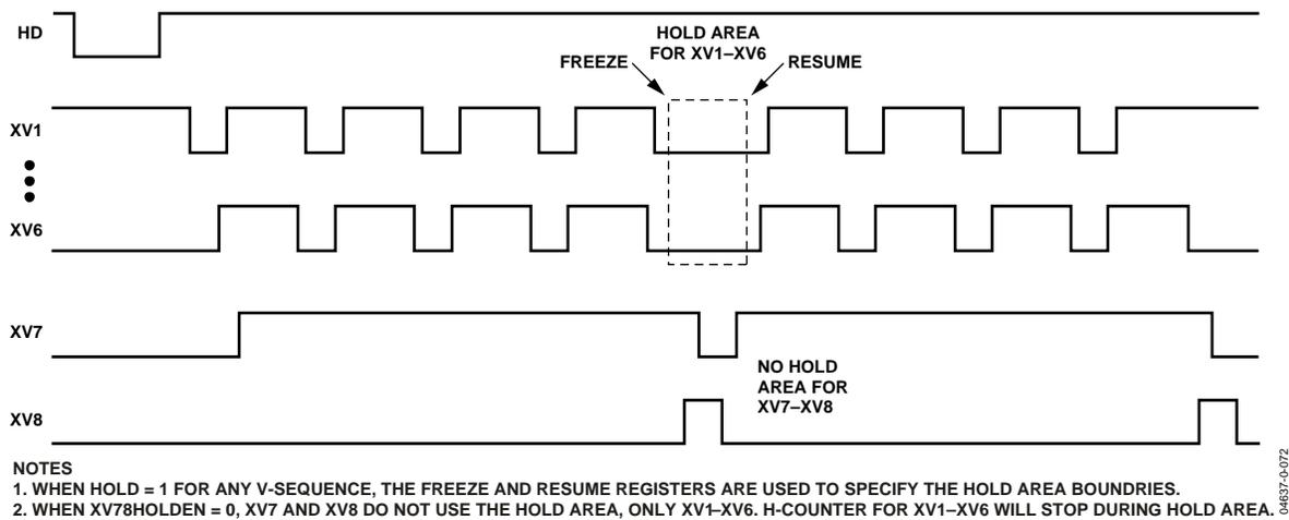
Figure 34. Vertical Hold Area Using the FREEZE/RESUME Registers
