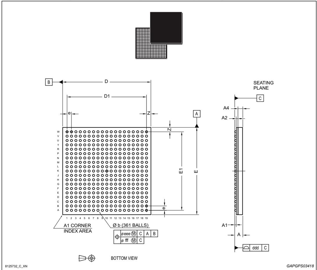
Table 2. LFBGA361 (16x16x1.7 mm) package mechanical data
