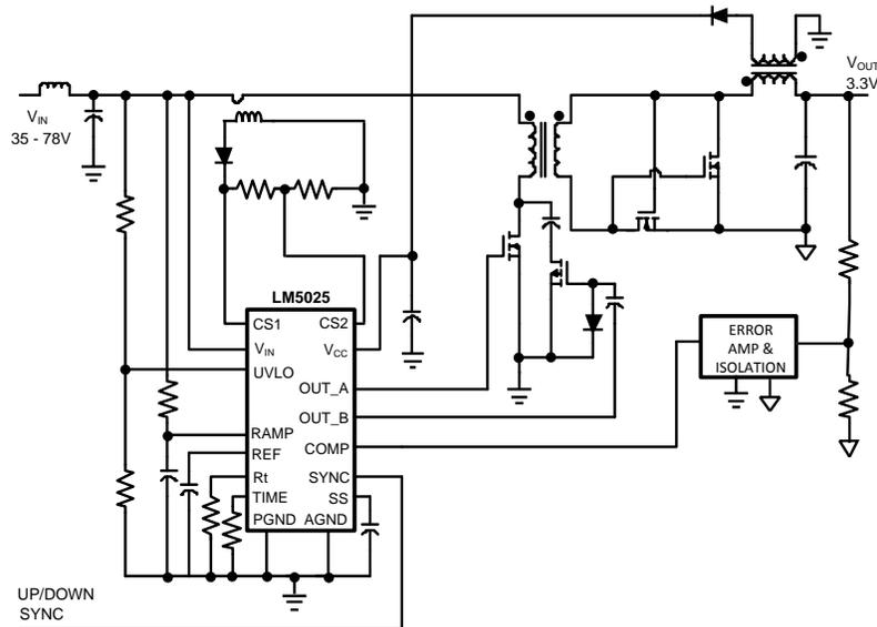
**Figure 13. Simplified Active Clamp Forward Power Converter**
