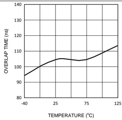
Figure 6. Overlap Time vs Temperature  $R_{SET} = 38 \text{ K}$
