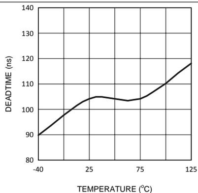
Figure 8. Dead Time vs Temperature R<sub>SET</sub> = 29.5 K
