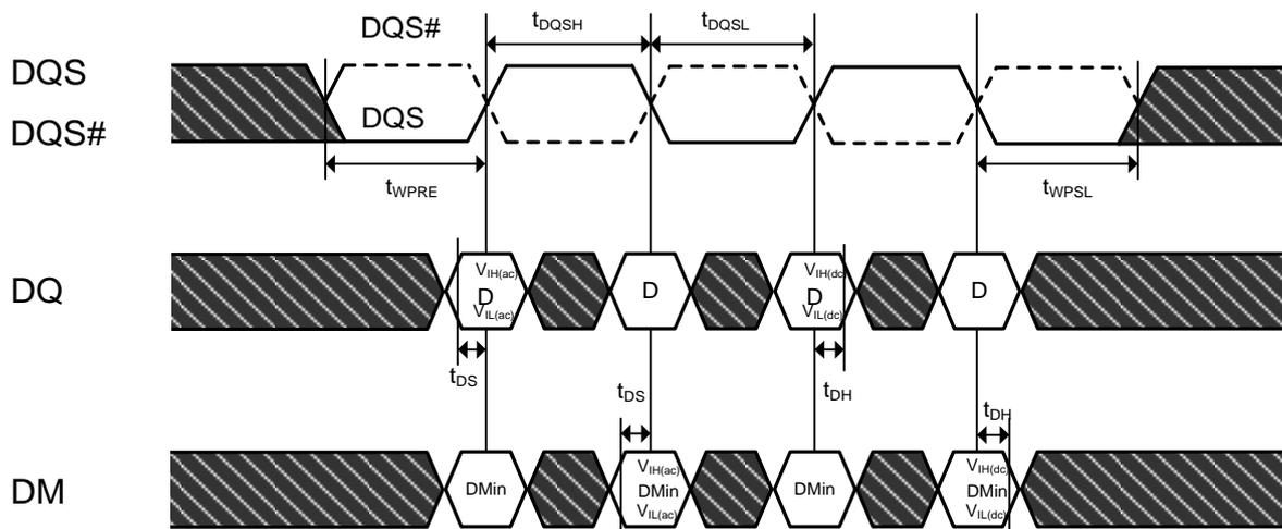
**Figure 27. Burst write operation: RL=5 (AL=2, CL=3), WL=4, BL=4**
