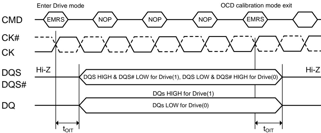
NOTE : Drive mode, both Drive(1) and Drive(0), is used for controllers to measure DDR2 SDRAM Driver impedance. In this mode, all outputs are driven out t<sub>OIT</sub> after "enter drive mode" command and all output drivers are turned-off t<sub>OIT</sub> after "OCD calibration mode exit" command.
