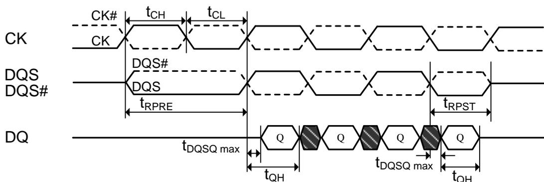
Figure 21. Burst read operation: RL=5 (AL=2, CL=3, BL=4)
