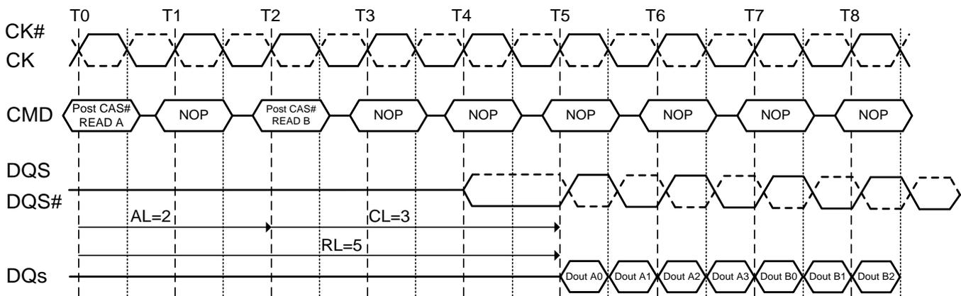
**NOTE :** The seamless burst read operation is supported by enabling a read command at every other clock for BL = 4 operation, and every 4 clock for BL =8 operation. This operation is allowed regardless of same or different banks as long as the banks are activated.
