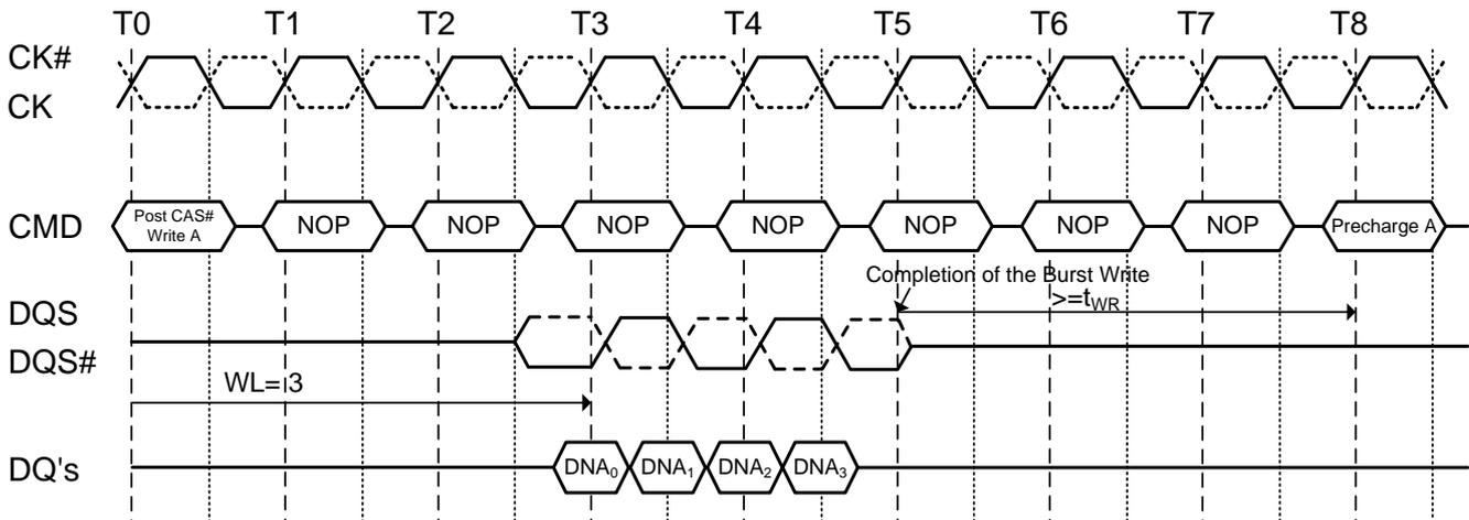
**Figure 39. Burst write followed by precharge:  $WL = (RL-1) = 4$**
