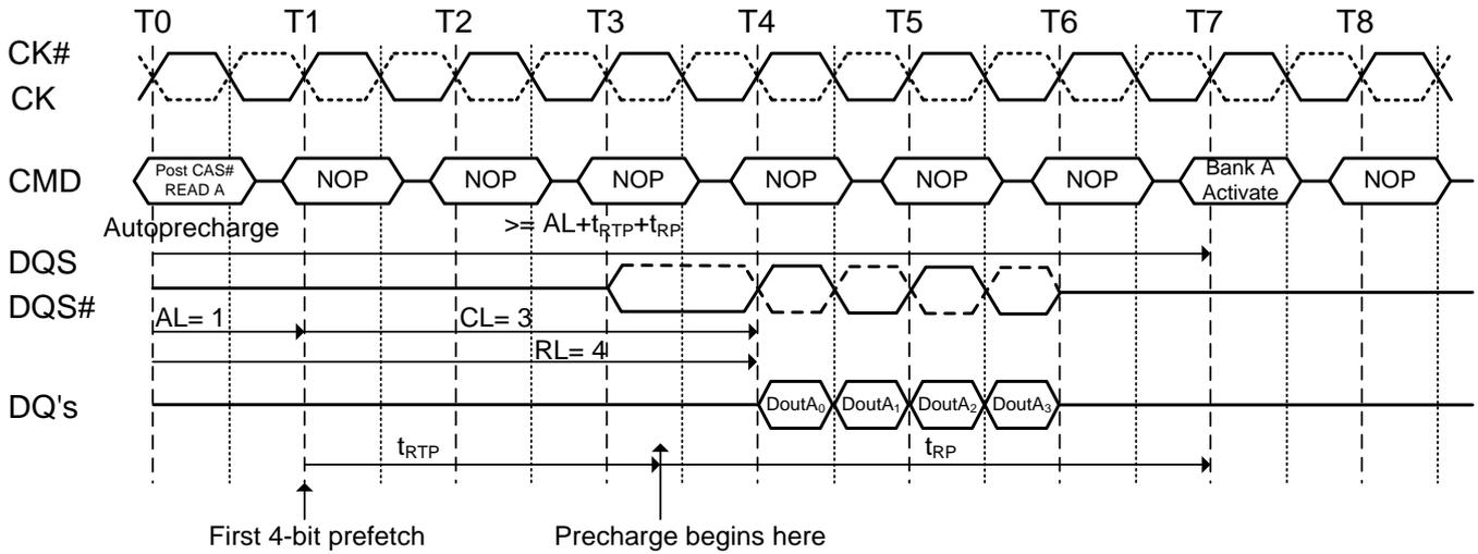
**Figure 42. Burst read operation with auto precharge followed by activation to the same bank ( $t_{RC}$  Limit):  $RL=5(AL=2, CL=3, \text{internal } t_{RCD}=3, BL=4, t_{RTP} \leq 2 \text{ clocks})$**
