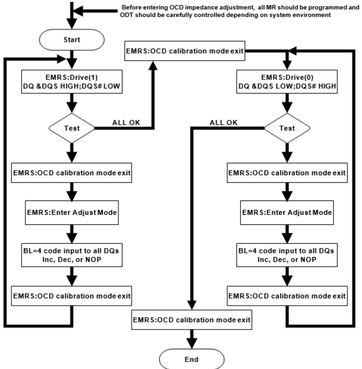
**Extended mode register for OCD impedance adjustment**
