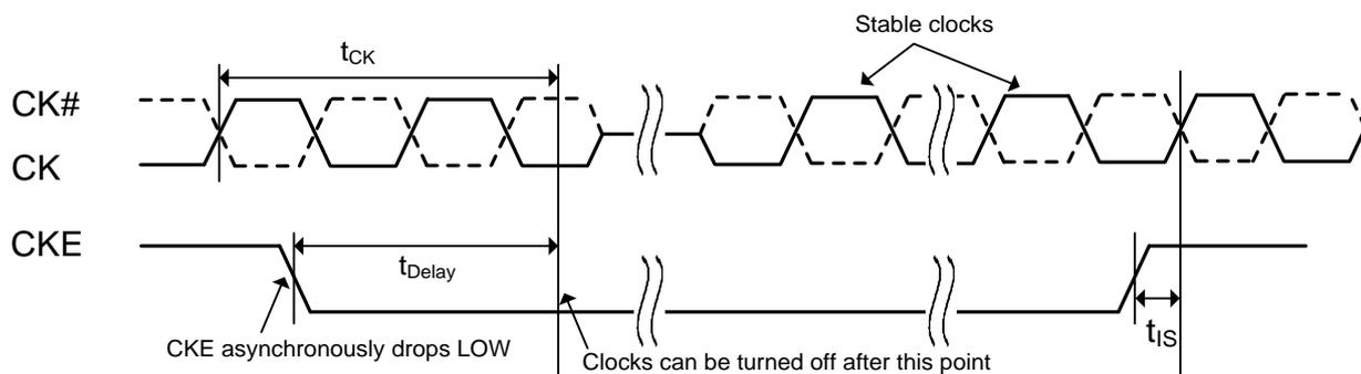
**Figure 60. Clock frequency change in precharge power down mode**
