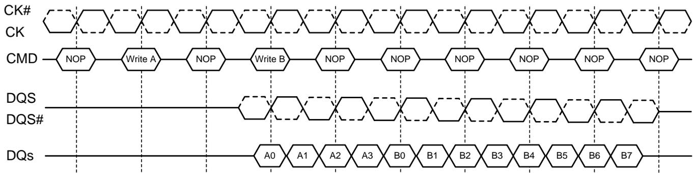
**NOTE 1:** Write burst interrupt function is only allowed on burst of 8. Burst interrupt of 4 is prohibited.
