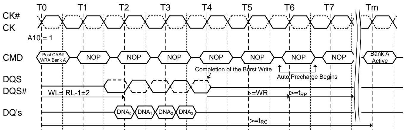
**Figure 45. Burst write with auto-precharge ( $WR+t_{RP}$ ):  $WL=4, WR=2, BL=4, t_{RP}=3$**
