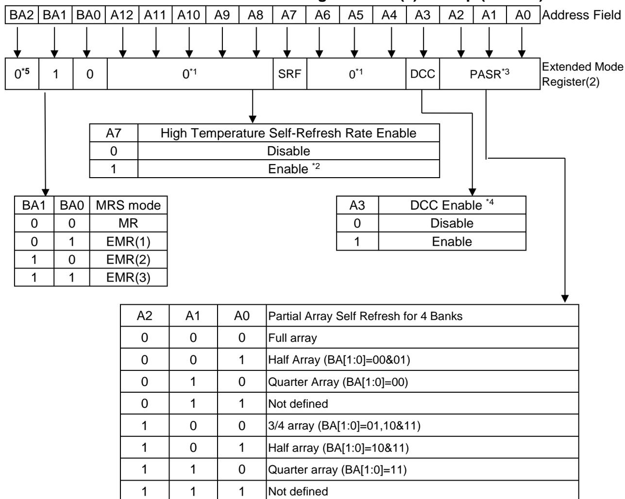
**Note 1:** The rest bits in EMRS(2) are reserved for future use and all bits in EMRS(2) except A0-A2, A7, BA0 and BA1 must be programmed to 0 when setting the extended mode register(2) during initialization.
