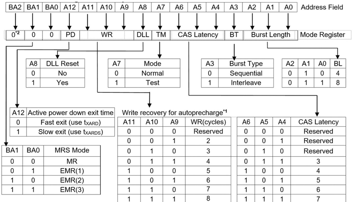
**Note 1:** For DDR2-800, WR min is determined by  $t_{CK} (avg)$  max and WR max is determined by  $t_{CK}(avg)$  min.  $WR [cycles] = RU \{t_{WR}[ns]/t_{CK}(avg)[ns]\}$ , where RU stands for round up. The mode register must be programmed to this value. This is also used with  $t_{RP}$  to determine  $t_{DAL}$ .
