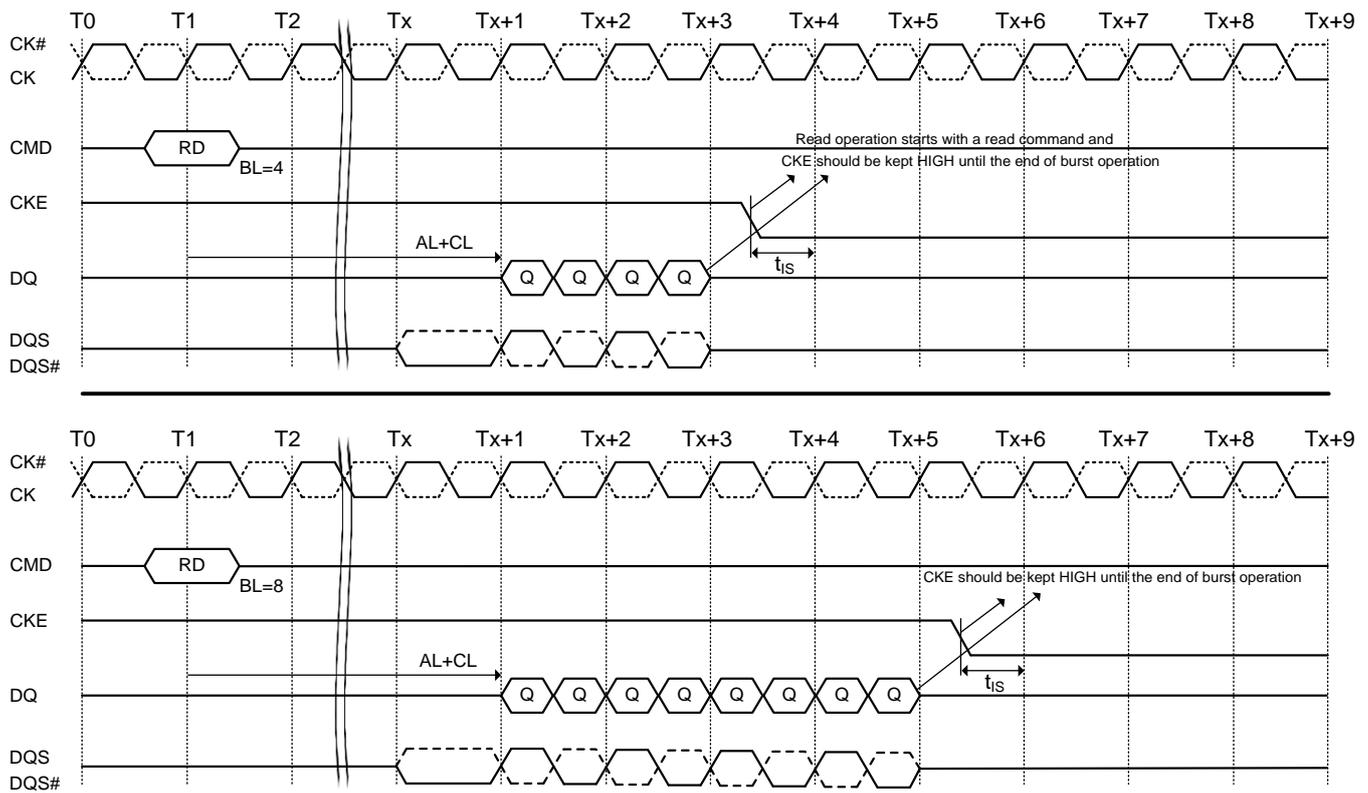
**Figure 52. Read with autoprecharge to power-down entry**
