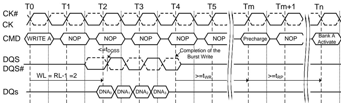
**Figure 29. Burst write followed by burst read:
