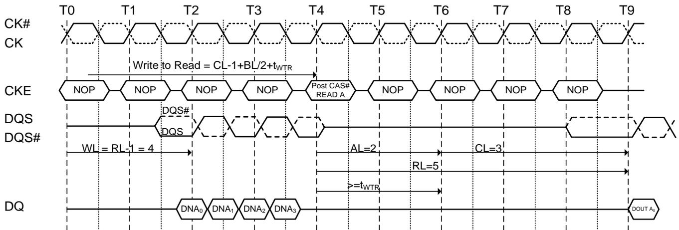
**NOTE :** The minimum number of clock from the burst write command to the burst read command is  $\lceil CL-1 + BL/2 + t_{WTR} \rceil$ . This  $t_{WTR}$  is not a write recovery time ( $t_{WR}$ ) but the time required to transfer the 4 bit write data from the input buffer into sense amplifiers in the array.  $t_{WTR}$  is defined in the timing parameter table of this standard.
