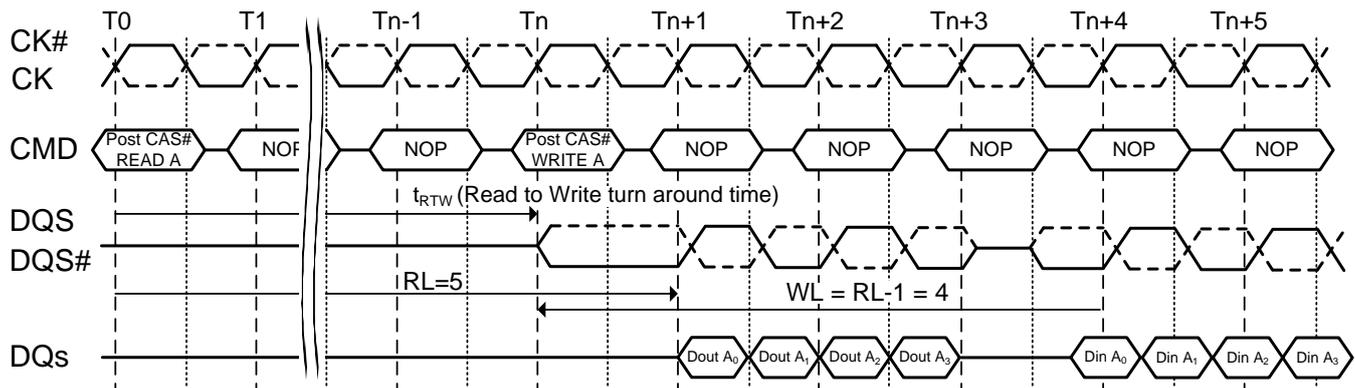
**NOTE :** The minimum time from the burst read command to the burst write command is defined by a read-to-write-turn-around-time, which is 4 clocks in case of BL = 4 operation, 6 clocks in case of BL = 8 operation.
