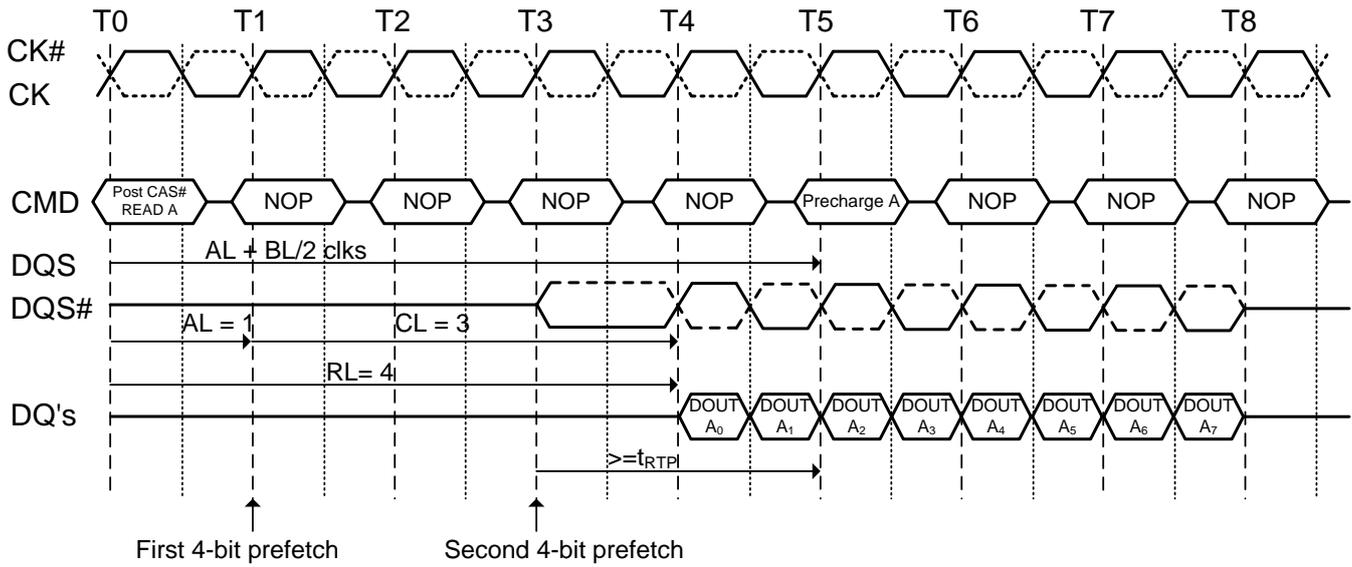
**Figure 35. Burst read operation followed by precharge:**
