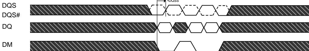
Figure 33. Burst read operation followed by precharge:
