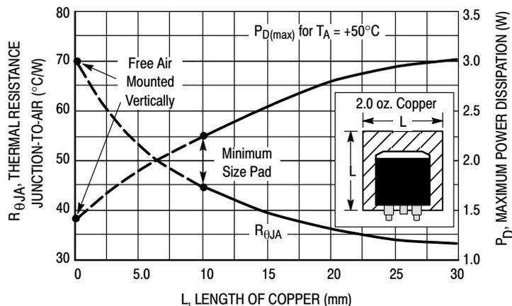
Figure 12. D<sup>2</sup>PAK Thermal Resistance and Maximum Power Dissipation versus P.C.B. Copper Length
