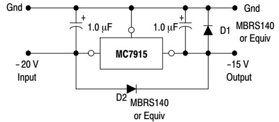
Figure 11. Protection Diodes
