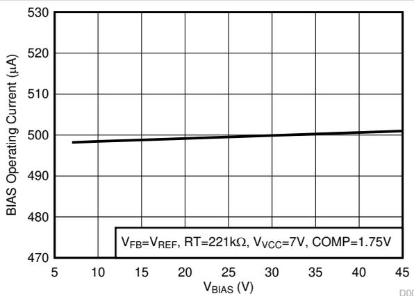
**Figure 8-9.  $I_{OPERATING(BIAS)}$  including RT current vs  $V_{BIAS}$**
