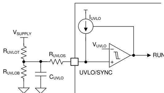
**Figure 9-4. Line UVLO using Three UVLO Resistors**
