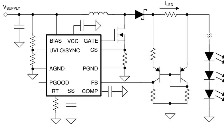
**Figure 10-13. LED Driver with High-Side Current Sensing**
