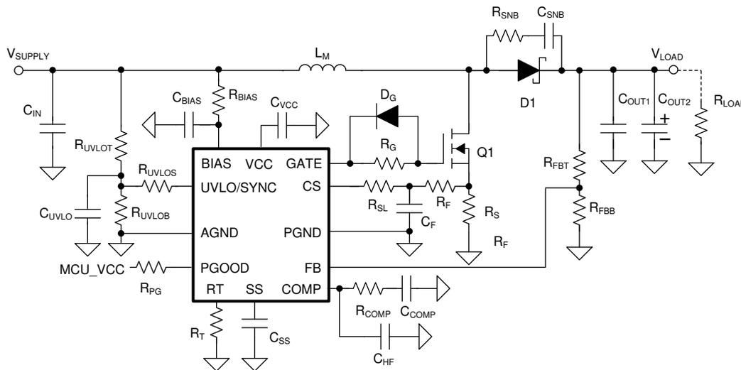
**Figure 10-1. Typical Boost Converter Circuit With Optional Components**
