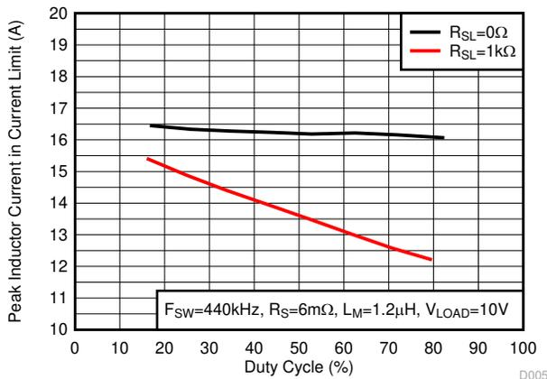
Figure 8-5. Peak Current Limit vs Duty Cycle
