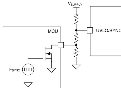
**Figure 9-14. UVLO, Standby, and Clock Synchronization (b)**
