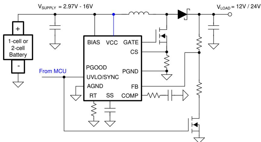
**Figure 10-5. Emergency-call / Boost On-Demand / Portable Speaker**
