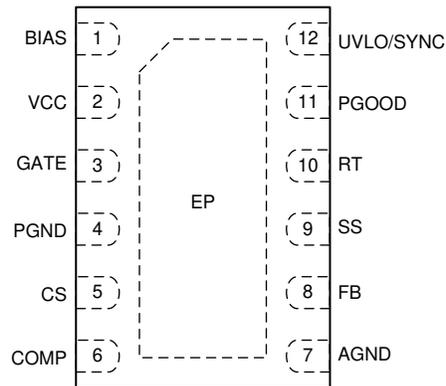
Figure 7-1. 12-Pin WSON DSS Package (Top View)
