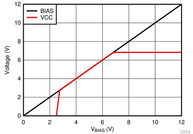
Figure 8-4. V<sub>CC</sub> vs V<sub>BIAS</sub> (No Load)
