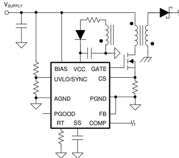
**Figure 9-7. External VCC Supply (BIAS  $\geq$  VCC)**
