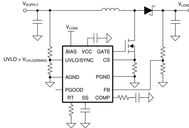
**Figure 9-6. Decrease the Minimum Operating Voltage After Start-Up**
