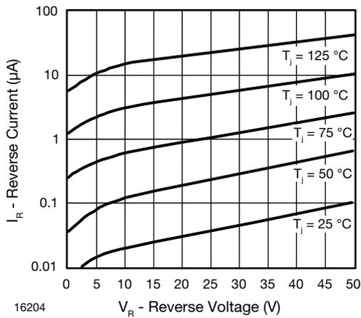
Fig. 1 - Reverse Current vs. Reverse Voltage
