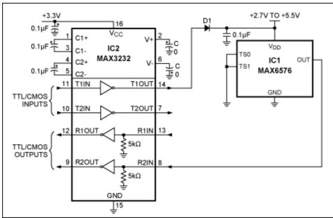
Figure 1. RS-232 powered temperature sensor.
