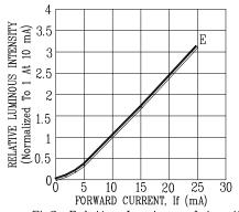
Fig3. Relative Luminous Intensity
