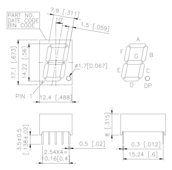
NOTES: 1.All dimensions are in millimeters. Tolerances are  $\pm~0.25~\text{mm}$  (0.01") unless otherwise noted.
