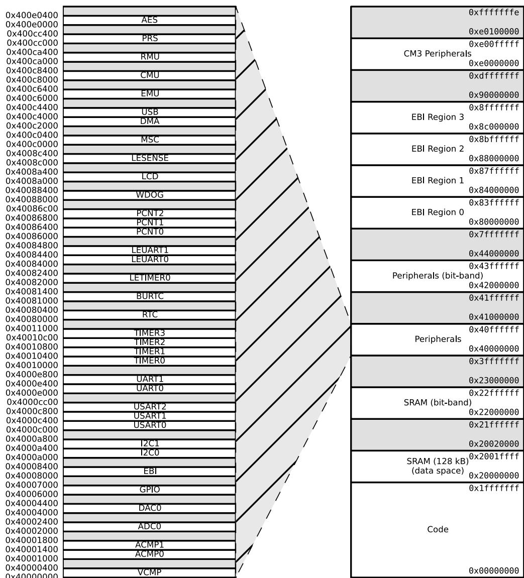
Figure 3.3. System Address Space with Peripheral Listing
