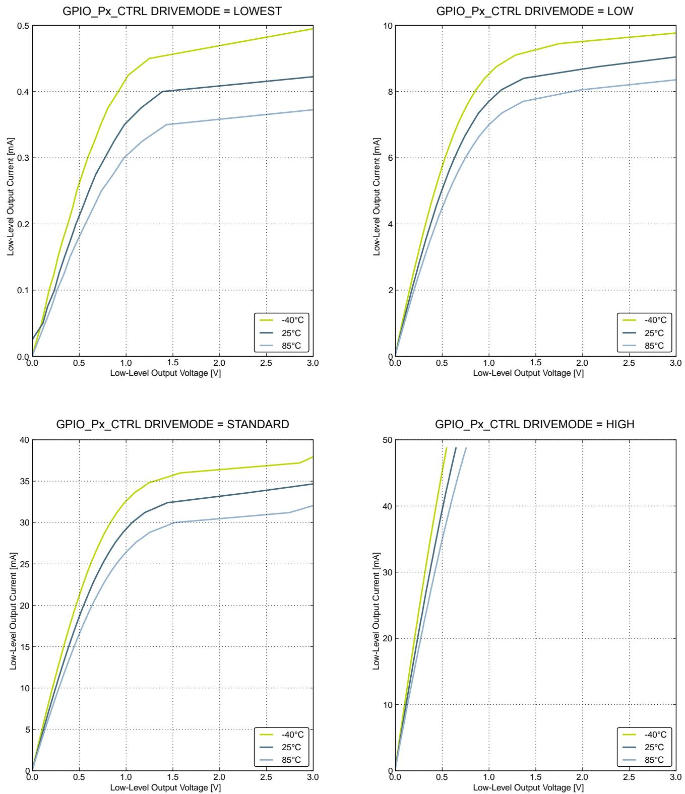
**Figure 4.12. Typical Low-Level Output Current, 3 V Supply Voltage**
