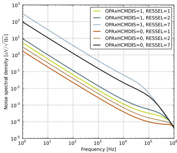
Figure 4.35. OPAMP Voltage Noise Spectral Density(Non-Unity Gain)
