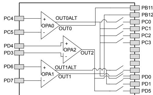
Figure 5.40. Opamp Pinout
