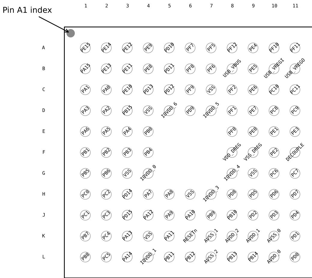
**Figure 5.39. EFM32GG990 Pinout (top view, not to scale)**
