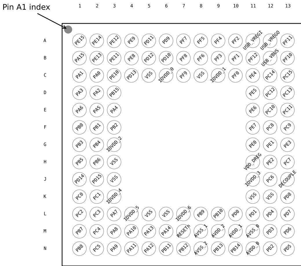
**Figure 5.19. EFM32GG395 Pinout (top view, not to scale)**
