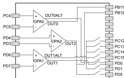
**Figure 5.22. Opamp Pinout**
