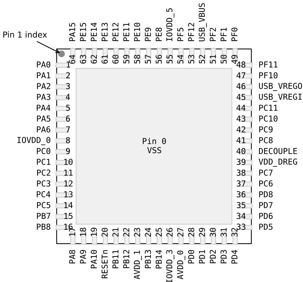
**Figure 5.11. EFM32GG330 Pinout (top view, not to scale)**
