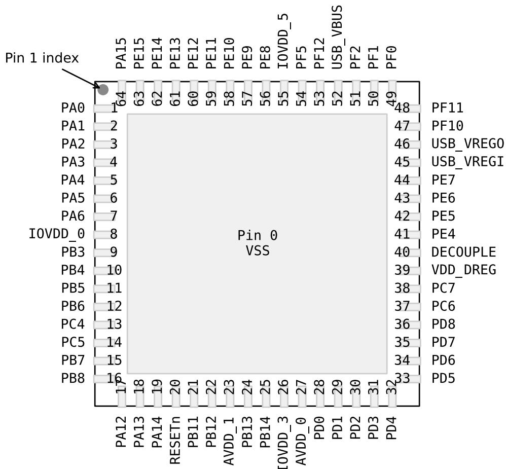
Figure 5.33. EFM32GG940 Pinout (top view, not to scale)
