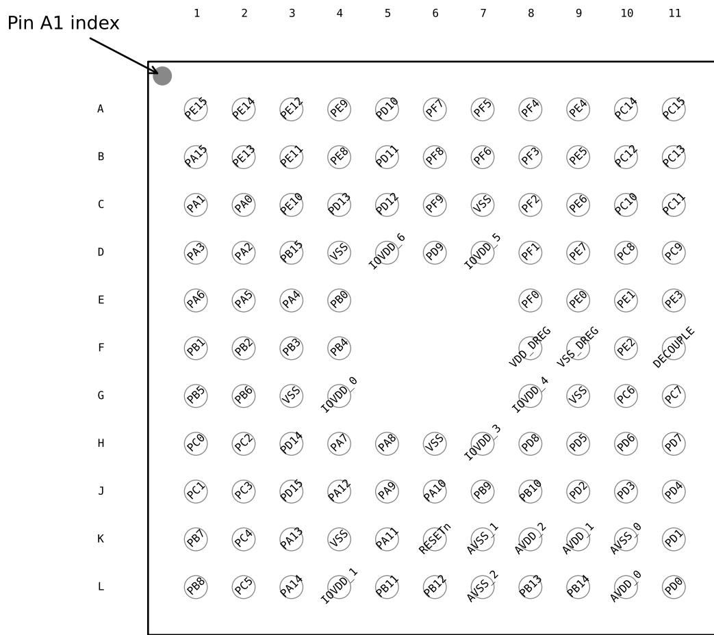
Figure 5.27. EFM32GG890 Pinout (top view, not to scale)
