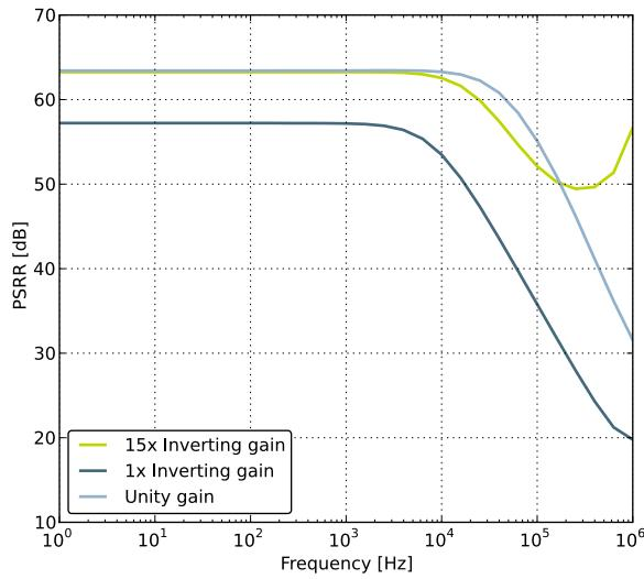
**Figure 4.33. OPAMP Negative Power Supply Rejection Ratio**
