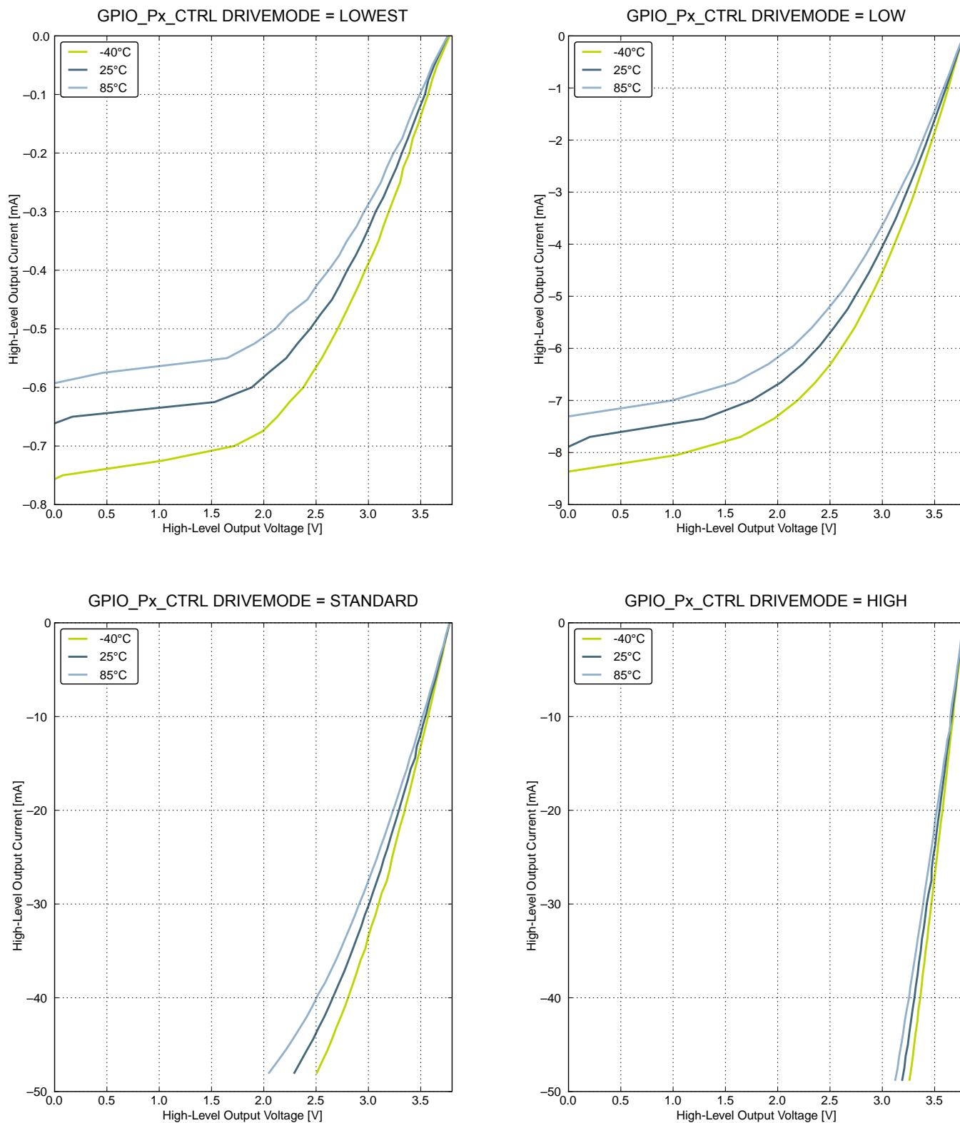
**Figure 4.15. Typical High-Level Output Current, 3.8 V Supply Voltage**
