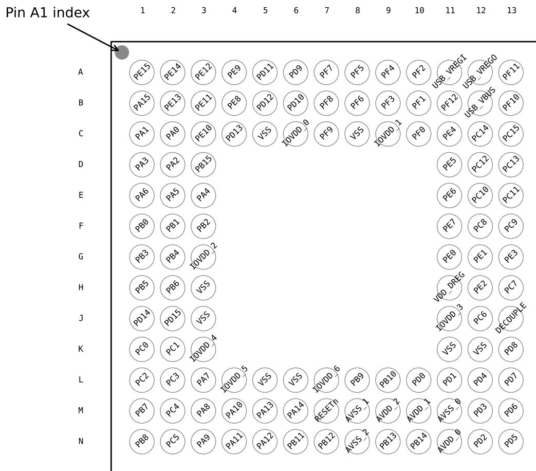
Figure 5.29. EFM32GG895 Pinout (top view, not to scale)
