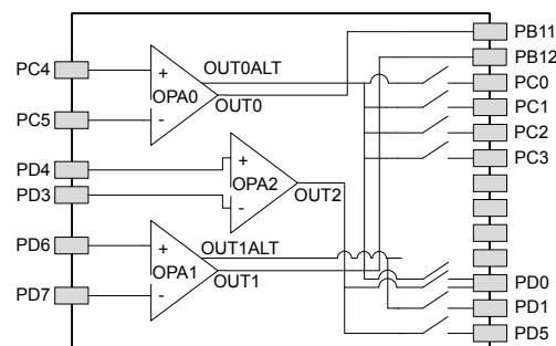
Figure 5.26. Opamp Pinout
