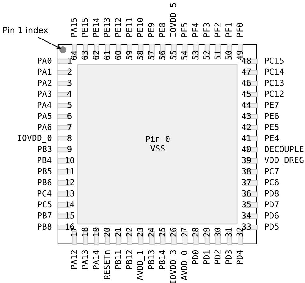
**Figure 5.21. EFM32GG840 Pinout (top view, not to scale)**
