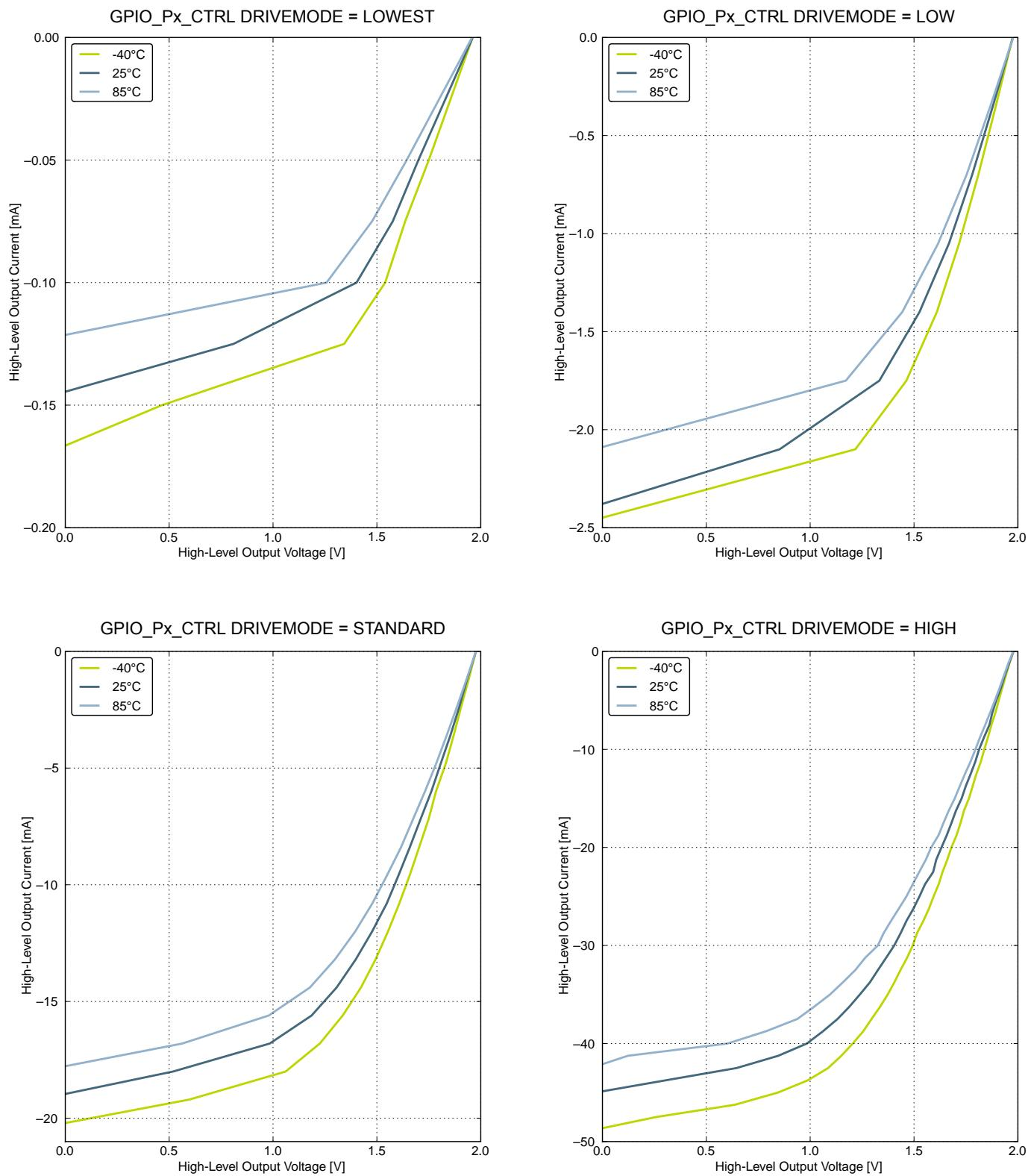
Figure 4.11. Typical High-Level Output Current, 2 V Supply Voltage
