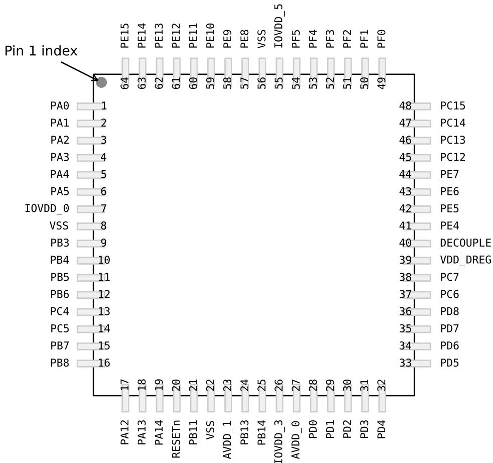
**Figure 5.23. EFM32GG842 Pinout (top view, not to scale)**
