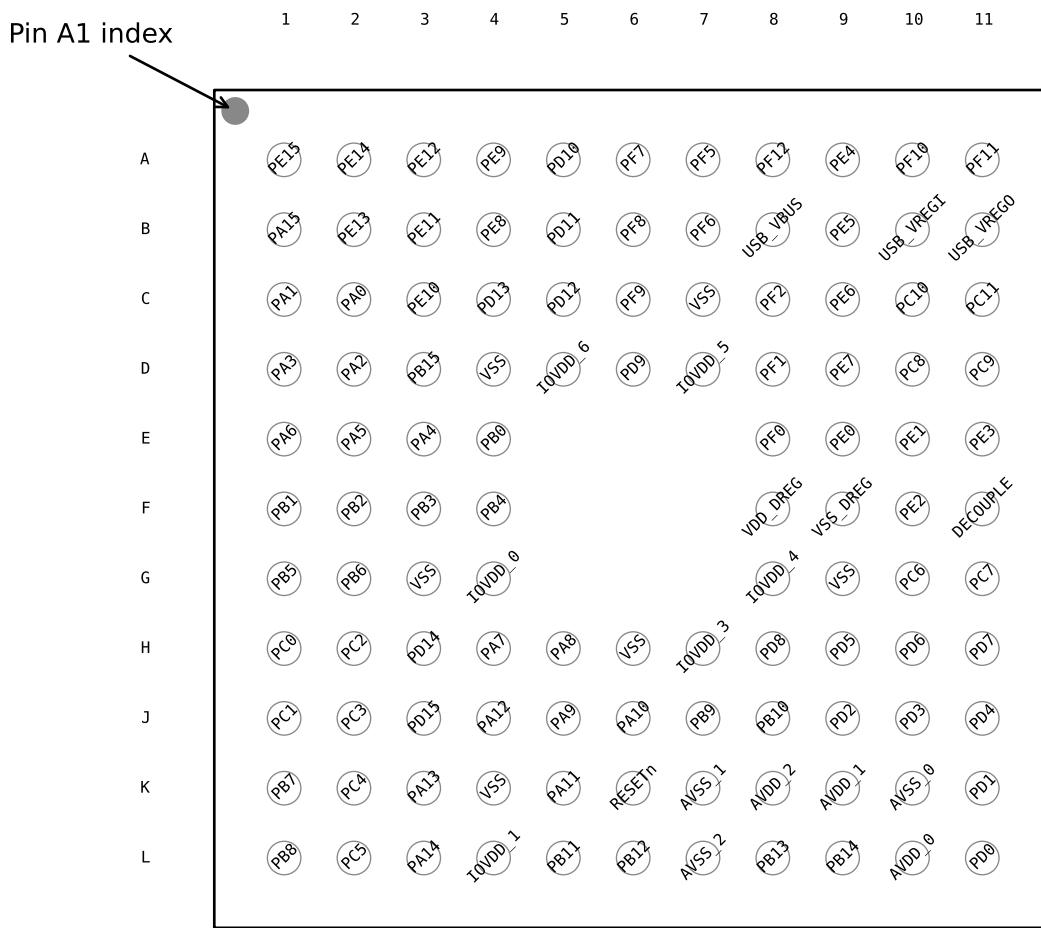
**Figure 5.17. EFM32GG390 Pinout (top view, not to scale)**
