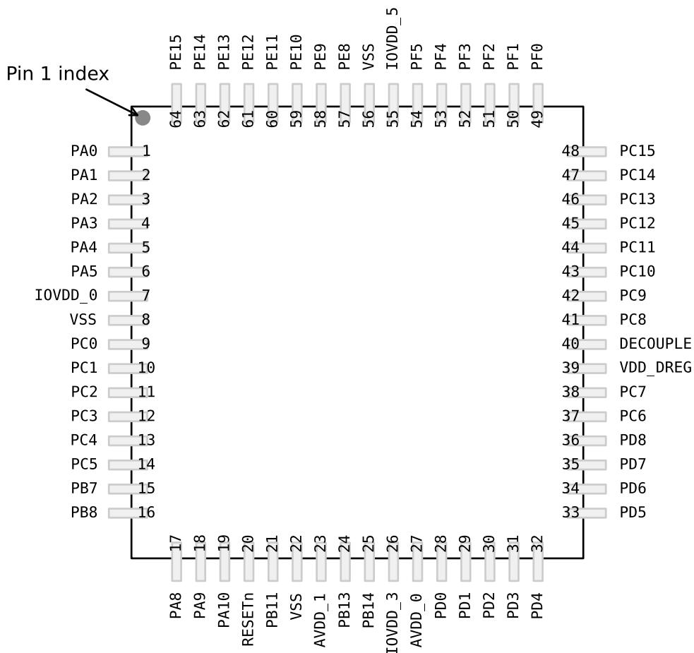
Figure 5.3. EFM32GG232 Pinout (top view, not to scale)
