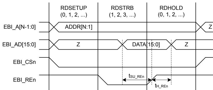
Figure 4.40. EBI Read Enable Related Timing Requirements
