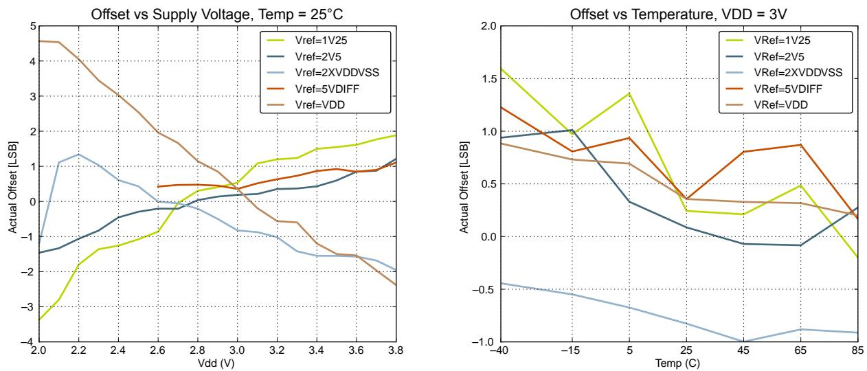
Figure 4.28. ADC Absolute Offset, Common Mode = VDD/2
