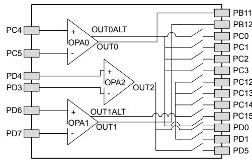
Figure 5.20. Opamp Pinout
