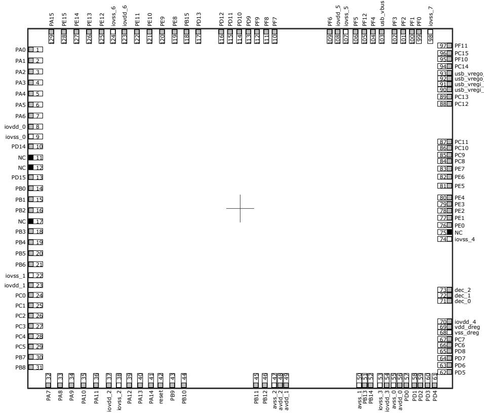
**Figure 5.31. EFM32GG900 Padout (top view, not to scale)**
