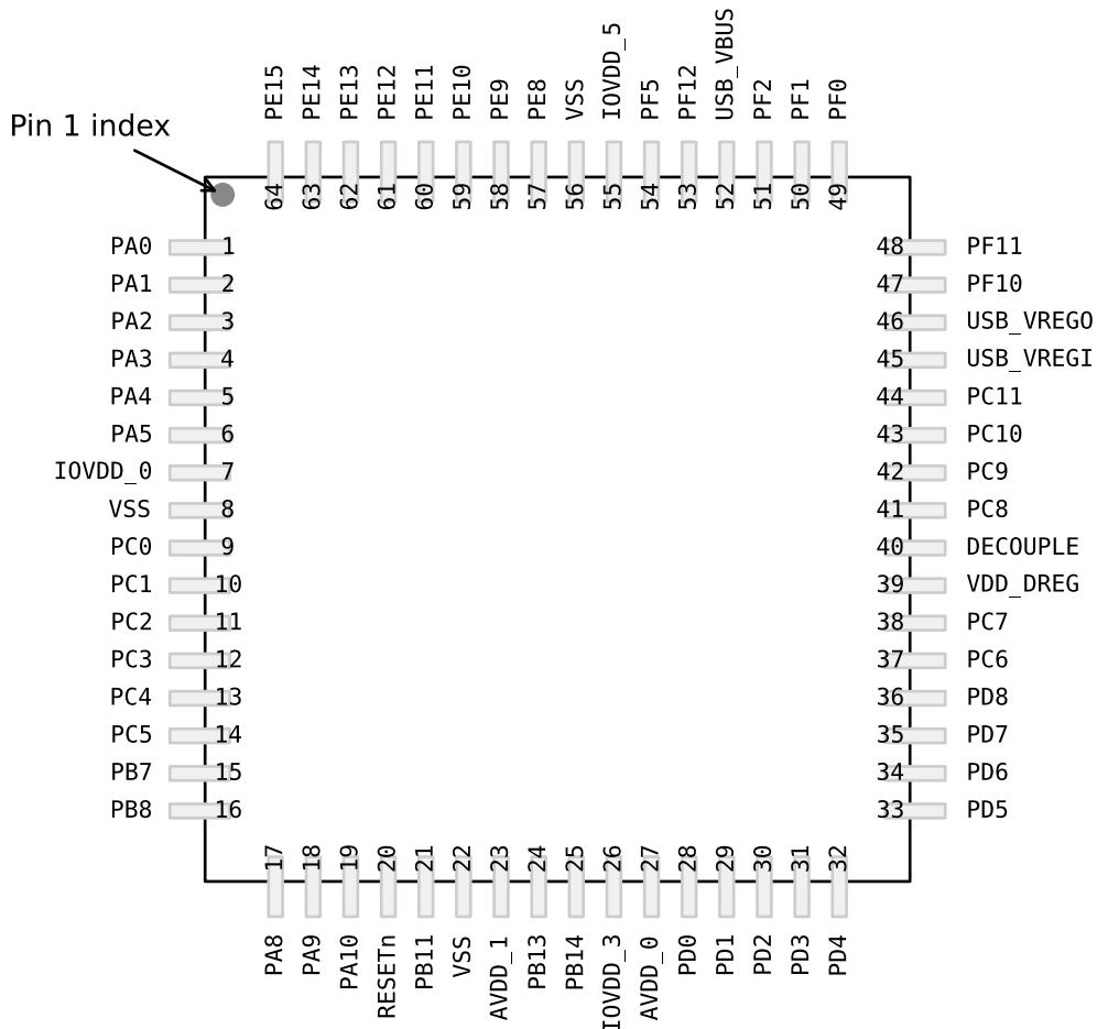
**Figure 5.13. EFM32GG332 Pinout (top view, not to scale)**
