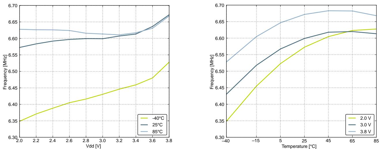
Figure 4.18. Calibrated HFRCO 7 MHz Band Frequency vs Supply Voltage and Temperature
