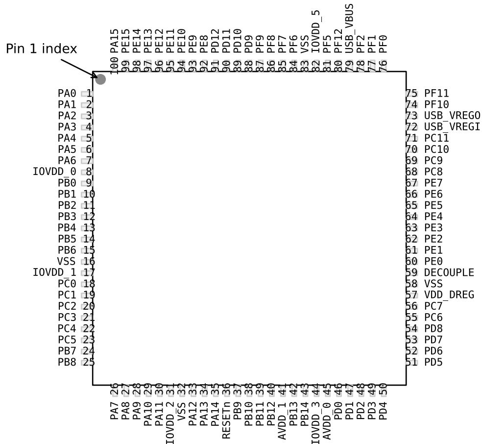
Figure 5.15. EFM32GG380 Pinout (top view, not to scale)
