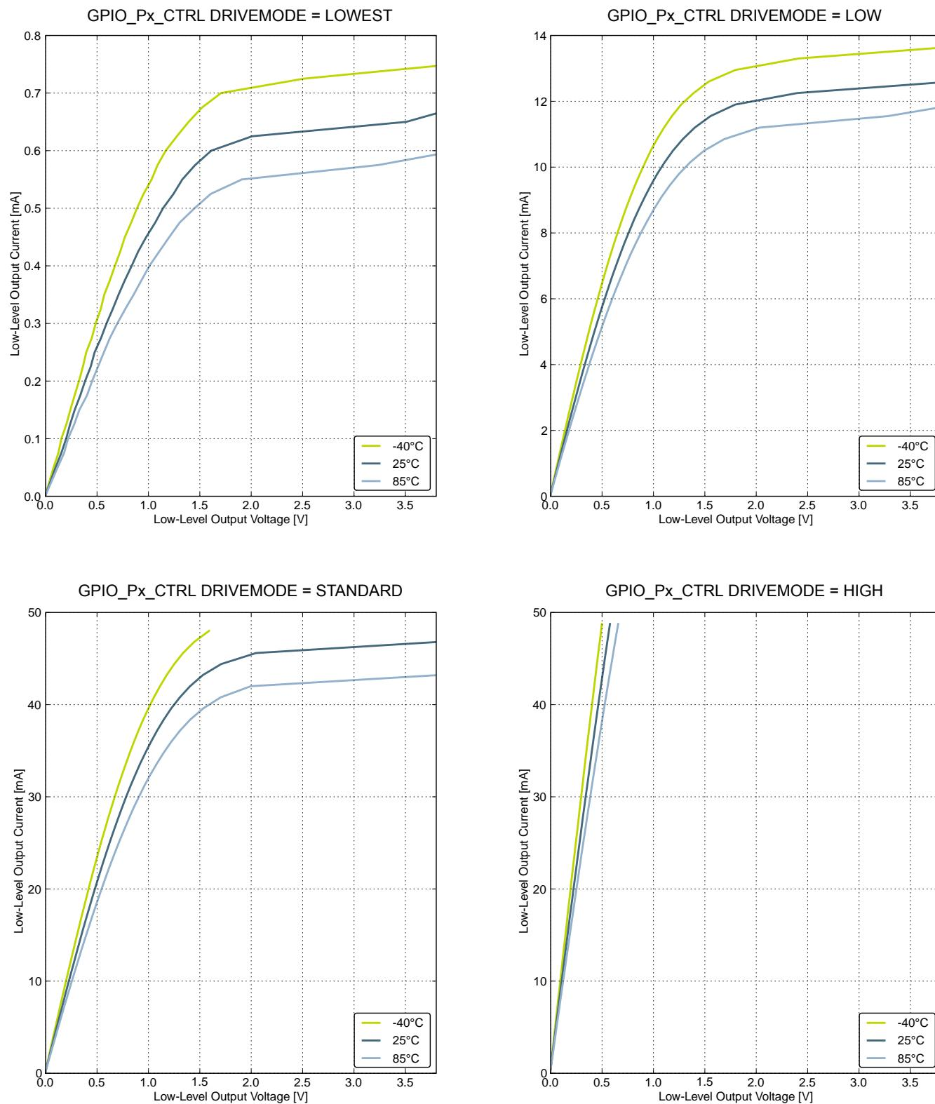
Figure 4.14. Typical Low-Level Output Current, 3.8 V Supply Voltage
