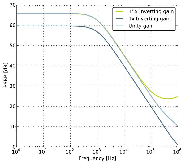
**Figure 4.32. OPAMP Positive Power Supply Rejection Ratio**
