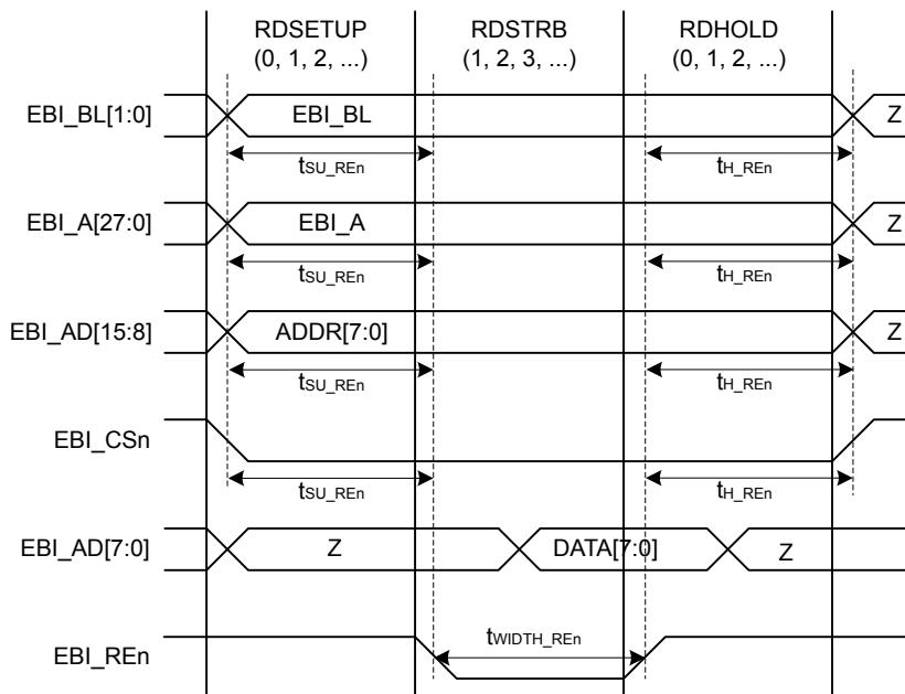
Figure 4.39. EBI Read Enable Related Output Timing
