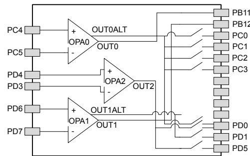
Figure 5.38. Opamp Pinout
