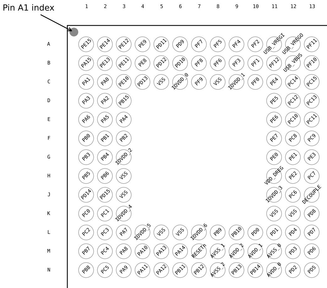
**Figure 5.9. EFM32GG295 Pinout (top view, not to scale)**
