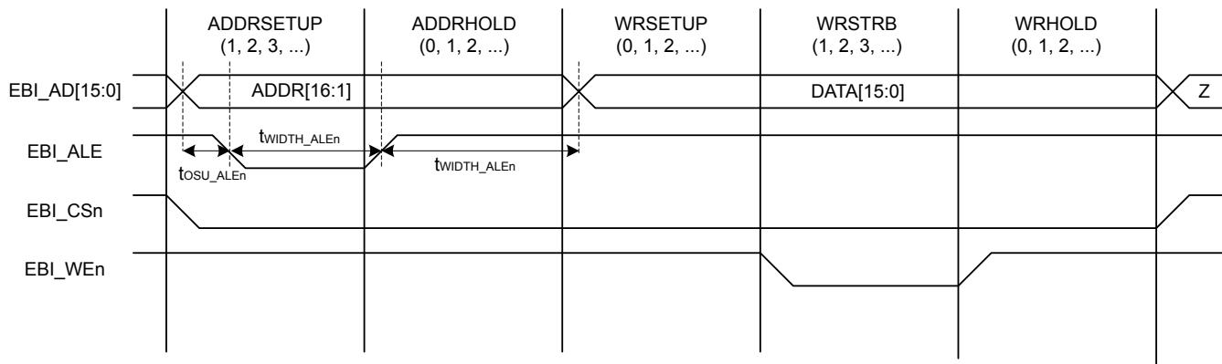
Figure 4.38. EBI Address Latch Enable Related Output Timing
