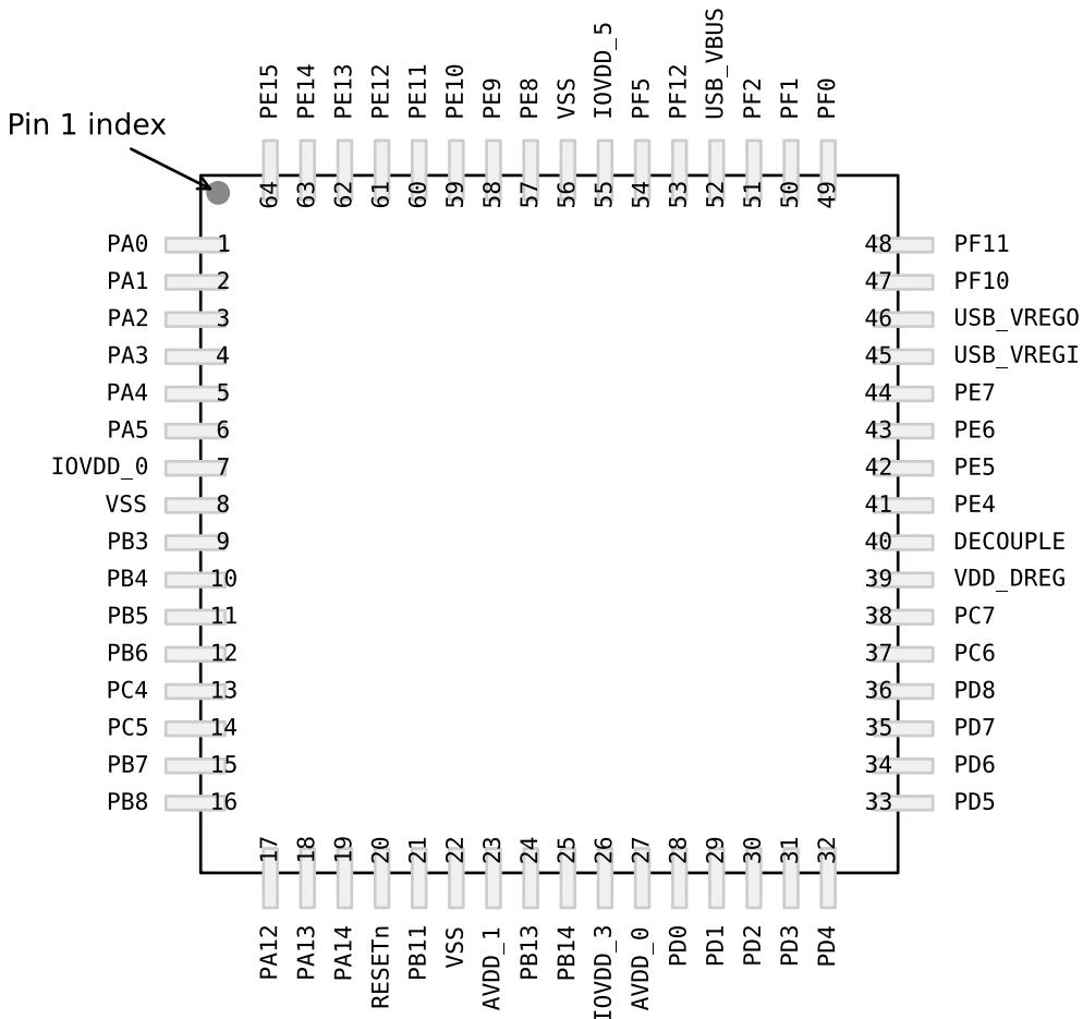
**Figure 5.35. EFM32GG942 Pinout (top view, not to scale)**
