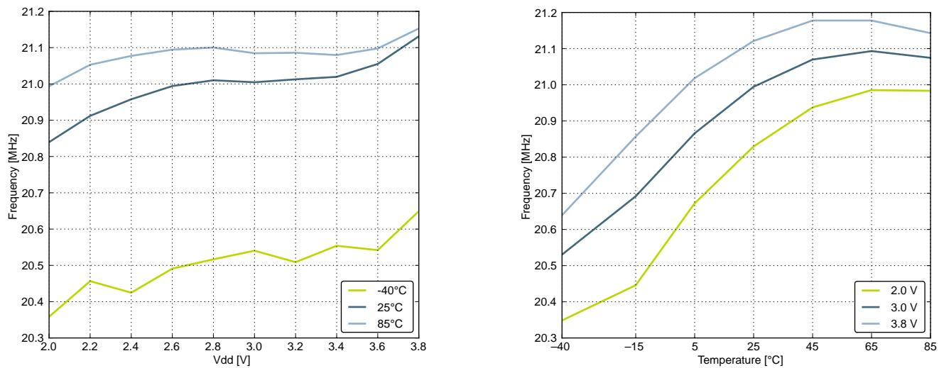
Figure 4.21. Calibrated HFRCO 21 MHz Band Frequency vs Supply Voltage and Temperature
