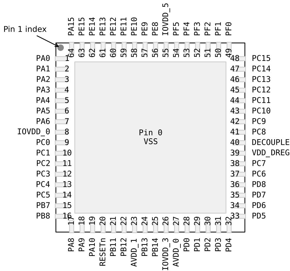
Figure 5.1. EFM32GG230 Pinout (top view, not to scale)
