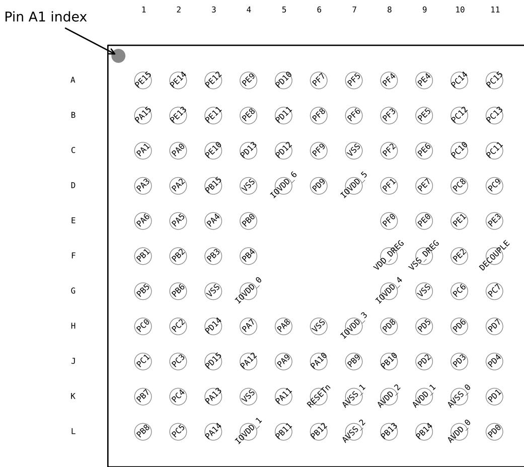
**Figure 5.7. EFM32GG290 Pinout (top view, not to scale)**
