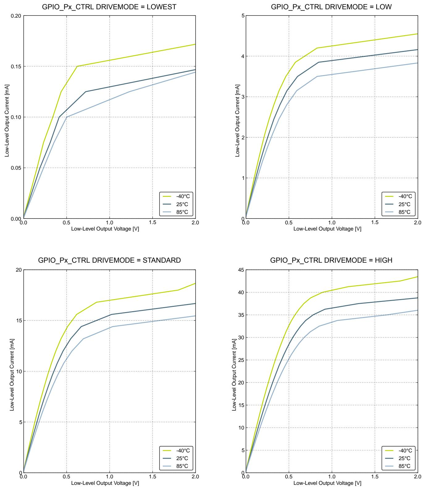
Figure 4.10. Typical Low-Level Output Current, 2V Supply Voltage
