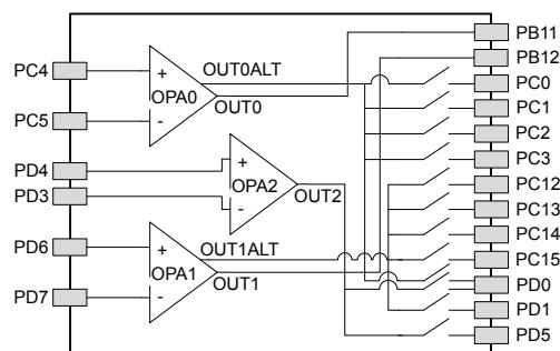
**Figure 5.2. Opamp Pinout**
