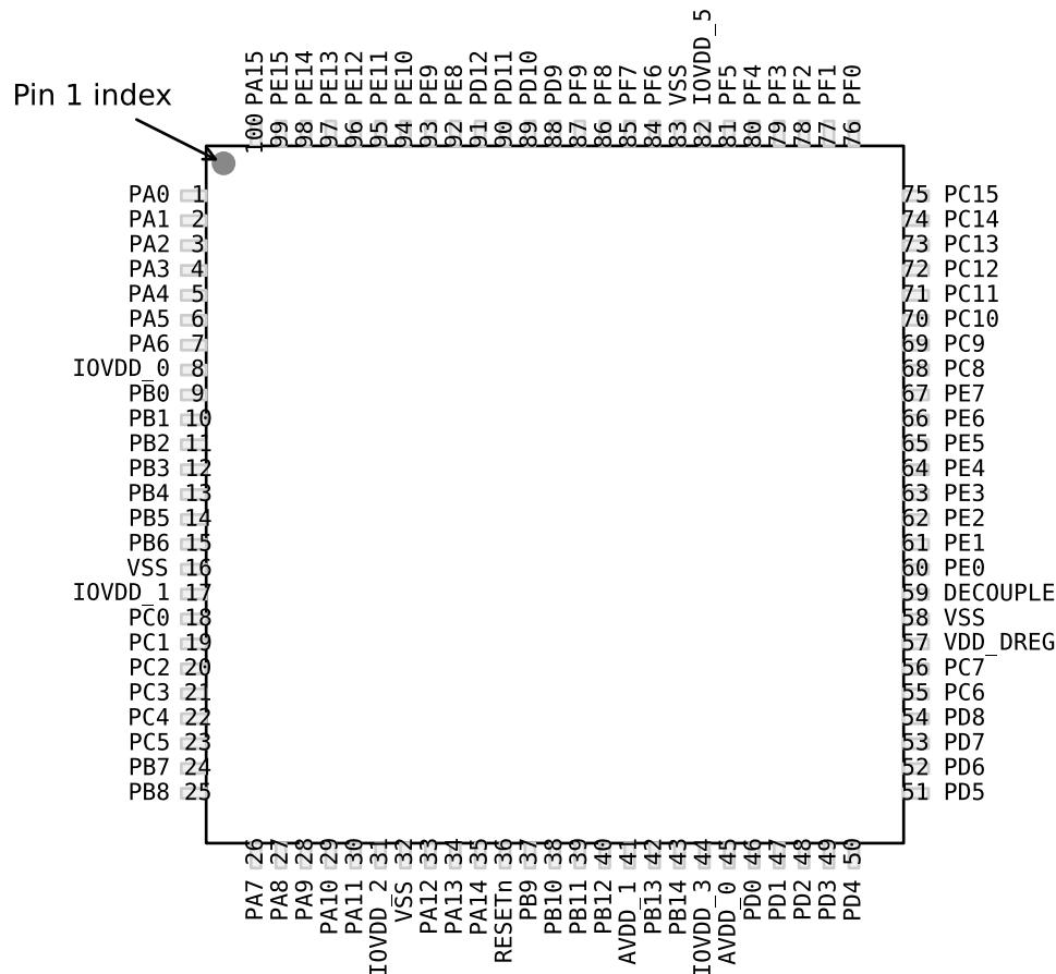
Figure 5.25. EFM32GG880 Pinout (top view, not to scale)
