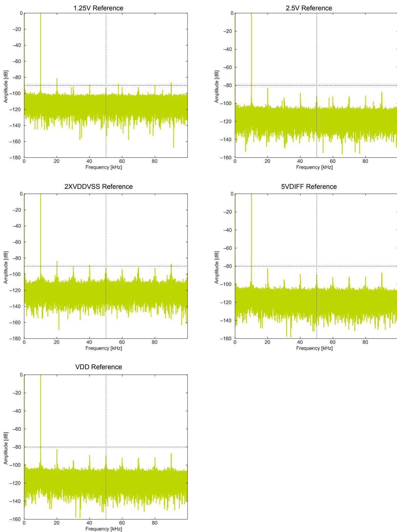
Figure 4.25. ADC Frequency Spectrum, VDD = 3 V, Temp = 25 °C
