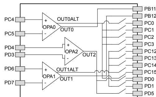
Figure 5.14. Opamp Pinout
