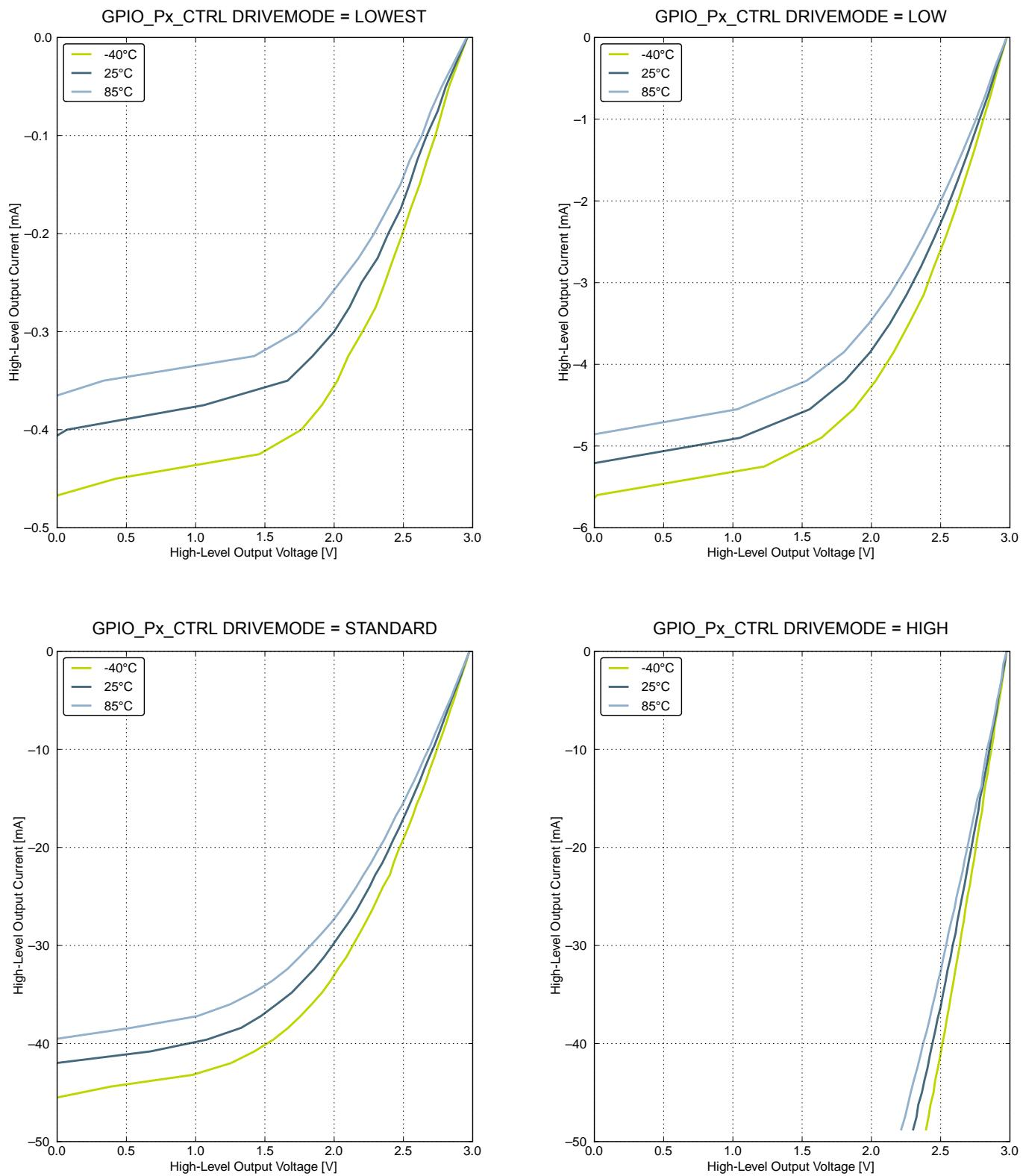
**Figure 4.13. Typical High-Level Output Current, 3 V Supply Voltage**
