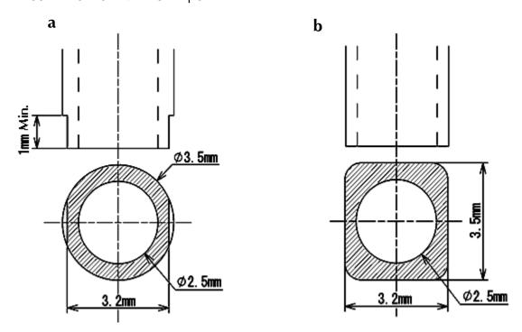
Nozzle with chamfering is recommended.
