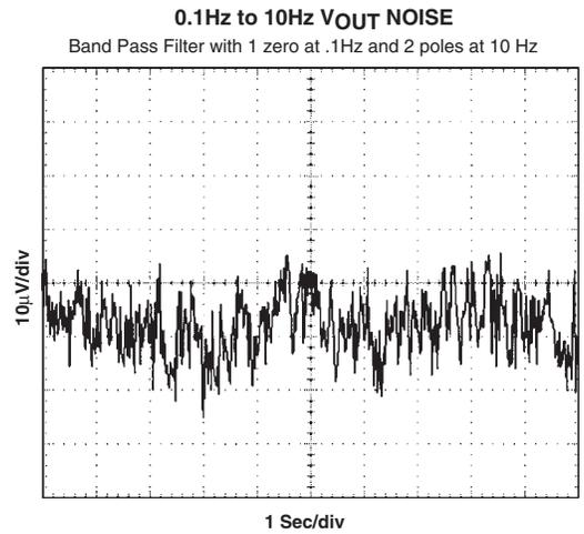
**Typical Performance Curves** ( $V_{IN} = 5.0V$ ,  $I_{OUT} = 0mA$ ,  $T_A = 25^\circ C$ , unless otherwise specified) (Continued)
