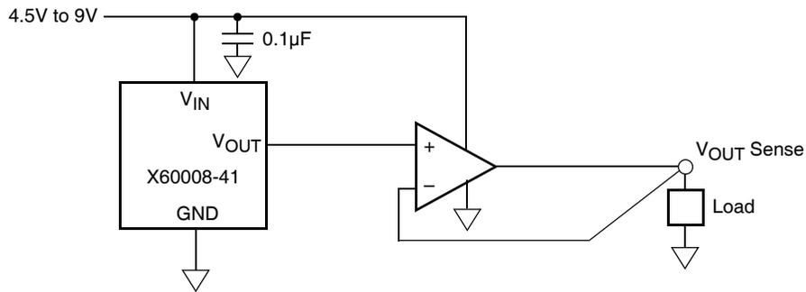
4.096V Full Scale Low-Drift 10-bit Adjustable Voltage Source
