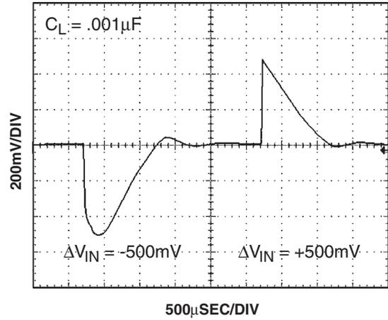
**Typical Performance Curves** ( $V_{IN} = 5.0V$ ,  $I_{OUT} = 0mA$ ,  $T_A = 25^\circ C$ , unless otherwise specified) (Continued)
