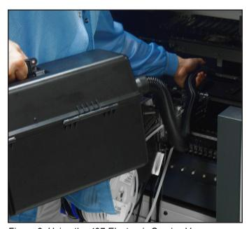
Figure 3. Using the 497 Electronic Service Vacuum
