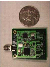
Figure 2. TD-SCDMA reference design board.
