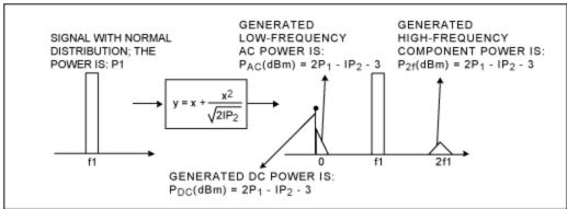
Figure 4. 2nd-order intermodulation products.
