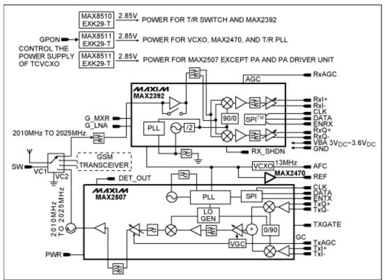
Figure 1. TD-SCDMA reference-design functional block diagram.
