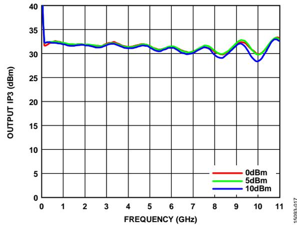
Figure 17. Output IP3 vs. Frequency for Various  $P_{OUT}/Tone$
