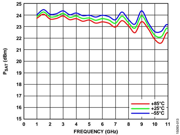
Figure 13.  $P_{SAT}$  vs. Frequency for Various Temperatures
