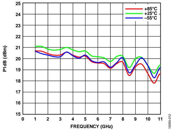
Figure 12. P1dB vs. Frequency for Various Temperatures
