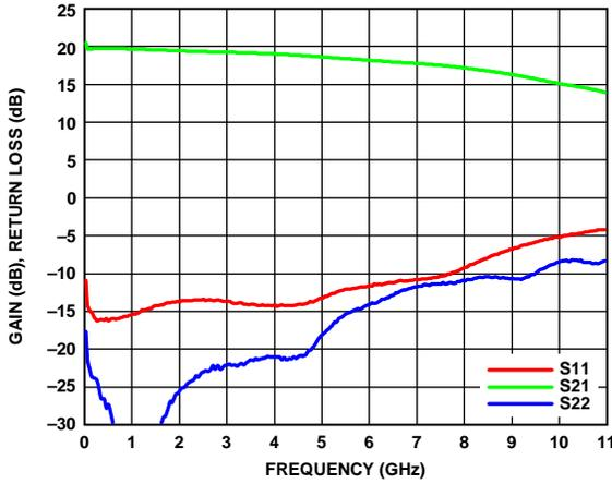
Figure 6. Gain and Return Loss vs. Frequency
