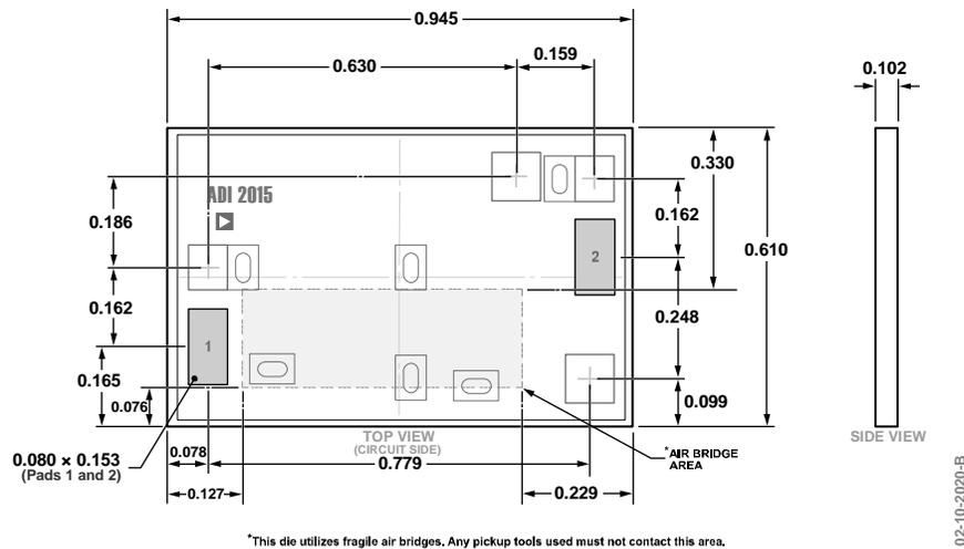
Figure 42. 2-Pad Bare Die [CHIP]
