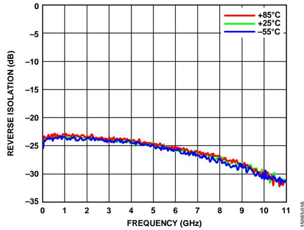
Figure 16. Reverse Isolation vs. Frequency for Various Temperatures
