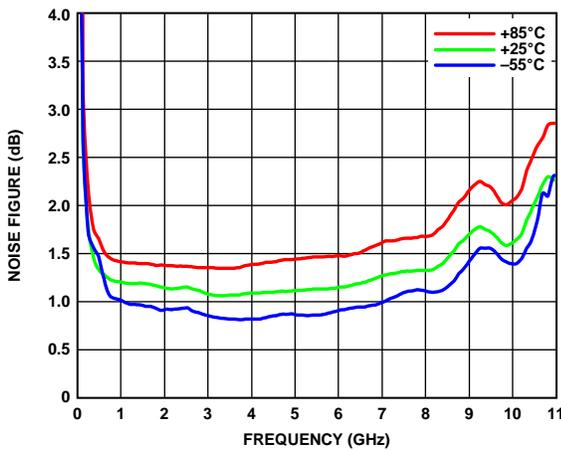
Figure 8. Noise Figure vs. Frequency for Various Temperatures
