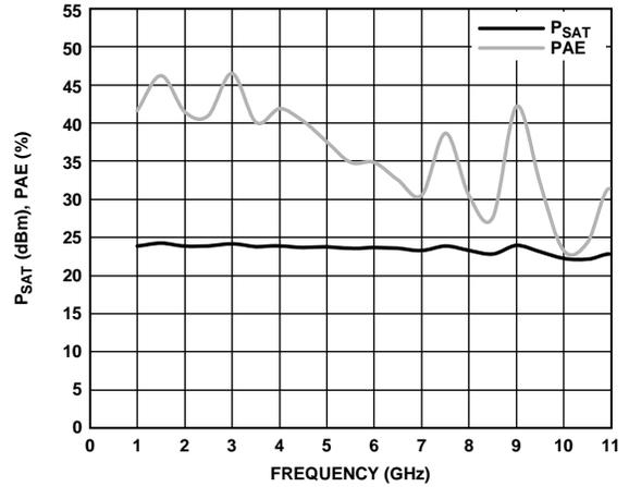
Figure 21.  $P_{SAT}$  and PAE vs. Frequency
