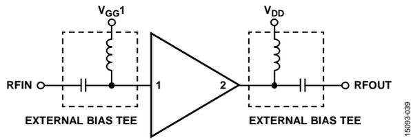
Figure 40. Application Circuit
