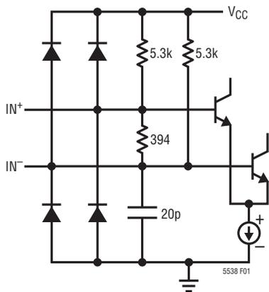
**Figure 1. Simplified Schematic of the Input Circuit**
