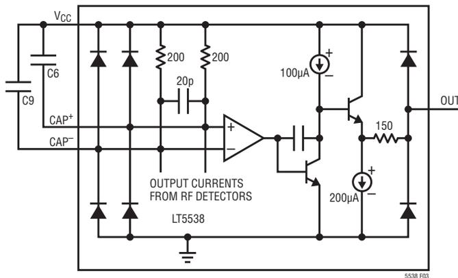
Figure 3. Simplified Schematic of the Output Interface
