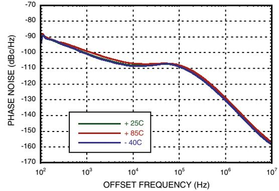
**SSB Phase Noise Fractional Spurs @ 9.61 GHz, Fref = 10 MHz, Loop BW = 10 kHz**
