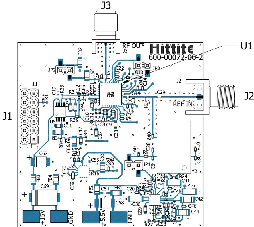
The circuit board used in the application should use RF circuit design techniques. Signal lines should have 50 Ohm impedance while the package ground leads and exposed paddle should be connected directly to the ground plane similar to that shown. A sufficient number of via holes should be used to connect the top and bottom ground planes. The evaluation circuit board shown is available from Hittite upon request.
