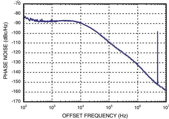
**SSB Phase Noise vs. Reference Freq. & Loop BW @ 9.6 GHz, Integer Mode**
