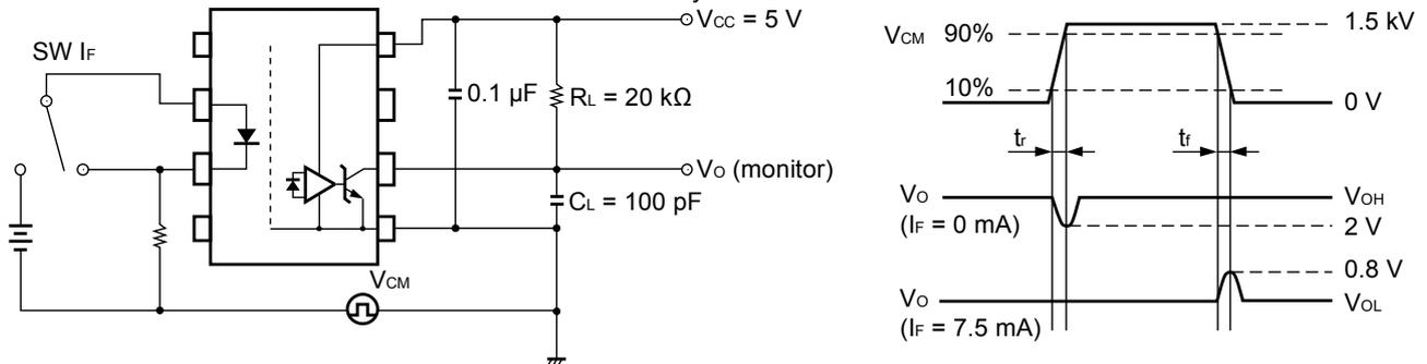
**Remark**  $C_L$  includes probe and stray wiring capacitance.
