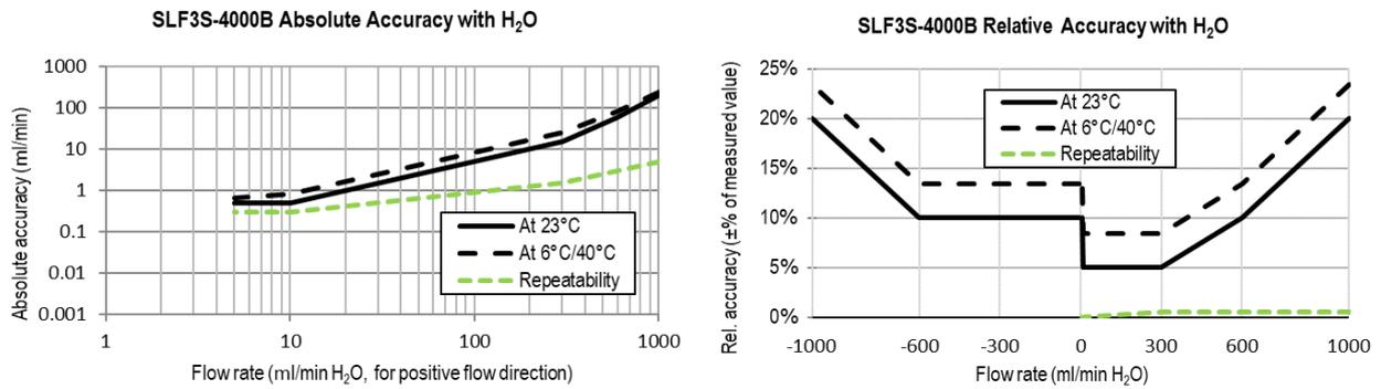
**Figure 1: Left:** Liquid flow sensor accuracy and repeatability across the flow range of the SLF3S-4000B. Relative error in ±% of measured value for H<sub>2</sub>O. **Right:** Liquid flow sensor accuracy and repeatability across the positive flow range of the SLF3S-4000B. Absolute error in ml/min for H<sub>2</sub>O.
