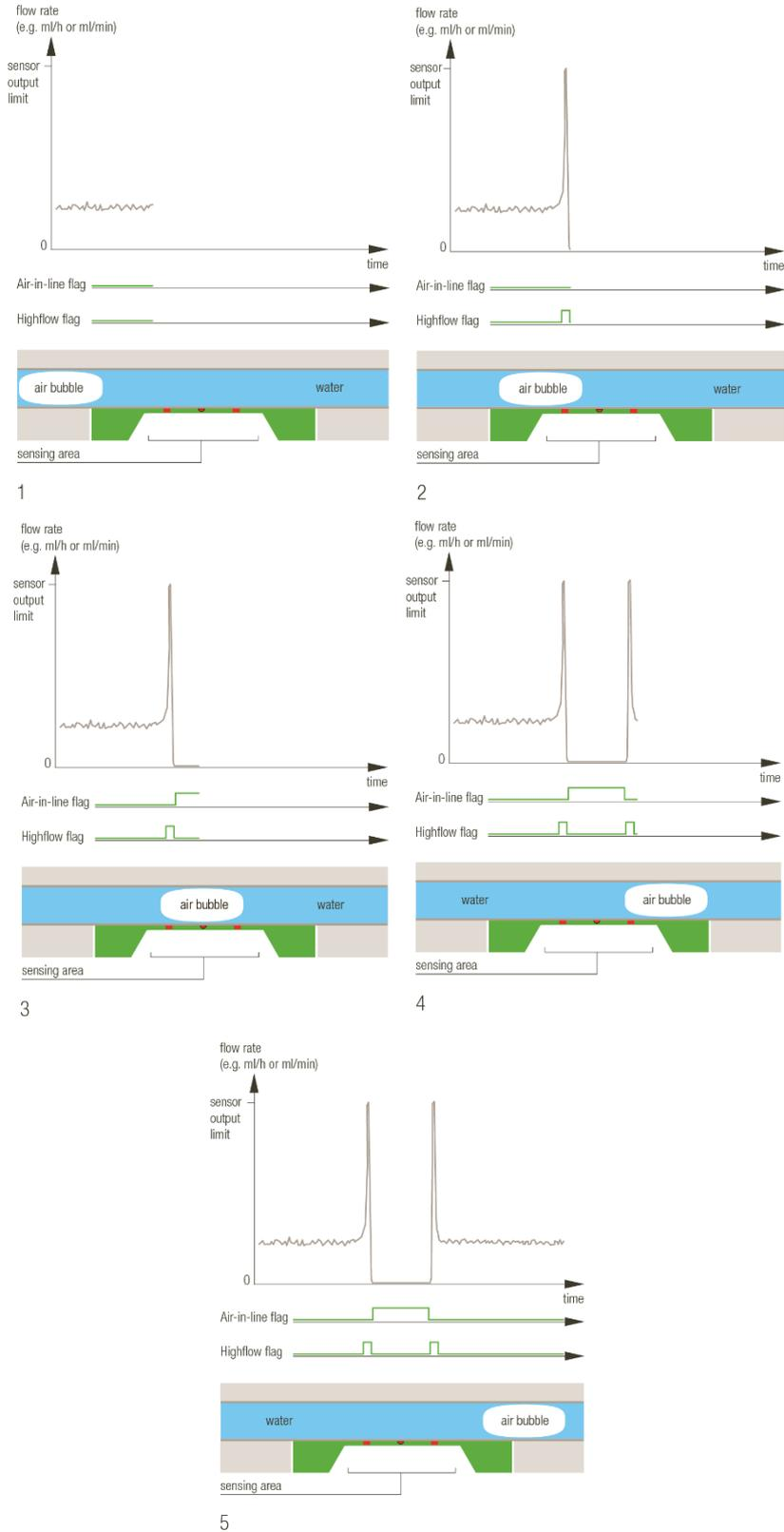
**Figure 3:** Detection of air-in-line events with the SLF3S-4000B. The graphs illustrate the air-in-line and high-flow flags while a bubble is passing through the sensor from left to right.
