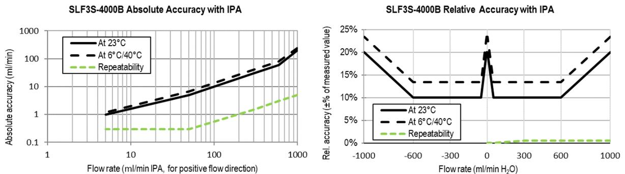
**Figure 2: Left:** Liquid flow sensor accuracy and repeatability across the flow range of the SLF3S-4000B. Relative error in ±% of measured value for IPA. **Right:** Liquid flow sensor accuracy and repeatability across the positive flow range of the SLF3S-4000B. Absolute error in ml/min for IPA.
