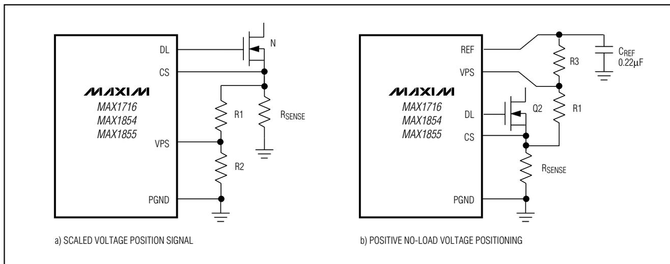
Figure 6. Voltage-Positioning Configurations
