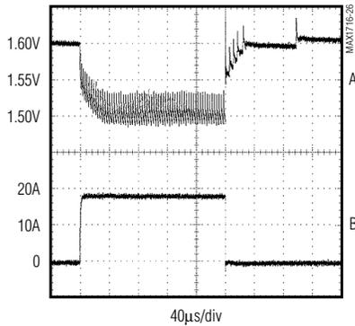
A.  $V_{OUT} = 1.6\text{V}$ , 50mV/div; B.  $I_{OUT} = 0.3\text{A TO } 18\text{A}$ , 10A/div
