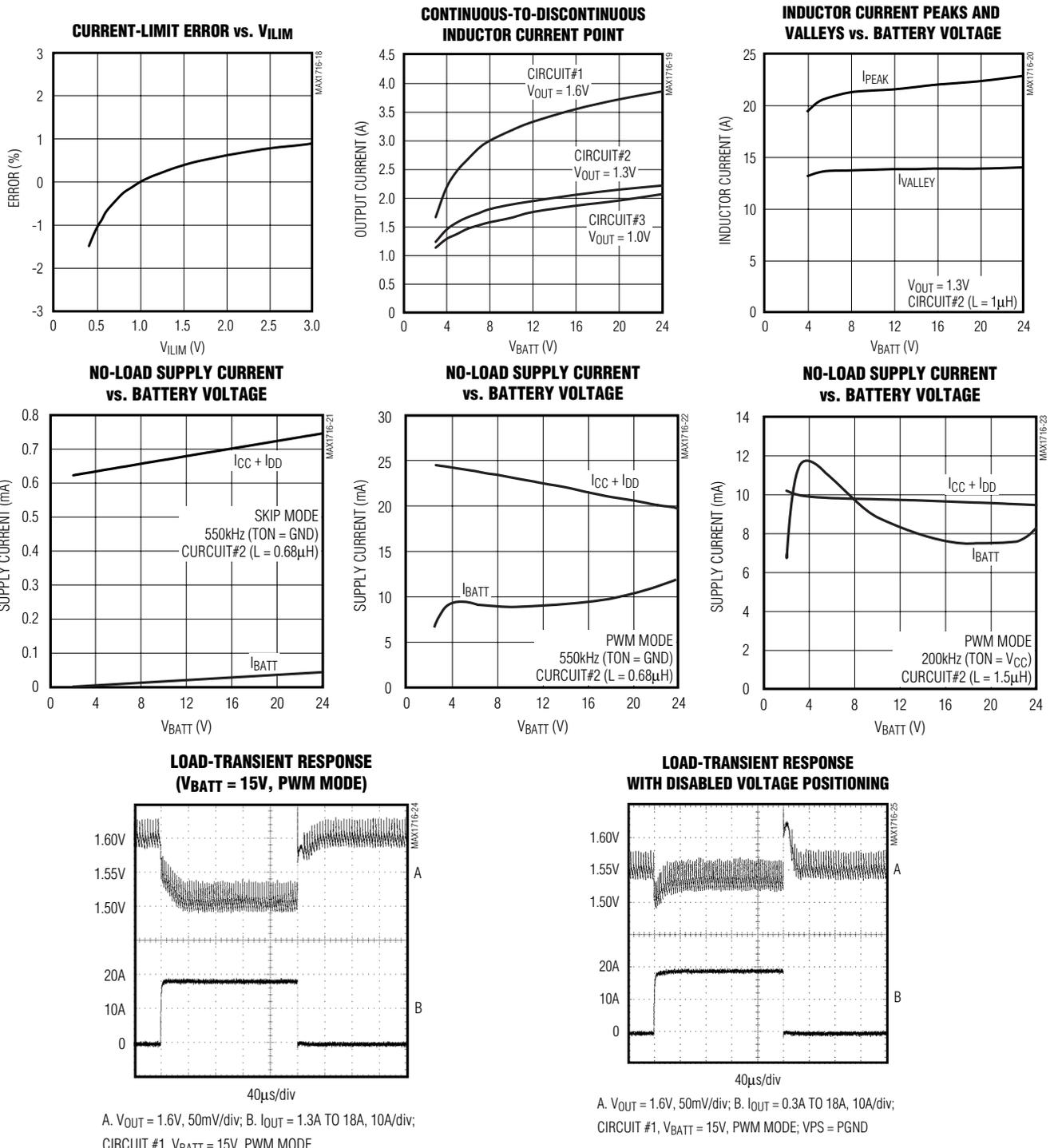
A.  $V_{OUT} = 1.6V$ , 50mV/div; B.  $I_{OUT} = 1.3A$  TO 18A, 10A/div; CIRCUIT #1,  $V_{BATT} = 15V$ , PWM MODE
