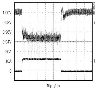
A.  $V_{OUT} = 1.0\text{V}$ , 20mV/div
