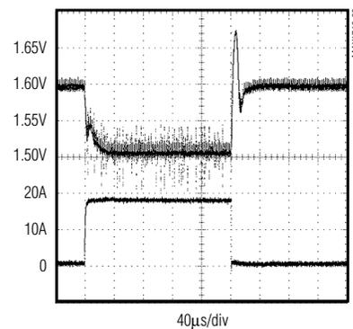
A.  $V_{OUT} = 1.6\text{V}$ , 50mV/div
