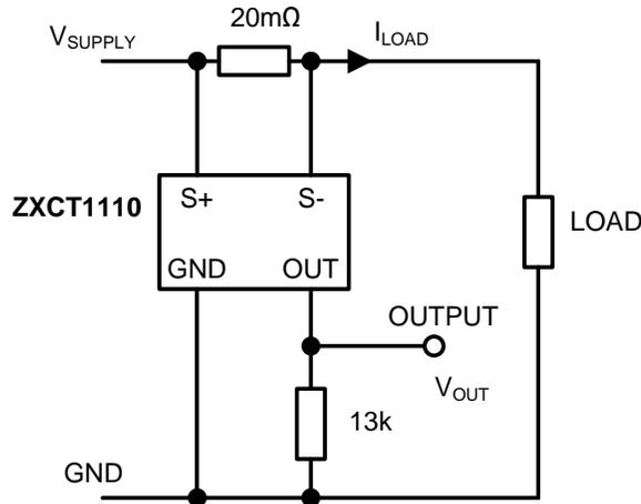
**Figure 3 Example Circuit using ZXCT1110**
