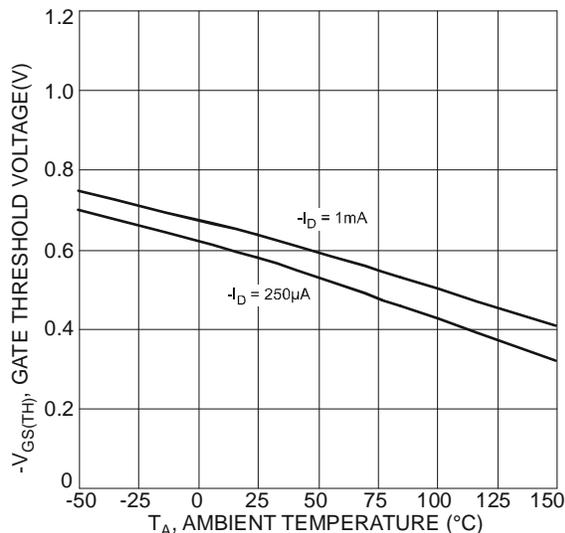
Fig. 5 Gate Threshold Variation vs. Ambient Temperature
