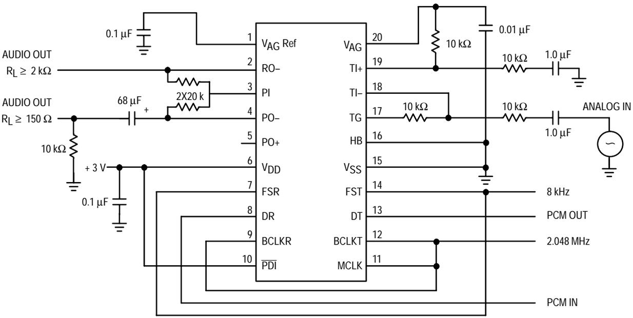
Figure 6. MC145483 Test Circuit — Signals Referenced to VSS
