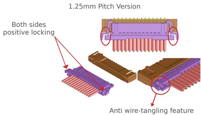
Both pitch versions offer similar locking features including side positive locks with anti wire-tangling feature and middle friction lock with window for visible mating assurance
