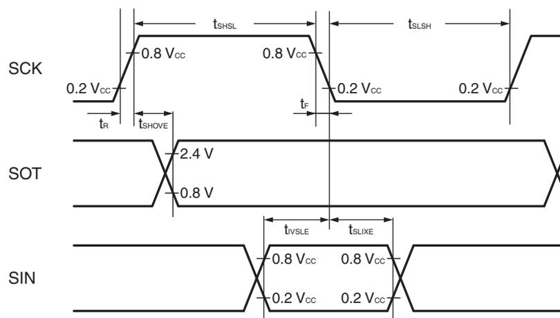
Sampling is executed at the rising edge of the sampling clock\*<sup>1</sup>, and serial clock delay is enabled\*<sup>2</sup>. (ESCR register : SCES bit = 0, ECCR register : SCDE bit = 1)
