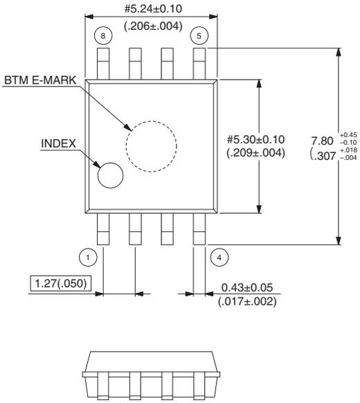
Note 1) Pins width and pins thickness include plating thickness.
