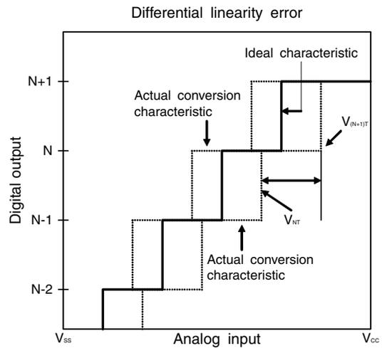
$$\text{Linearity error of digital output } N = \frac{V_{NT} - \{1 \text{ LSB} \times N + V_{OT}\}}{1 \text{ LSB}}$$
