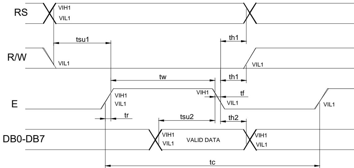
Read cycle ( $T_a=25^\circ\text{C}$ ,  $V_{DD}=5.0\text{V}$ )
